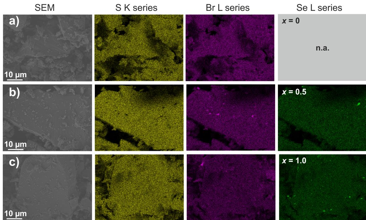
Figure S1: SEM and EDX analysis of  $\text{Li}_6\text{PS}_{5-x}\text{Se}_x\text{Br}$  showing the excellent elemental homogeneity.
