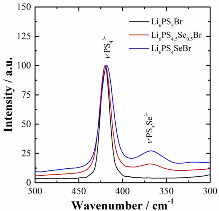
Figure S2: Raman spectra for  $\text{Li}_6\text{PS}_{5-x}\text{Se}_x\text{Br}$  ( $x = 0, 0.5$  and  $1.0$ ) showing the increase in the  $\text{PS}_3\text{Se}^{3-}$  vibrational mode with increasing Se content.
