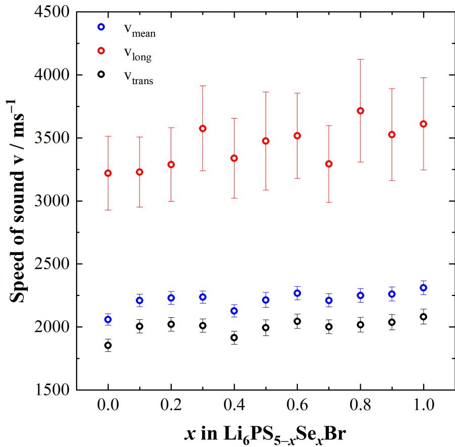
Figure S3: Measured longitudinal, transverse and mean speeds of sound for  $\text{Li}_6\text{PS}_{5-x}\text{Se}_x\text{Br}$ .
