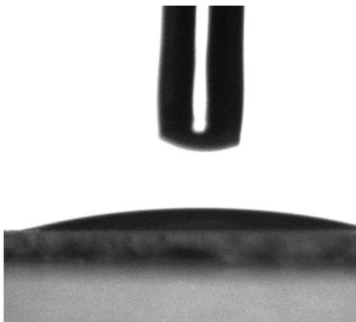
**Figure S4.** Contact angle measurement of hexadecane on compressed pellet of CPM-300. The oil droplet will wet the CPM-300 sample immediately upon contact, giving an initial transient contact angle of  $\sim 17.8^\circ$ , and complete wetting can be seen in less than 10 seconds.
