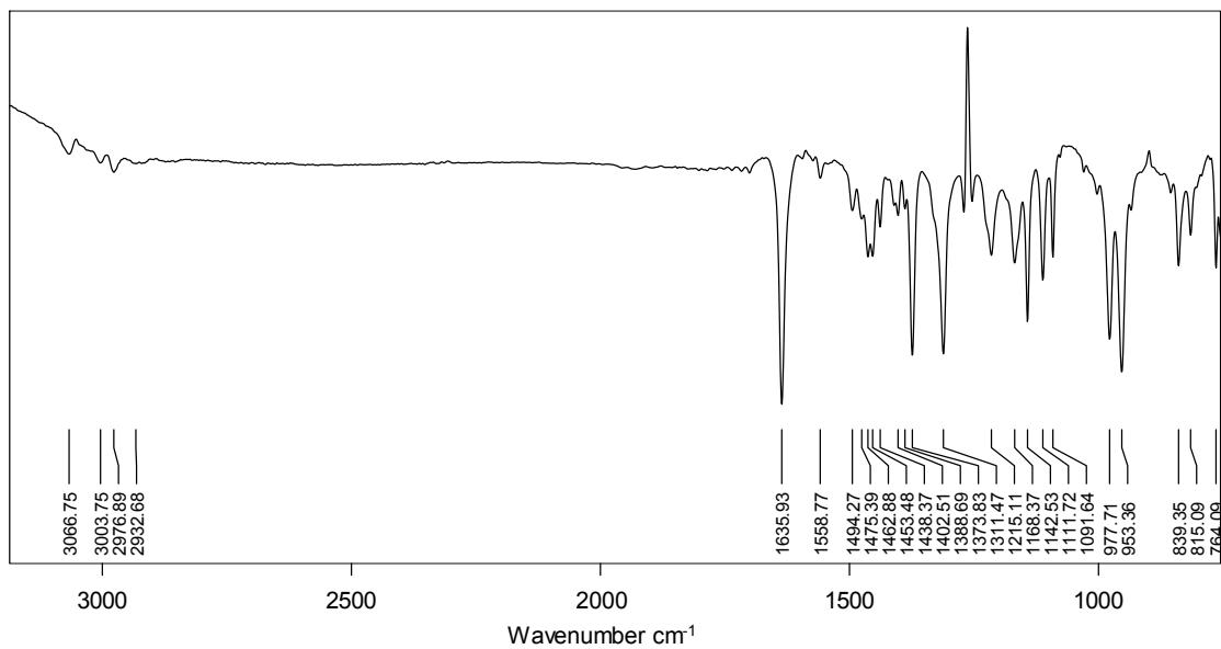
**Figure S8.** Solution ATR infrared spectra of the filtered reaction  $\{\text{Bo}^{\text{M}}\text{Flu}\}\text{Rh}(\eta^4\text{-C}_{16}\text{H}_{12}) + 1 \text{ eq. AgSbF}_6$  as a 0.1 M solution in  $\text{CH}_2\text{Cl}_2$ .
