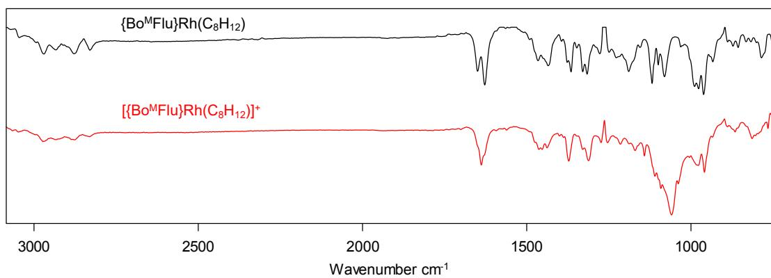
**Figure S6.** Solution ATR infrared spectra of  $\{\text{Bo}^{\text{M}}\text{Flu}\}\text{Rh}(\eta^4\text{-C}_8\text{H}_{12})$  (Black) and  $[\{\text{Bo}^{\text{M}}\text{Flu}\}\text{Rh}(\text{C}_8\text{H}_{12})]^+ \text{[BF}_4^-$  (Red) as 0.1 M solutions in  $\text{CH}_2\text{Cl}_2$ .
