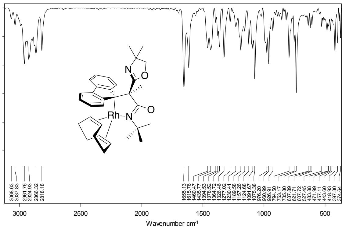
**Figure S40.** Infrared spectrum (KBr) of  $\{\text{Bo}^{\text{M}}\text{Flu}\}\text{Rh}(\eta^4\text{-C}_8\text{H}_{12})$ .
