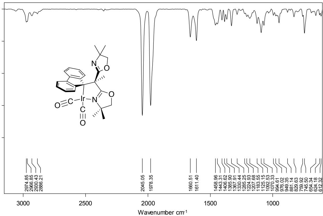
**Figure S49.** Infrared spectrum (KBr) of  $\{\text{Bo}^{\text{M}}\text{Flu}\}\text{Ir}(\text{CO})_2$ .
