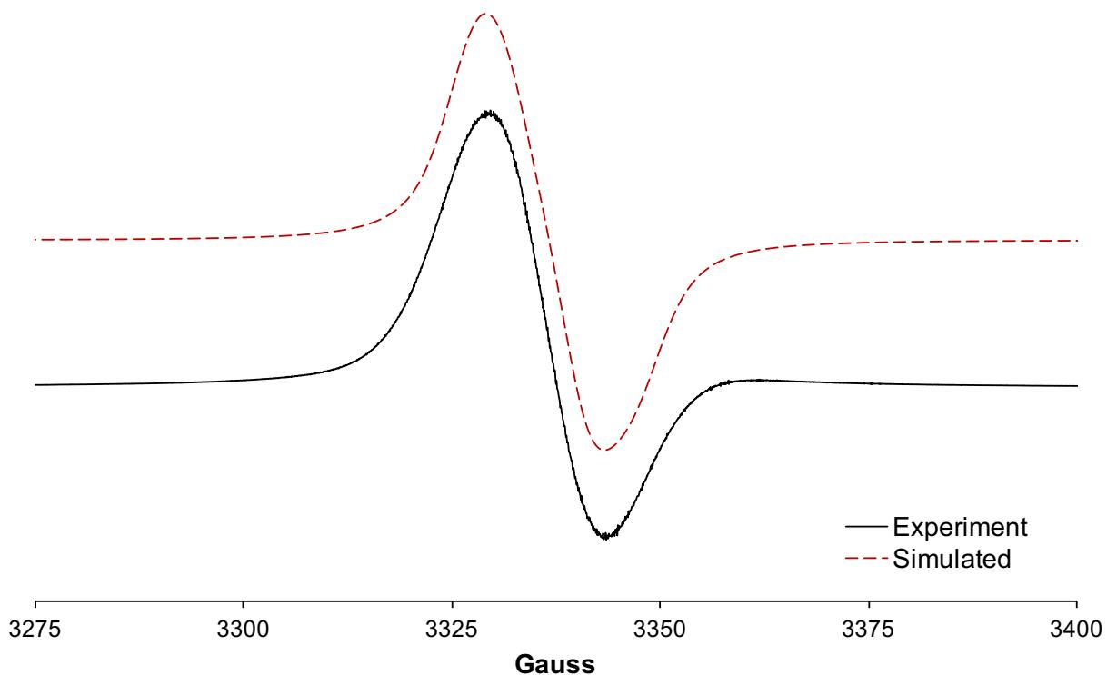
**Figure S13.** CW X-band EPR spectra of  $\{\text{Bo}^{\text{M}}\text{Flu}\}\text{Rh}(\eta^4\text{-C}_8\text{H}_{12})\text{][BF}_4$  in 2-methyltetrahydrofuran with 0.1 M  $[\text{nBu}_4\text{N}]\text{PF}_6$  at 20 K.  $g_x = 2.012$  ( $A_{\text{Rh}} = 15.5$  G)  $g_y = 2.004$  ( $A_{\text{Rh}} = 16.5$  G)  $g_z = 2.009$  ( $A_{\text{Rh}} = 19.2$  G).
