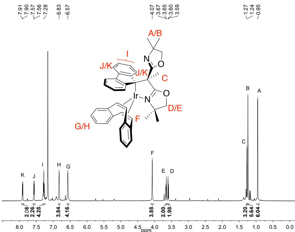
**Figure S59.**  $^1\text{H}$  NMR spectrum of  $\{\text{Bo}^{\text{M}}\text{Flu}\}\text{Ir}(\eta^4\text{-C}_{16}\text{H}_{12})$  acquired in benzene- $d_6$ .
