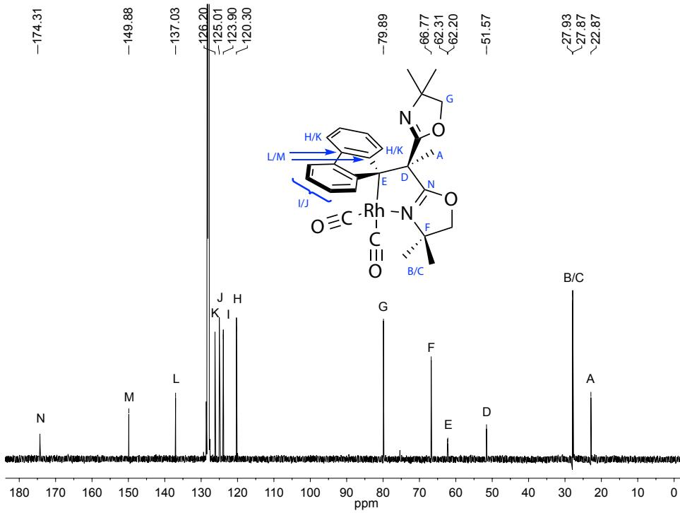
**Figure S45.**  $^{13}\text{C}\{^1\text{H}\}$  NMR spectrum of  $\{\text{Bo}^{\text{M}}\text{Flu}\}\text{Rh}(\text{CO})_2$  acquired in benzene- $d_6$ .
