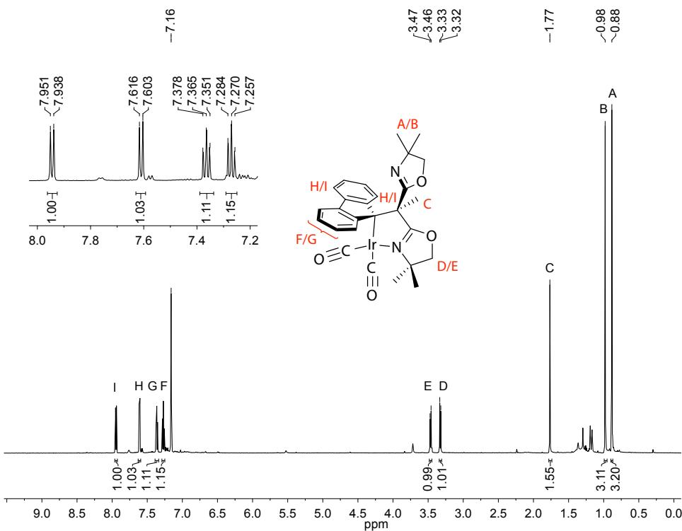
**Figure S47.**  ${}^1\text{H}$  NMR spectrum of  $\{\text{Bo}^{\text{M}}\text{Flu}\}\text{Ir}(\text{CO})_2$  acquired in benzene- $d_6$ .
