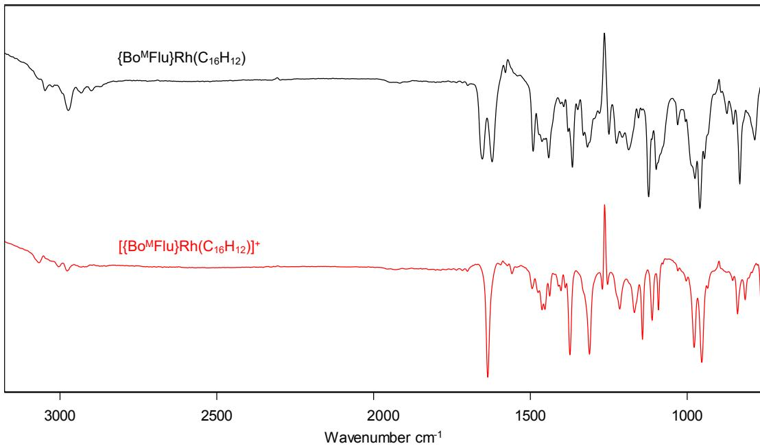
**Figure S9.** Solution ATR of  $\{\text{Bo}^{\text{M}}\text{Flu}\}\text{Rh}(\eta^4\text{-C}_{16}\text{H}_{12})$  (Black) and  $[\{\text{Bo}^{\text{M}}\text{Flu}\}\text{Rh}(\text{C}_{16}\text{H}_{12})][\text{SbF}_6]$  (Red) as 0.1 M solutions in  $\text{CH}_2\text{Cl}_2$ .
