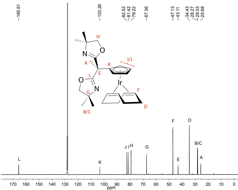
**Figure S29.**  $^{13}\text{C}\{\text{H}\}$  NMR spectrum of  $\{\text{Bo}^{\text{M}}\text{Cp}\}\text{Ir}(\eta^4\text{-C}_8\text{H}_{12})$  acquired at room temperature in benzene- $d_6$ .
