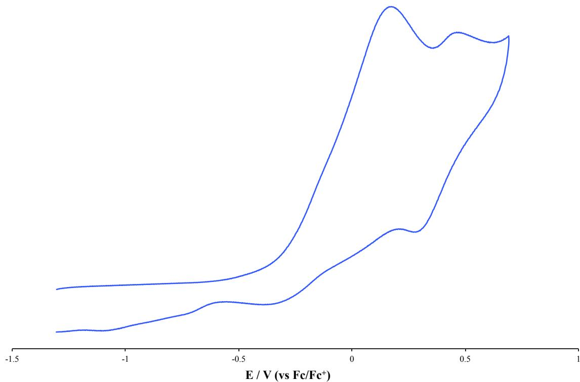
**Figure S3.** Cyclic voltammogram of  $\{\text{Bo}^{\text{M}}\text{Flu}\}\text{Rh}(\text{CO})_2$ . Conditions: 1 mM in methylene chloride, 0.1 M  $[(\text{nBu})_4\text{N}][\text{BF}_4]$ ,  $0.1 \text{ V}\cdot\text{s}^{-1}$ .  $E$  values are given in V versus  $\text{Cp}_2\text{Fe}/\text{Cp}_2\text{Fe}^+$ .
