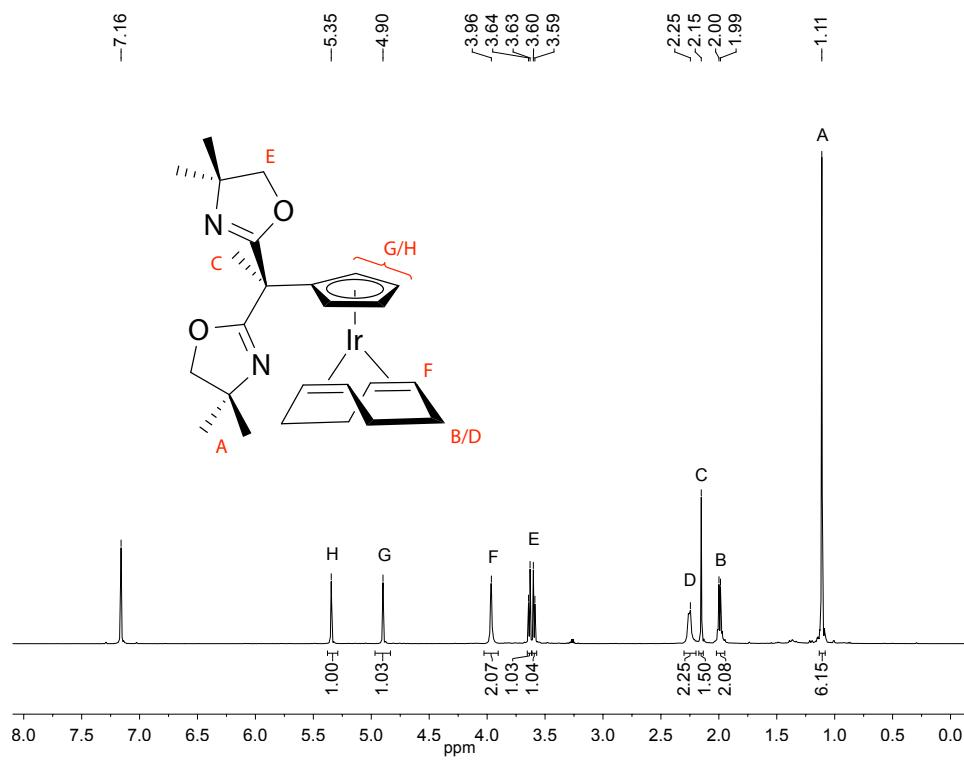
**Figure S28.**  ${}^1\text{H}$  NMR spectrum of  $\{\text{Bo}^{\text{M}}\text{Cp}\}\text{Ir}(\eta^4\text{-C}_8\text{H}_{12})$  acquired at room temperature in benzene- $d_6$ .
