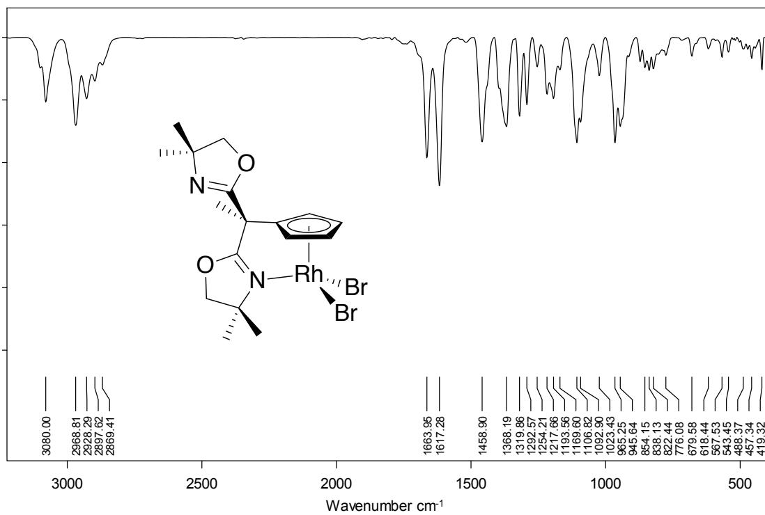
**Figure S34.** Infrared spectrum (KBr) of  $\{\text{Bo}^M \text{Cp}\} \text{RhBr}_2$ .
