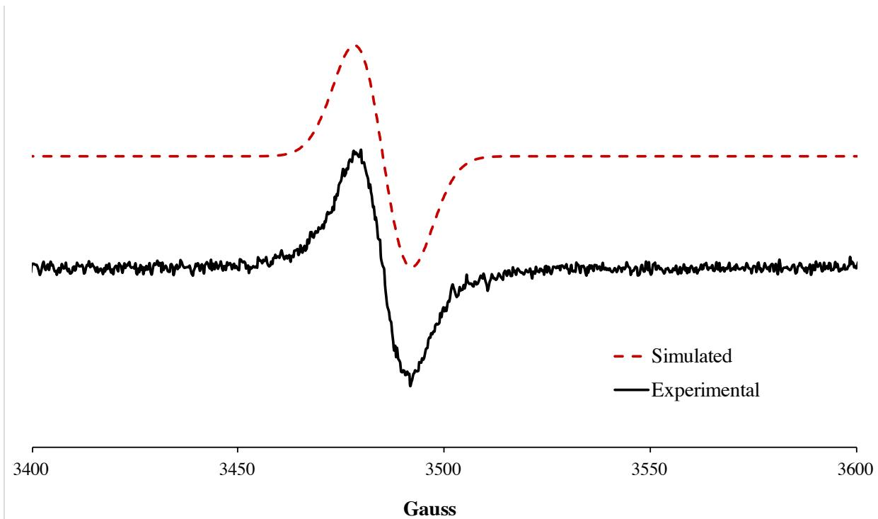
**Figure S18.** CW X-band EPR spectra of  $\{ \text{Bo}^{\text{M}}\text{Flu} \} \text{Ir}(\eta^4\text{-C}_{16}\text{H}_{12}) \text{[BF}_4]$  at a 10 mM solution in  $\text{CH}_2\text{Cl}_2$  at 298 K. The spectrum is simulated using isotropic parameters  $g = 2.018$  ( $A_{\text{Ir}} = 2.3$  G).
