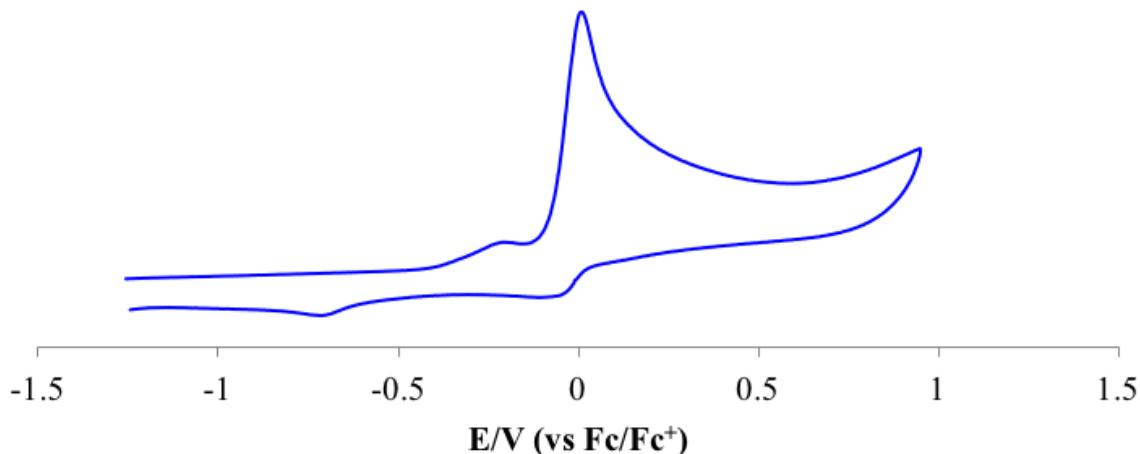
**Figure S1.** Cyclic voltammogram of {Bo<sup>M</sup>Cp}Rh( $\eta^4$ -C<sub>8</sub>H<sub>12</sub>). Conditions: 1 mM in CH<sub>3</sub>CN, 0.1 M [(nBu)<sub>4</sub>N][BF<sub>4</sub>], 0.5 V·s<sup>-1</sup>. *E* values are given in V vs Cp<sub>2</sub>Fe/Cp<sub>2</sub>Fe<sup>+</sup>.
