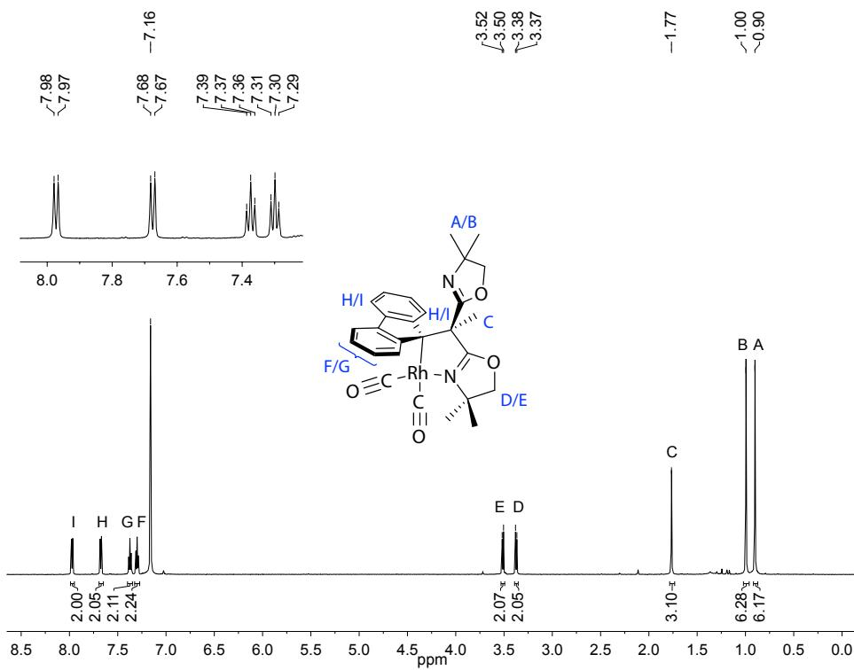
**Figure S44.**  $^1\text{H}$  NMR spectrum of  $\{\text{Bo}^{\text{M}}\text{Flu}\}\text{Rh}(\text{CO})_2$  acquired in benzene- $d_6$ .
