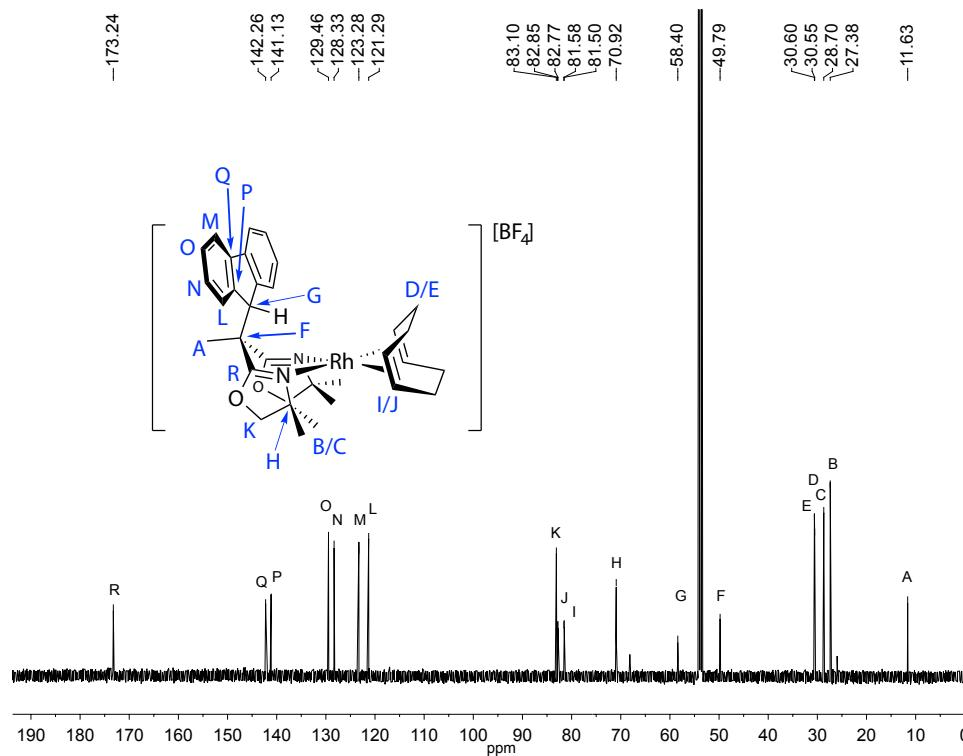
**Figure S51.**  $^{13}\text{C}\{\text{H}\}$  NMR spectrum of  $\{\text{Bo}^{\text{M}}\text{Flu}-\text{H}\}\text{Rh}(\eta^4\text{-C}_8\text{H}_{12})\text{[BF}_4]$  acquired at room temperature in methylene chloride- $d_2$ .
