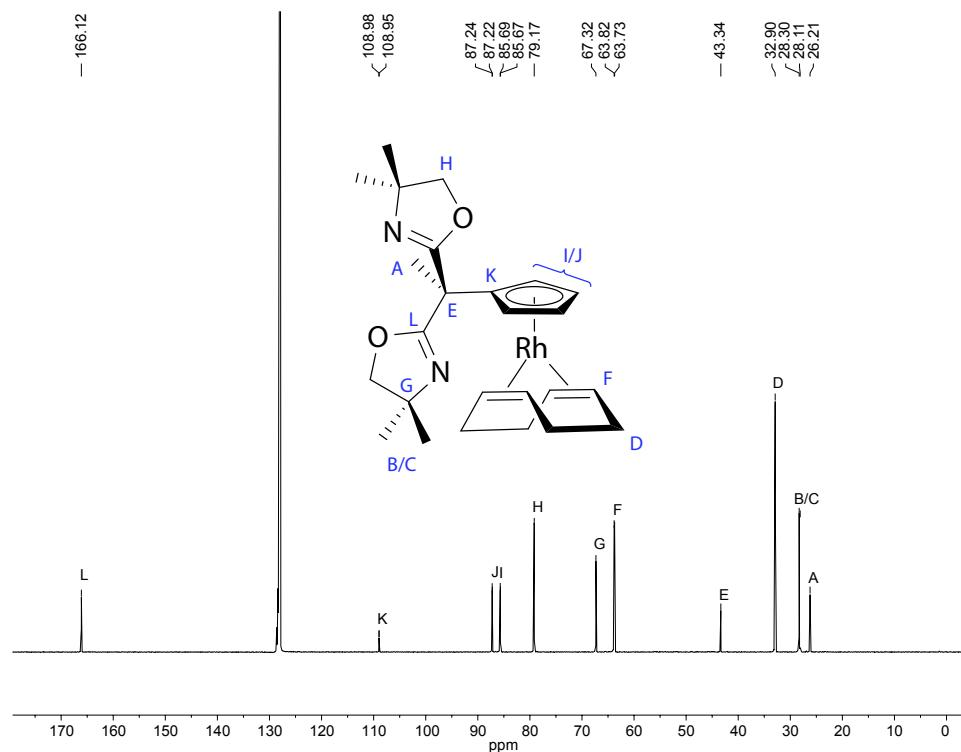
**Figure S26.**  $^{13}\text{C}\{^1\text{H}\}$  NMR spectrum of  $\{\text{Bo}^{\text{M}}\text{Cp}\}\text{Rh}(\eta^4\text{-C}_8\text{H}_{12})$  acquired at room temperature in benzene- $d_6$ .
