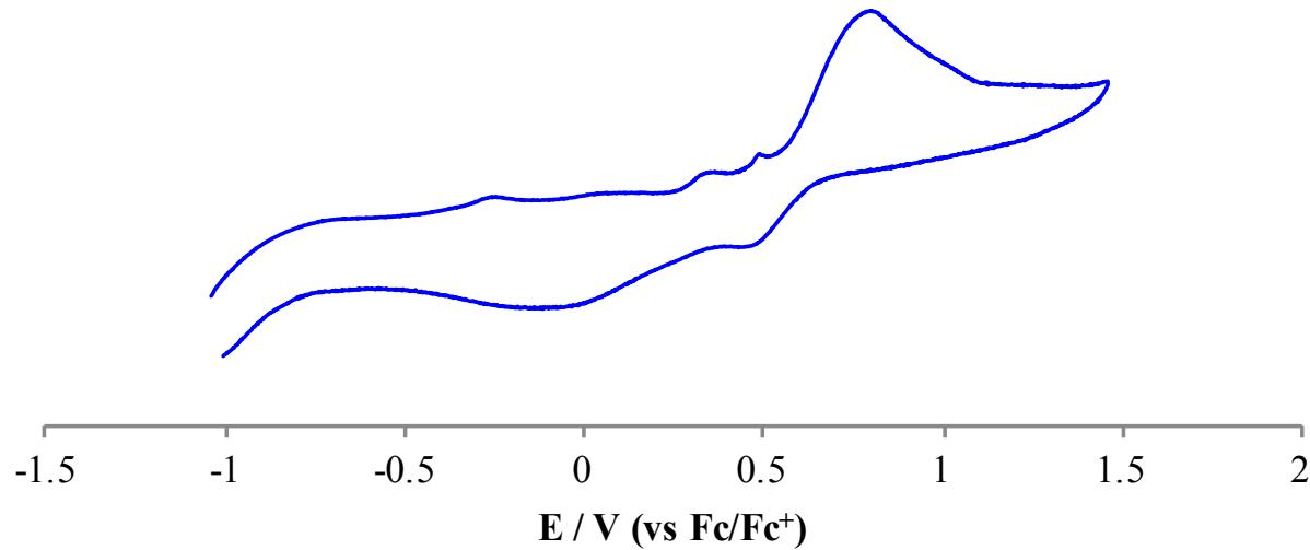
**Figure S2.** Cyclic voltammogram of  $\{\text{Bo}^{\text{M}}\text{Cp}\}\text{RhBr}_2$ . Conditions: 1 mM in  $\text{CH}_3\text{CN}$ , 0.1 M  $[(\text{nBu})_4\text{N}][\text{BF}_4]$ ,  $0.1 \text{ V}\cdot\text{s}^{-1}$ .  $E$  values are given in V versus  $\text{Cp}_2\text{Fe}/\text{Cp}_2\text{Fe}^+$ .
