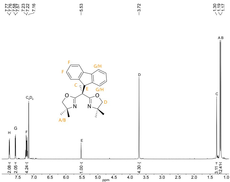
**Figure S35.**  $^1\text{H}$  NMR spectrum of  $\text{Bo}^M\text{FluH}$  acquired at room temperature in benzene- $d_6$ .
