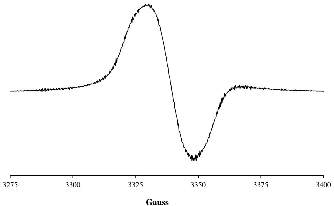
**Figure S17.** CW X-band EPR spectra of  $\{ \text{Bo}^{\text{M}}\text{Flu} \} \text{Rh}(\eta^4\text{-C}_{16}\text{H}_{12}) \text{[BF}_4]$  in 2-methyltetrahydrofuran at 10 K.
