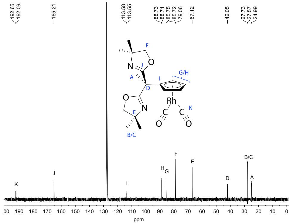
**Figure S23.**  $^{13}\text{C}\{\text{H}\}$  NMR spectrum of  $\{\text{Bo}^{\text{M}}\text{Cp}\}\text{Rh}(\text{CO})_2$  acquired at room temperature in benzene- $d_6$ .
