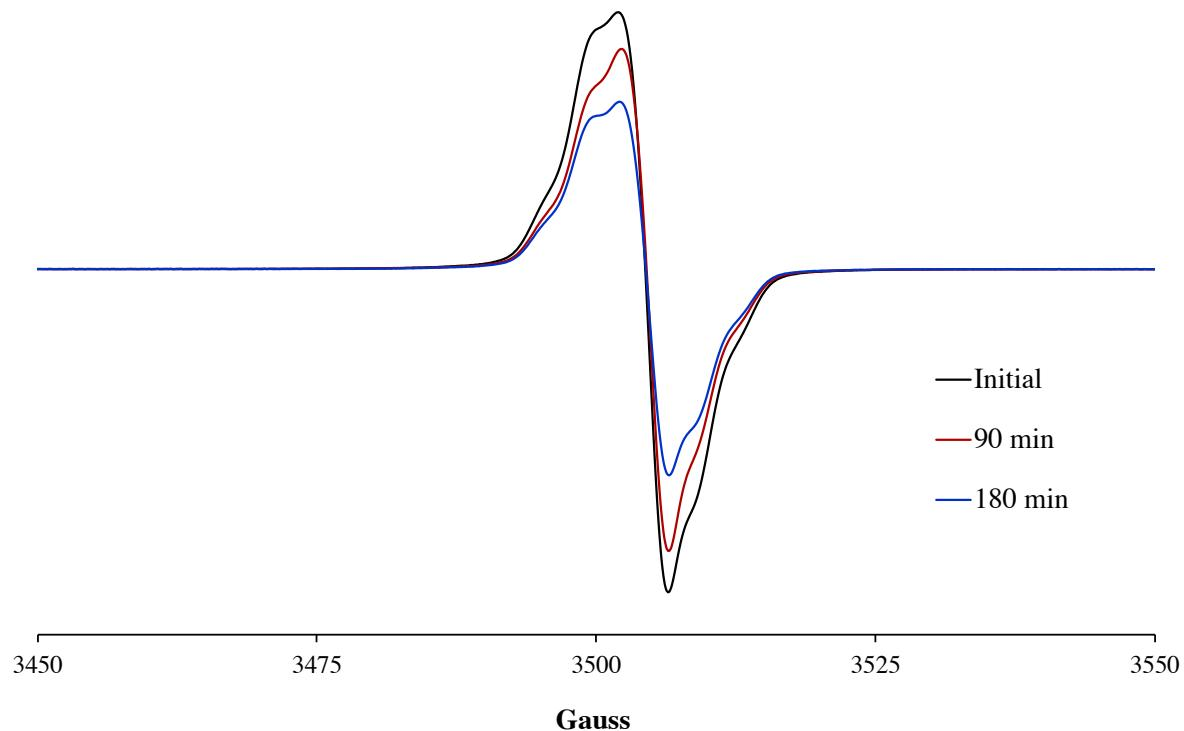
**Figure S12.** CW X-band EPR spectra of  $\{\text{Bo}^{\text{M}}\text{Flu}\}\text{Rh}(\eta^4\text{-C}_8\text{H}_{12})\text{[BF}_4]$  in 2-methyltetrahydrofuran at 298 K, measured at 0 min. (black), 90 min. (red), and 180 min. (blue) after reaction with  $[\text{Ag}]\text{[BF}_4]$ , showing the decay of the odd-electron species at room temperature.
