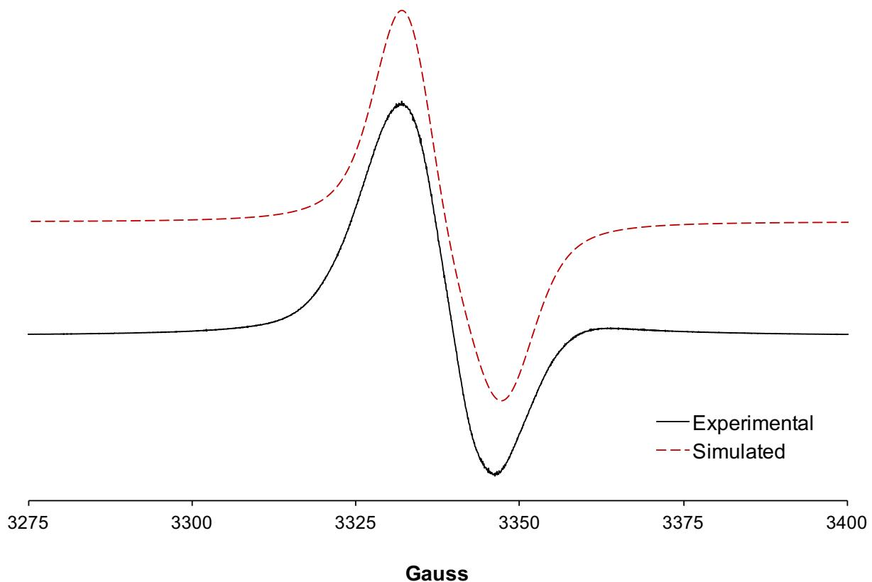
**Figure S16.** CW X-band EPR spectra of  $\{\text{Bo}^M\text{Flu}\}\text{Rh}(\eta^4\text{-C}_{16}\text{H}_{12})\text{[BF}_4]$  in 2-methyltetrahydrofuran with 0.1 M  $[\text{nBu}_4\text{N}]\text{PF}_6$  at 20 K.  $g_x = 2.004$  ( $A_{\text{Rh}} = 25.5$  G)  $g_y = 2.007$  ( $A_{\text{Rh}} = 20.5$  G)  $g_z = 2.009$  ( $A_{\text{Rh}} = 15.2$  G).
