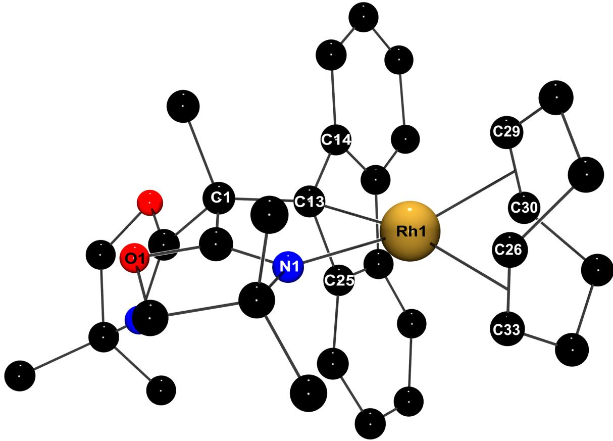
**Figure S65.** Geometry of  $\left[\{C,N\text{-}\kappa^2\text{-Bo}^M\text{Flu}\}\text{Rh}(\eta^4\text{-C}_8\text{H}_{12})\right]^+$  as determined by DFT calculations using the M06-L functional.
