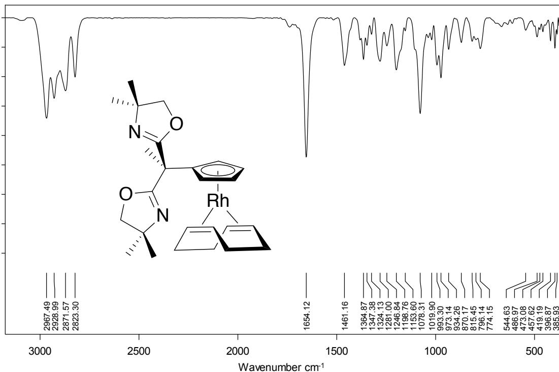
**Figure S27.** Infrared spectrum (KBr) of  $\{\text{Bo}^{\text{M}}\text{Cp}\}\text{Rh}(\eta^4\text{-C}_8\text{H}_{12})$ .
