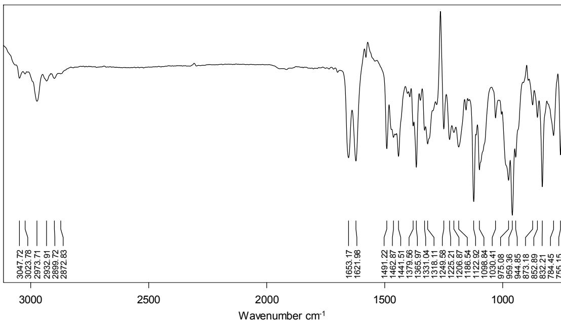
**Figure S7.** Solution ATR of  $\{\text{Bo}^{\text{M}}\text{Flu}\}\text{Rh}(\eta^4\text{-C}_{16}\text{H}_{12})$  as a 0.1 M solution in  $\text{CH}_2\text{Cl}_2$ .
