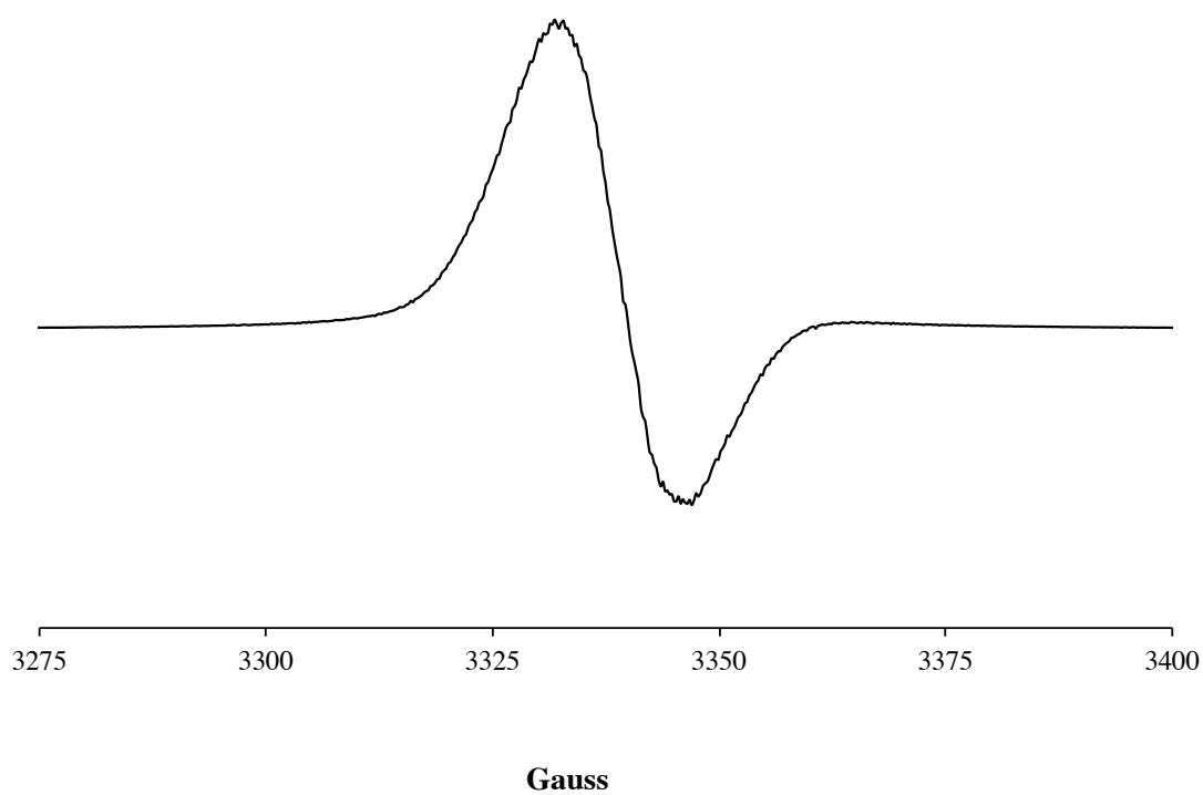
**Figure S15.** CW X-band EPR spectra of  $\{\text{Bo}^{\text{M}}\text{Flu}\}\text{Rh}(\eta^4\text{-C}_{16}\text{H}_{12})\text{][BF}_4$  in 2-methyltetrahydrofuran at 20 K.
