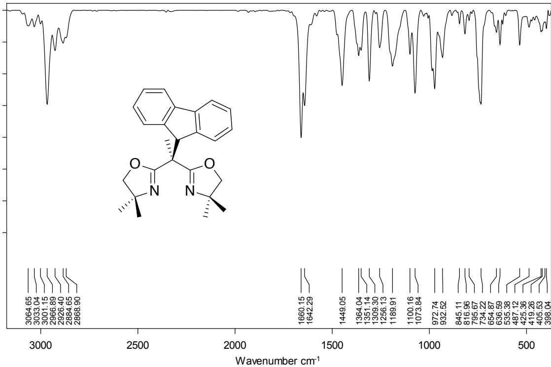
**Figure S37.** Infrared spectrum (KBr) of  $\text{Bo}^{\text{M}}\text{FluH}$ .
