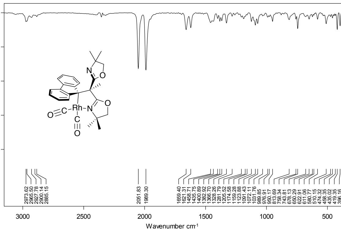
**Figure S46.** Infrared spectrum (KBr) of  $\{\text{Bo}^{\text{M}}\text{Flu}\}\text{Rh}(\text{CO})_2$ .
