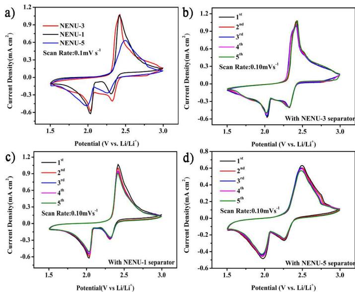
**Figure S10.** (a) Electrochemistry of Li-S batteries compared with PW<sub>12</sub>, NENU-3, NENU-1 and NENU-5 separators. Cyclic voltammetry (CV) curves of the batteries using (b) NENU-3, (c) NENU-1 and (d) NENU-5 separators with the 0.10 mV s<sup>-1</sup>.
