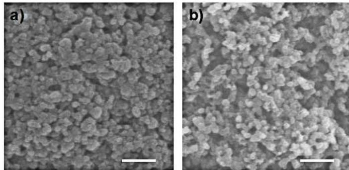
**Figure S2.** (a) The top surface SEM image of the PW<sub>12</sub> separator and (b) SEM image of the top surface of the NENU-3 separator. Scale bar 1 μm.
