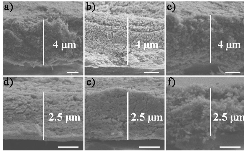
**Figure S4.** The cross section SEM image of the (a)  $\text{PW}_{12}$ , (b)  $\text{PMo}_{12}$ , (c)  $\text{SiW}_{12}$ , (d) NENU-3, (e) NENU-1 and (f) NENU-5 separator by coating. Scale bar 1  $\mu\text{m}$ .
