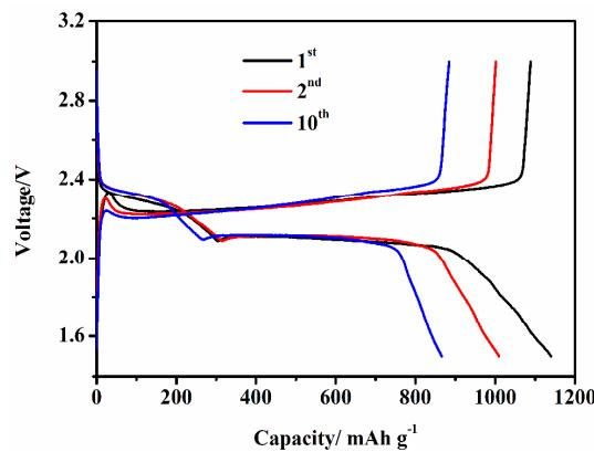
**Figure S6.** Typical galvanostatic charge–discharge profiles of the battery at the 1st, 2nd, and 10th cycles using  $\text{PW}_{12}$  separator when it was discharged to 1.5 V.
