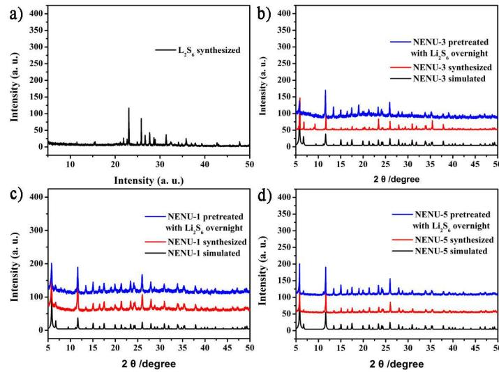
**Figure S12.** (a) XRD patterns of  $\text{Li}_2\text{S}_6$  synthesized. XRD pattern of (b) NENU-3, (c) NENU-1 and (d) NENU-5 pretreated with  $\text{Li}_2\text{S}_6$  (red line), the synthesized (blue line) and simulated XRD of NENU-3, NENU-1 and NENU-5 (black line).
