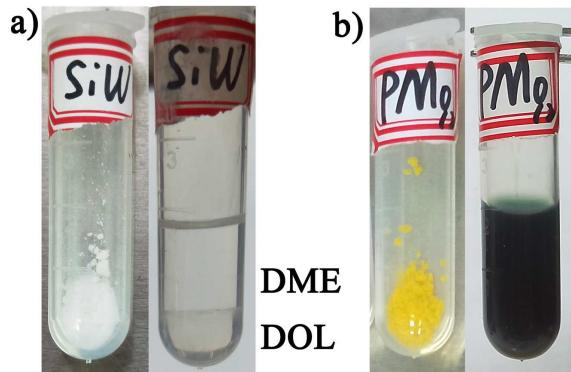
**Figure S15.** (a) The color change between  $\text{SiW}_{12}$  and pretreated with  $\text{Li}_2\text{S}_6$ . (b) The color change between  $\text{PMo}_{12}$  and pretreated with  $\text{Li}_2\text{S}_6$ .
