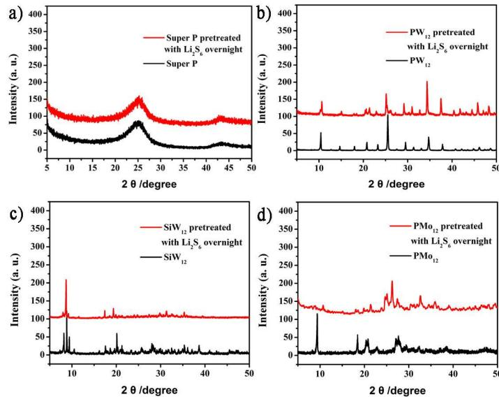
**Figure S11.** XRD patterns of (a) Super P, (b)  $\text{PW}_{12}$ , (c)  $\text{SiW}_{12}$  and (d)  $\text{PMo}_{12}$  pretreated with  $\text{Li}_2\text{S}_6$  (red line) and the XRD of Super P,  $\text{PW}_{12}$ ,  $\text{SiW}_{12}$  and  $\text{PMo}_{12}$  (black line).
