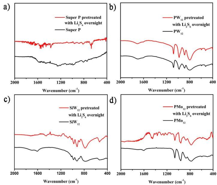
**Figure S13.** IR spectra of (a) Super P, (b)  $\text{PW}_{12}$ , (c)  $\text{SiW}_{12}$ , and (d)  $\text{PMo}_{12}$  pretreated with  $\text{Li}_2\text{S}_6$  (red line) and Super P,  $\text{PW}_{12}$ ,  $\text{SiW}_{12}$  and  $\text{PMo}_{12}$  (black line).
