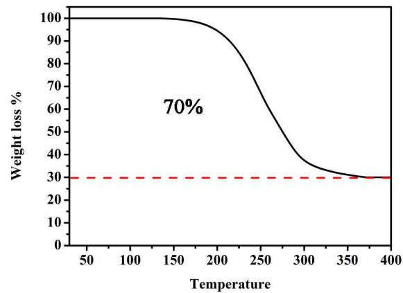
**Figure S1.** TGA curve of the CMK-3/S composite. The weight loss of sulfur in the CMK-3/S composite was measured to 70%.
