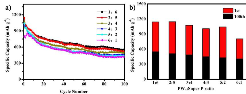
**Figure S5.** (a) The cycling performance comparison and (b) capacities variation of  $\text{PW}_{12}$ /Super P separator with the variation weight ratio of  $\text{PW}_{12}$  to Super P. The separator loading is 0.25  $\text{mg cm}^{-2}$ .
