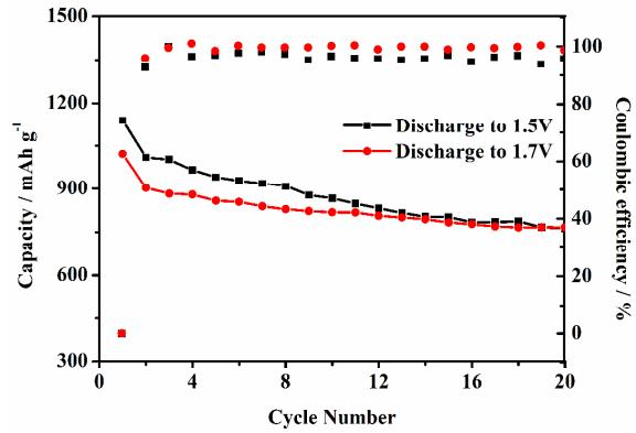
**Figure S7.** Comparative cycle performance of batteries using PW<sub>12</sub> separator when the battery was discharged to 1.7 and 1.5 V.
