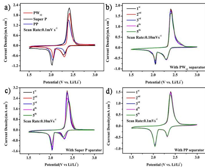
**Figure S8.** (a) Electrochemistry of Li-S batteries compared with PW<sub>12</sub>, Super P and PP separators. Cyclic voltammetry (CV) curves of the batteries using (b) PW<sub>12</sub>, (c) Super P and (d) PP separators with the 0.10 mV s⁻¹.
