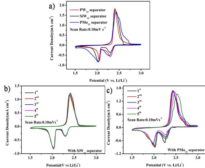
**Figure S9.** (a) Electrochemistry of Li-S batteries compared with PW<sub>12</sub>, SiW<sub>12</sub> and PMo<sub>12</sub> separators. Cyclic voltammetry (CV) curves of the batteries using (b) SiW<sub>12</sub> and (c) PMo<sub>12</sub> separators with the 0.10 mV s<sup>-1</sup>.
