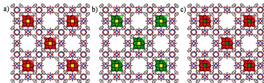
**Figure S16.** The structure and pore size of (a) NENU-3, (b) NENU-5 and (c) NENU-1. Grey: Carbon; Blue: Copper; Red: Oxygen.
