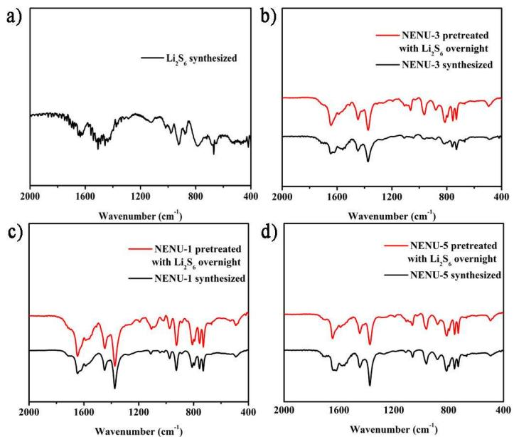
**Figure S14.** IR spectra of  $\text{Li}_2\text{S}_6$  synthesized. IR spectra of (a)  $\text{Li}_2\text{S}_6$ , (b) NENU-3, (c) NENU-1 and (d) NENU-5 pretreated with  $\text{Li}_2\text{S}_6$  (red line) and NENU-3, NENU-1 and NENU-5 synthesized (black line).
