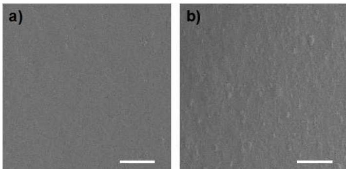
**Figure S3.** (a) The top surface SEM image of the PW<sub>12</sub> separator and (b) SEM image of the top surface of the NENU-3 separator. Scale bar 10 μm.
