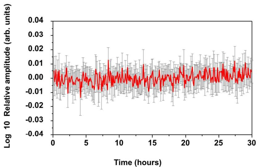
**Figure S1. Measured amplitude variation of detected THz response.** Average amplitude including all frequency components (red) and variation for individual frequency components from 0.3 to 2 THz (gray). Standard variation of all data points is 0.0085 in terms of absorbance, log 10 of relative amplitude, which corresponds to a 1.97% variation in THz signal intensity on a linear scale.
