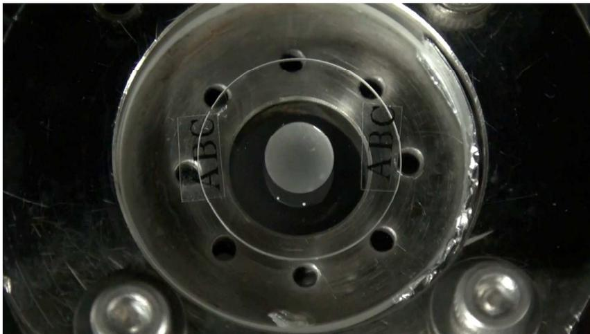
**Movie S2. Movie of NaCl solution freezing after the end of Movie S1.** The frozen NaCl aqueous solution was cooled down to 248 K. The movie shows that the frozen NaCl solution transformed into sodium chloride dihydrate (white in color and corresponding what is depicted in Fig. 2B and Fig. 2C).
