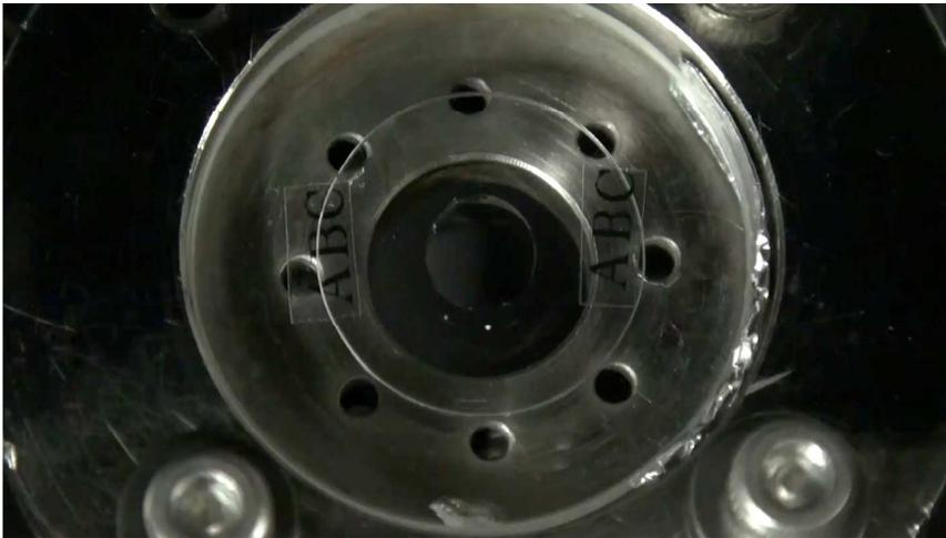
**Movie S1. Movie of freezing NaCl solution.** The 1-mol/L NaCl aqueous solution in a container with polymer sides and a THz-transparent glass plate bottom was cooled down to 250 K. The movie shows that the NaCl solution froze just after the supercooling and hexagonal (I<sub>h</sub>) ice appeared (gray in color and corresponding to what is depicted in Fig. 2A and Fig. 2B). The movie is in real time.
