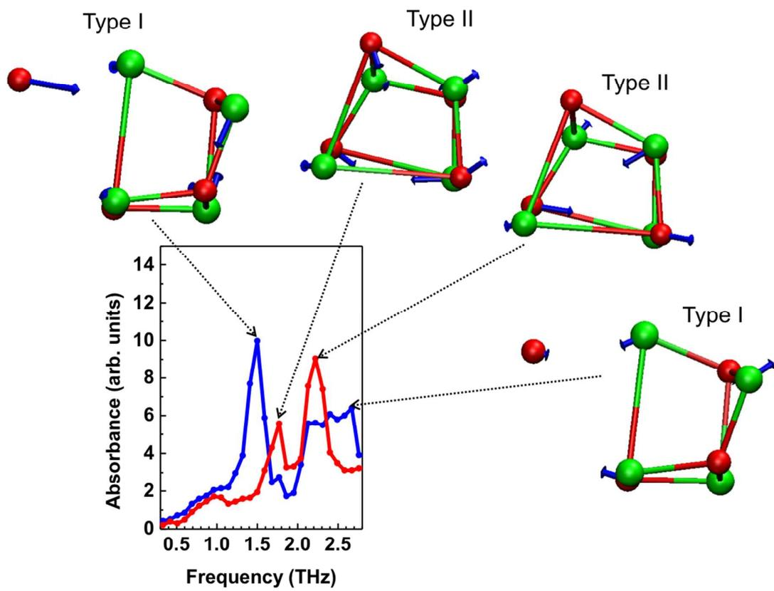
Figure S4. Normal modes of vibration in Type-I and Type-II unit-cell-sized NaCl-cluster particles in ice. The blue arrows indicate the vectors of the normal mode of the vibration. The colors of the ions and ionic bonds in the cluster are the same as those in Fig. 4.
