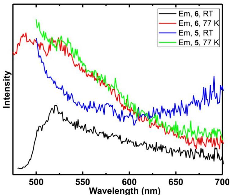
**Figure S2.** Emission spectra of  $^3\text{MLCT}$  phosphorescence of complexes **5** and **6** at RT and at 77 K in a dry, air-free EtOH/MeOH (4:1) solution in a quartz EPR tube.
