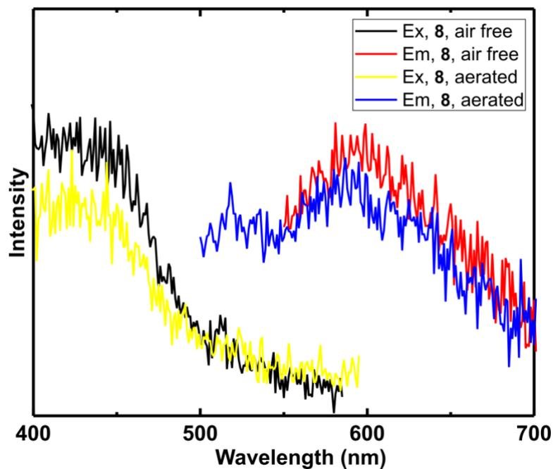
**Figure S4.** Excitation and emission spectra of  $^3\text{MLCT}$  phosphorescence of complex **8** at RT in air-free and aerated EtOH/MeOH (4:1) solution in an airtight quartz cuvette.
