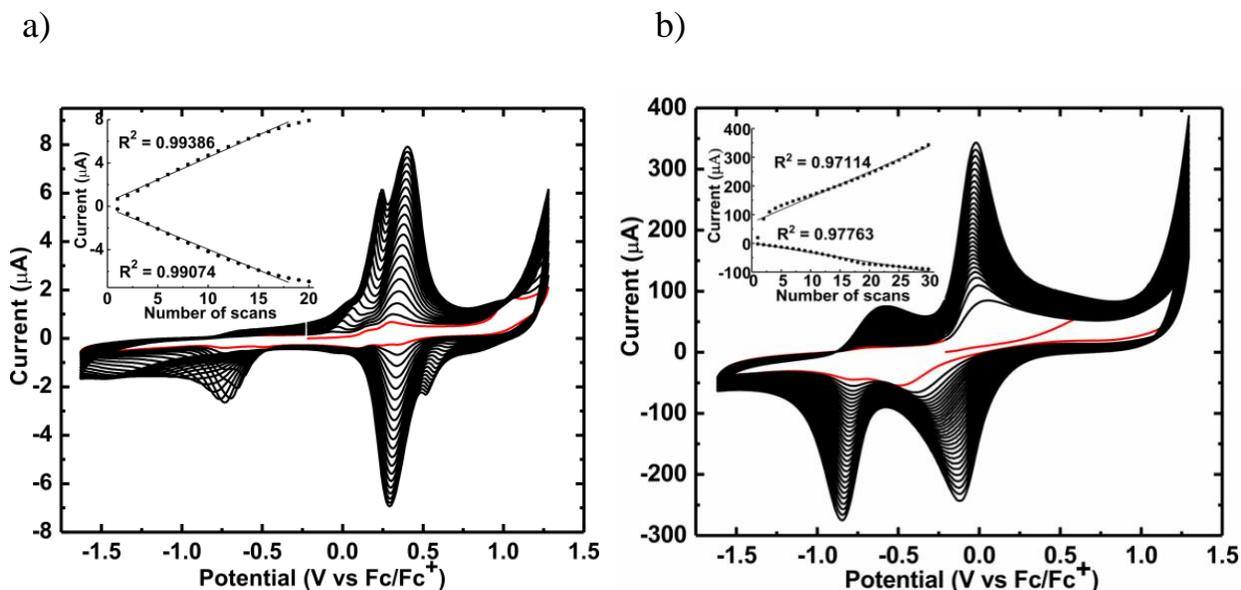
**Figure S1.** Electropolymerization of ruthenium complexes, initial scans shown in red. Insets: Current vs. number of scans. a) **5** (left) b) **6** (right).
