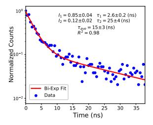
Figure S1: Time resolved PL intensity data and bi-exponential decay fitting
