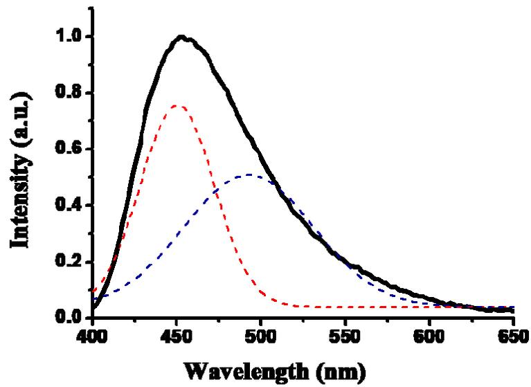
Figure S1: PL spectrum fitted by two Gaussian functions for as-prepared, diluted Si-CNDs.
