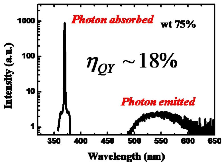
Figure S6: Experimental data of absolute PL-QY measurement for cross-linked Si-CNDs.
