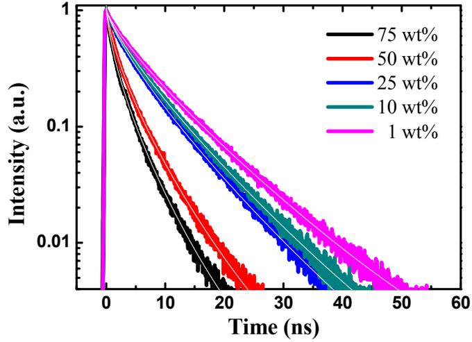
**Figure S7: Fitting results for cross-linked Si-CND thin films with different loadings**
