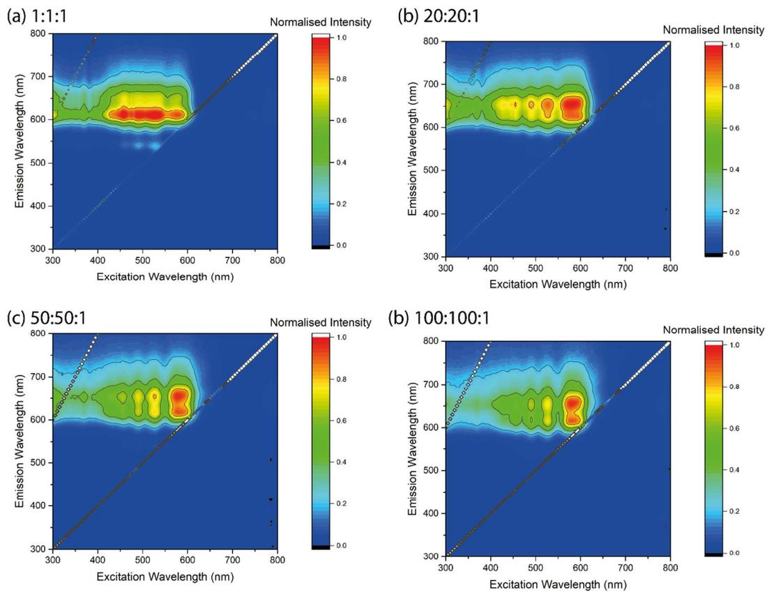
Figure S8: Two-dimensional emission/excitation spectra clearly showing that, under any excitation, emission occurs from the red dye at 650 nm.
