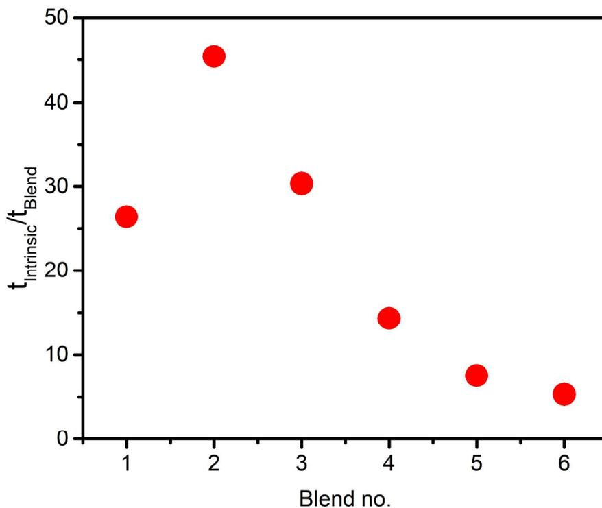
Figure S7: Relative transfer efficiency of the different fabricated PMMA composites, taken by measuring the lifetime of red dye in the blend compared to its intrinsic lifetime when isolated. An almost 50-fold increase in its lifetime is seen when incorporating into the dye into the blend structure, emphasising efficient FRET.
