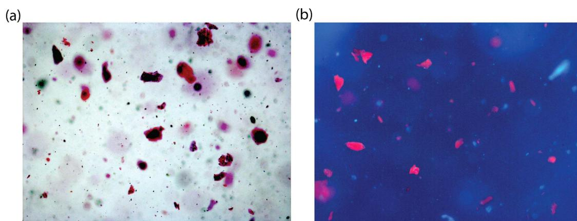
Figure S4: PMMA/dye LHCs dispersed within an 80:20 lauryl methacrylate and ethylene glycol dimethacrylate matrix (a) under white light and (b) under 365 nm UV lamp illumination.
