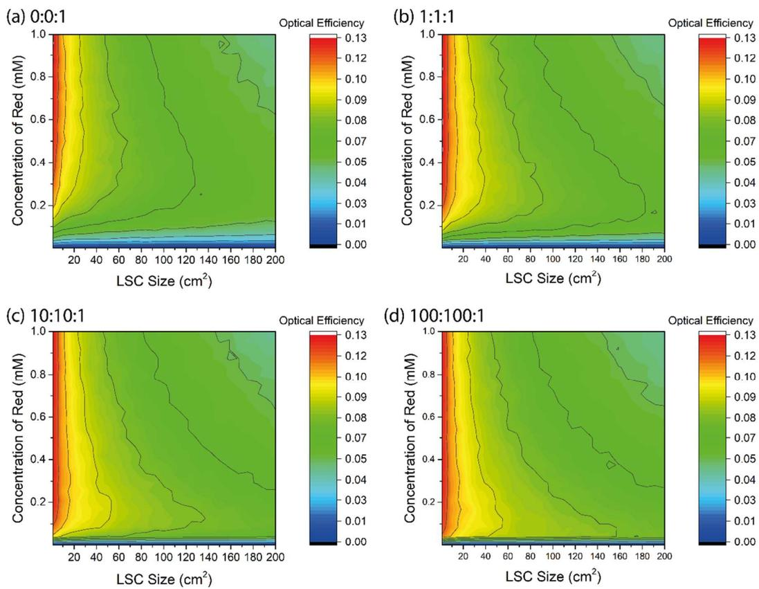
Figure S9: Results of Monte-Carlo ray tracing simulations on different ratio LHCs. Full details on the simulations can be found in the methods section.
