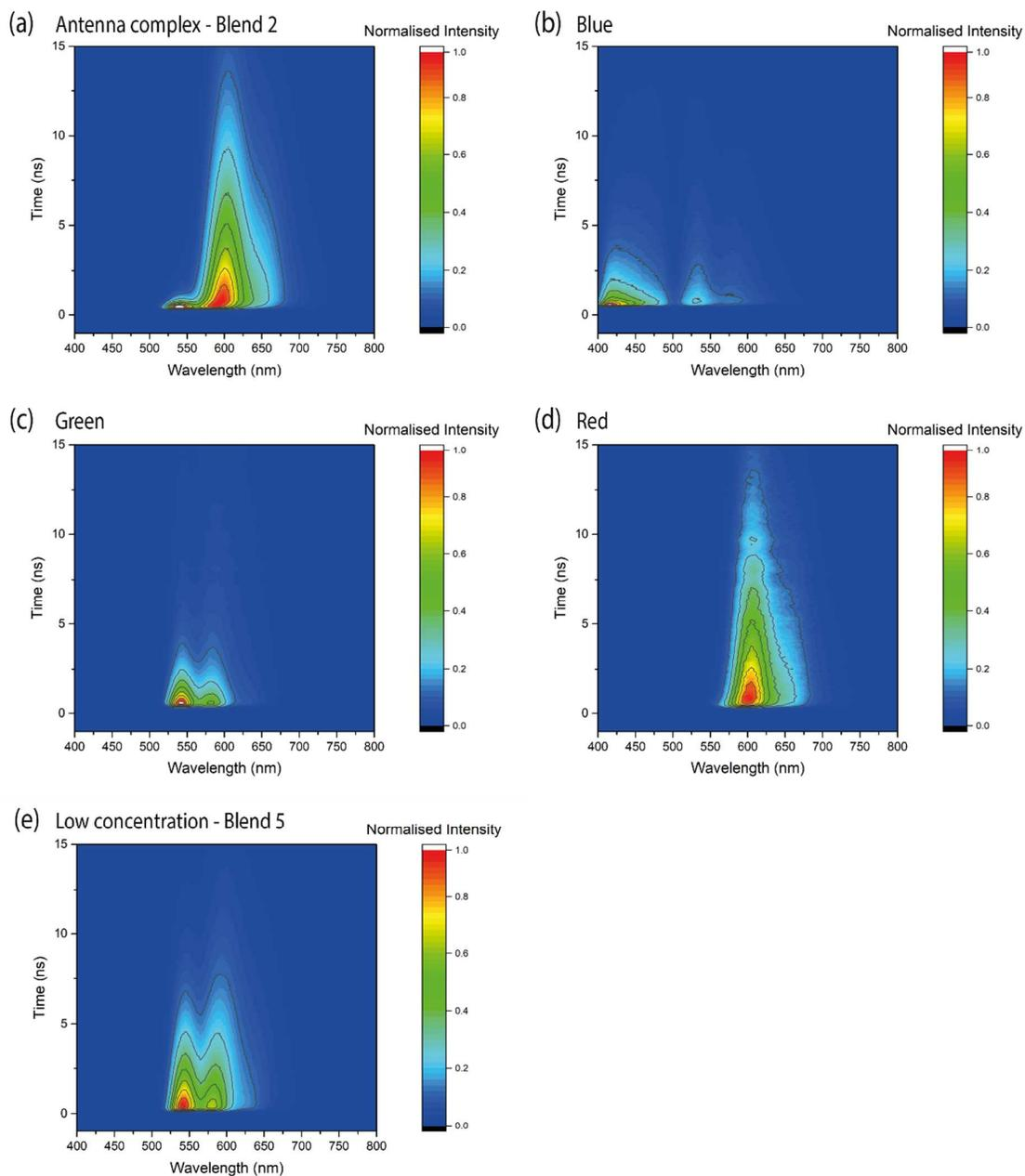
Figure S6: Transient photoluminescence of different PMMA composites. Lowering the concentration of dyes within the blend leads to dual emission (e) and reduces the overall efficiency.
