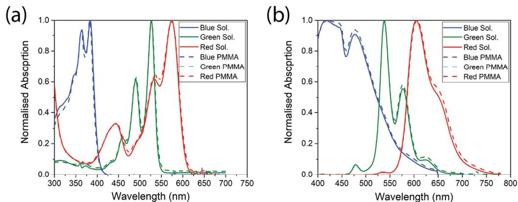
Figure S1: Comparison of absorption and emission spectra shifts upon incorporation into a PMMA matrix (0.1 w/w %).
