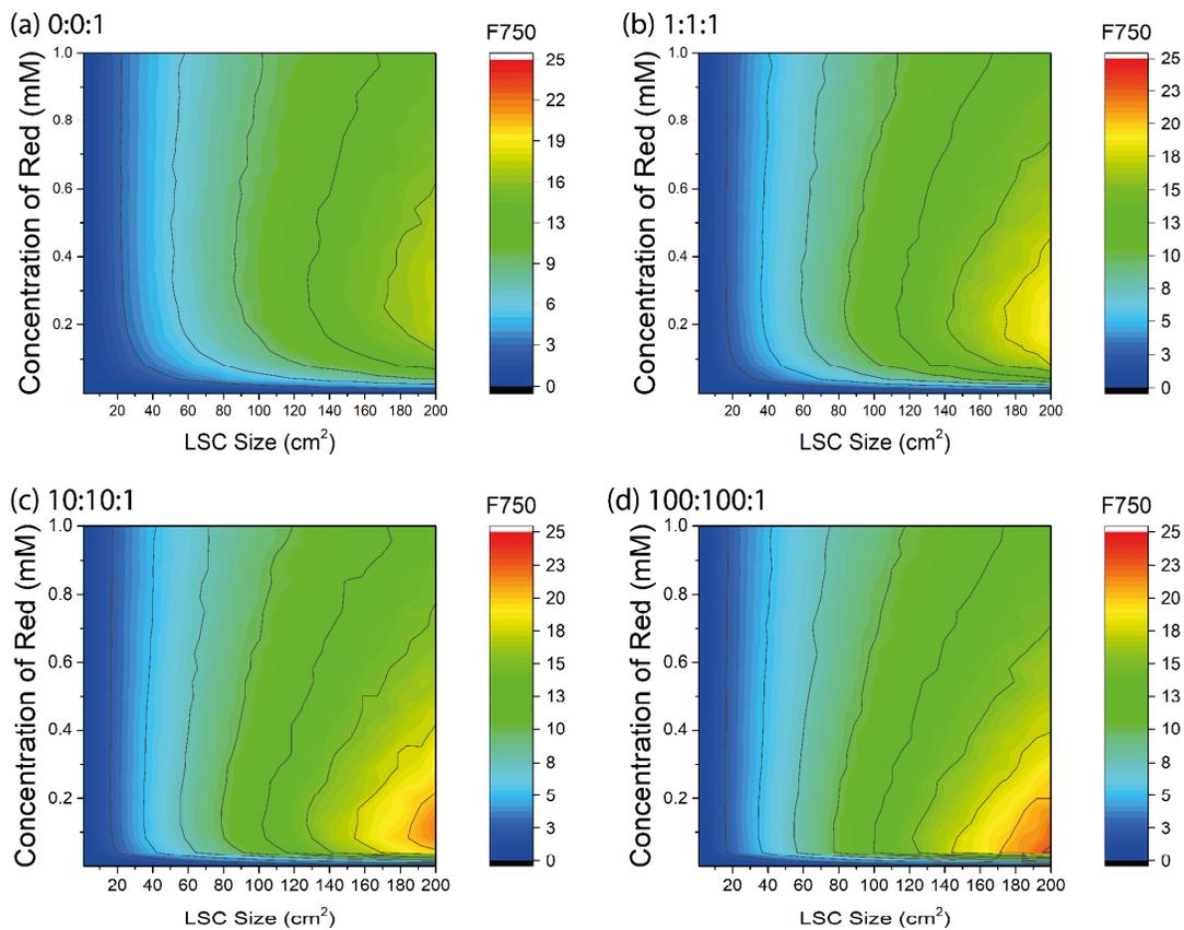
Figure S10: Results of Monte-Carlo ray tracing simulations on different ratio LHCs with a flux threshold of 750 nm. Full details on the simulations can be found in the methods section of the main text.
