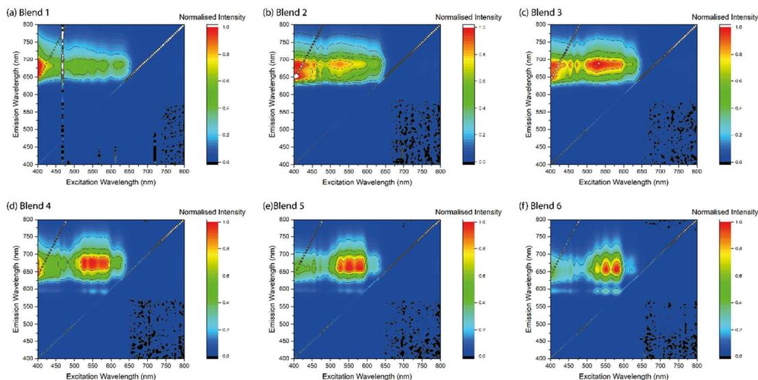
Figure S2: Two-dimensional emission/excitation spectra clearly showing that for concentrated complexes, under any excitation, emission occurs from the red dye at 650 nm but at lower concentrations emission from the green dye at 600 occurs.
