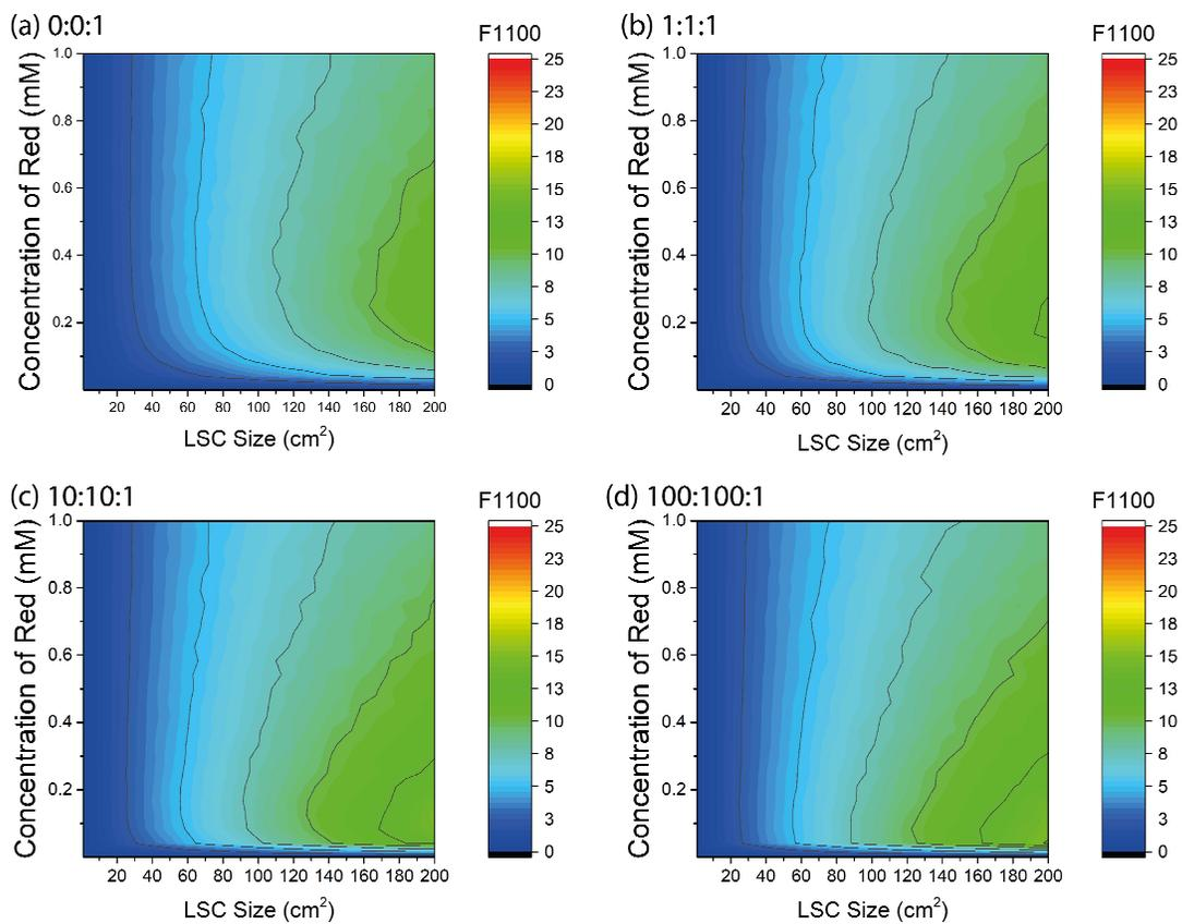
Figure S11: Results of Monte-Carlo ray tracing simulations on different ratio LHCs with a flux threshold of 1100 nm. Full details on the simulations can be found in the methods section of the main text.
