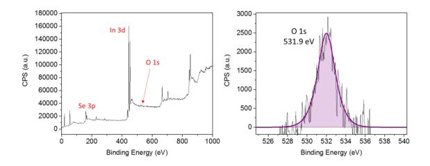
**Figure S3. XPS of oxygen 1s core orbital peak.** The position of the peak is found to be 531.9 eV, which is assigned to physisorbed oxygen. No oxide peak is detected at 530 eV. The amount of surface physisorbed oxygen is found to be very low, at 3.4%.
