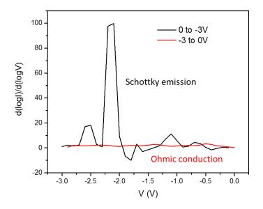
**Figure S6. Conduction mechanism in MBE grown**  $\alpha$ -In<sub>2</sub>Se<sub>3</sub>. For the voltage sweep from - 3 to 0 V (red), ohmic behavior is observed, in which  $dlog(I)/dlog(V) \approx 1$ . For the voltage sweep from 0 to -3 V (black), increasing slope of log(I)-log(V) curve is observed, which indicates Schottky barrier controlled conduction.
