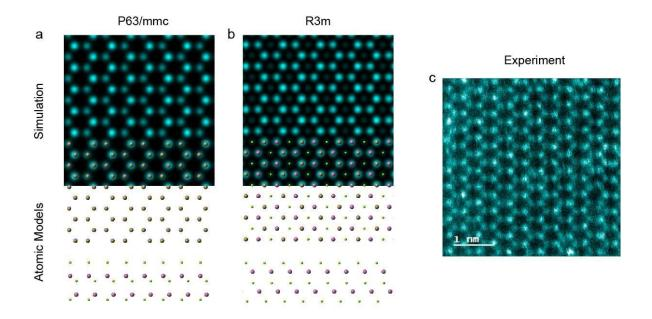
**Figure S4. Identifying the structural phase of \alpha-In<sub>2</sub>Se<sub>3</sub>. (a) Simulation of the** *P63/mmc***<sup>1</sup> and (b)** *R3m***<sup>2</sup> structural phases. Atomic models are overlaid, and the side views are depicted in the lower panels. (c) Atomic-resolution STEM-ADF image of the as-grown \alpha-In<sub>2</sub>Se<sub>3</sub> monolayer film, which indicates that it belongs to the** *P63/mmc* **space group.**
