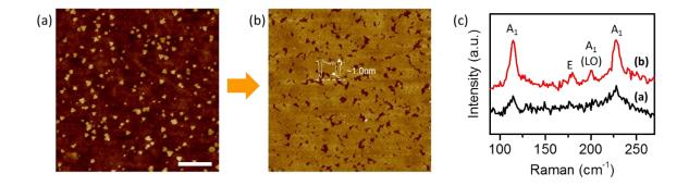
**Figure S1. MBE growth of monolayer InSe.** AFM topography of (a) the initial growth of InSe and (b) the subsequent coalescence to form a continuous monolayer. (c) Raman spectra of the respectively InSe grown at the different stages shown in (a) and (b). Scale bar for both AFM images: 600 nm.
