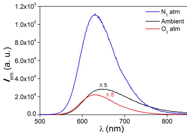
**Supporting Figure S38.** Emission spectra of **PQ3** in PBS:DMSO (9:1 v/v) mixture at various conditions.
