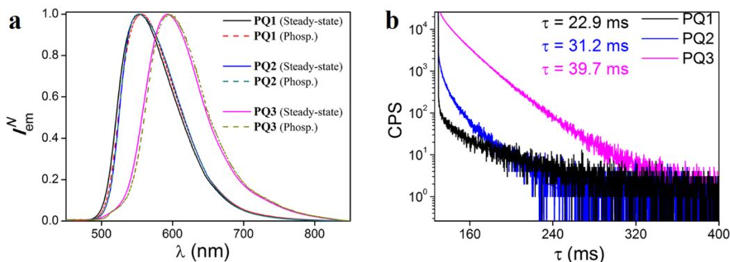
**Supporting Figure S32.** (a) Stead state emission and phosphorescence of **PQ1**, **PQ2**, and **PQ3** in crystals. (b) Lifetimes of the conjugates.
