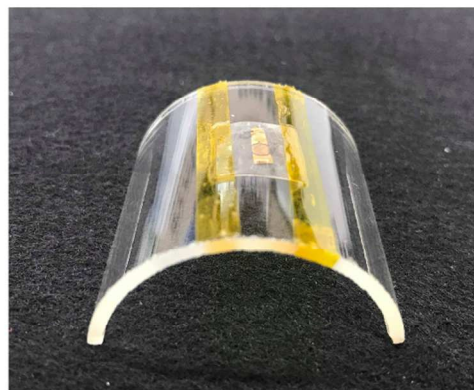
Figure S5. (a) The curvature of the curved substrates, including 1.82 cm, 1.14 cm, 0.74 cm, and 0.52 cm. (b) Photograph of device under bending.
