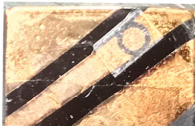
Figure S7. (a) PVA material was spin-coated on SiO 2 substrate. (b) The final device after transferring graphene and depositing chlorophyll.
