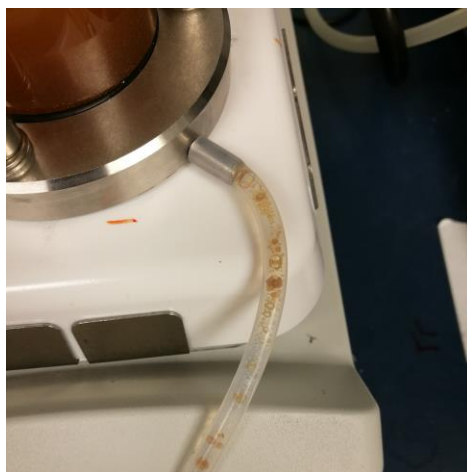
Figure S7. Crude oil in permeate solution in the case of nascent PVDF membrane
