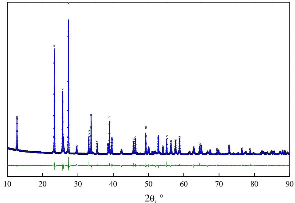
**Figure S1.** XRD pattern and Rietveld refinement for pristine  $\text{MoO}_3$ .
