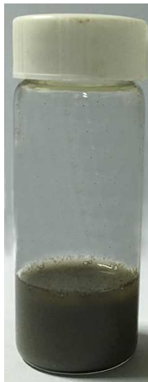
Figure S-1. The photograph of exfoliated h-BN@PDA dispersion prepared via ball milling in water.
