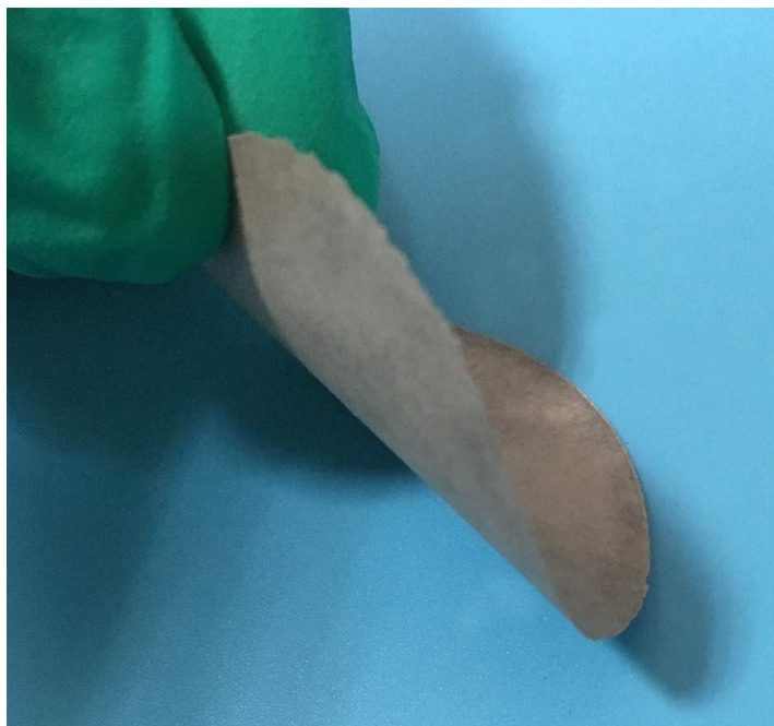
Figure S-8. The photograph of exfoliated h-BN@PDA/CNC composite when folded.
