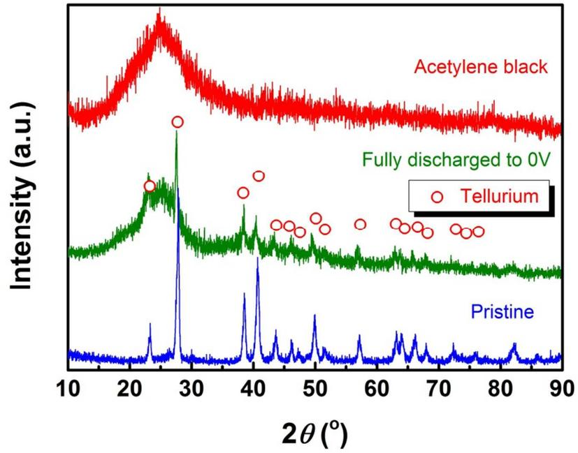
Figure S3: *Ex situ* X-ray diffraction patterns of tellurium cathode: pristine and fully discharged to 0 V.
