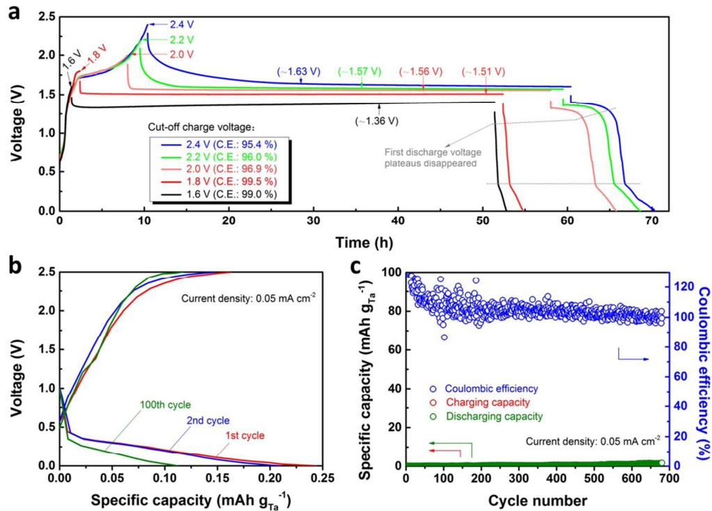
**Figure S4:** (a) The shelf life test of the Al-Te battery. (b) Charge/discharge curves of the tantalum foil. (c) Capacity as a function of cycle number of the tantalum foil at a current density of 0.05 mA/cm<sup>2</sup>. The capacity of tantalum foil is less than 0.5 mAh/g<sub>Ta</sub> over 600 cycles, which indicates that the side reaction caused by tantalum is negligible.
