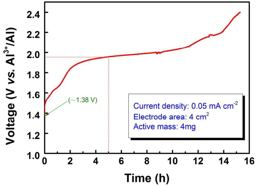
Figure S1: Voltage-time plot of galvanostatic electrolysis at a current density of 0.05 mA/cm<sup>2</sup>.
