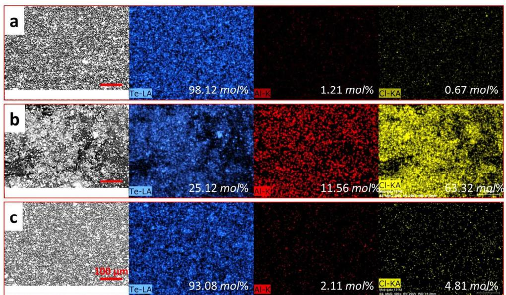
**Figure S2:** EDS of tellurium electrodes: (a) pristine, (b) charged to 2.4 V and (c) reverted to 0.5 V by discharge from 2.4 V.
