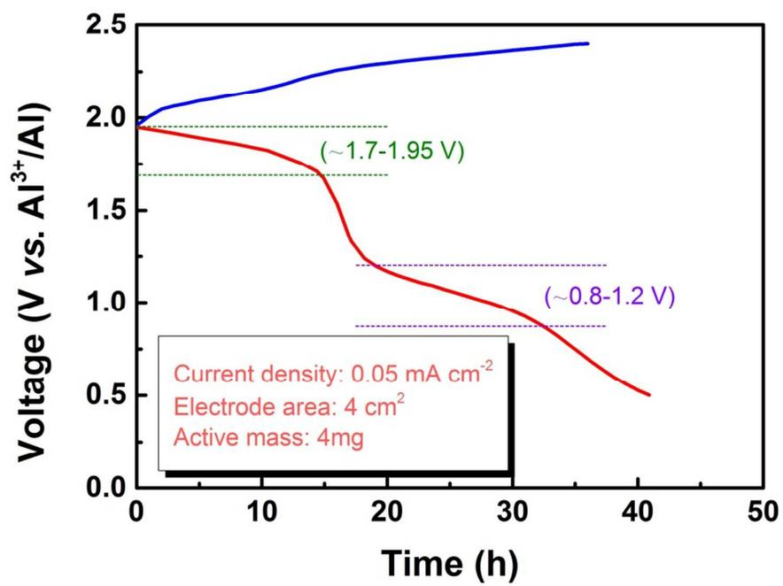
**Figure S5:** Galvanostatic charge and discharge curves of the novel Al-S battery at a current density of 0.05 mA/m<sup>2</sup>.
