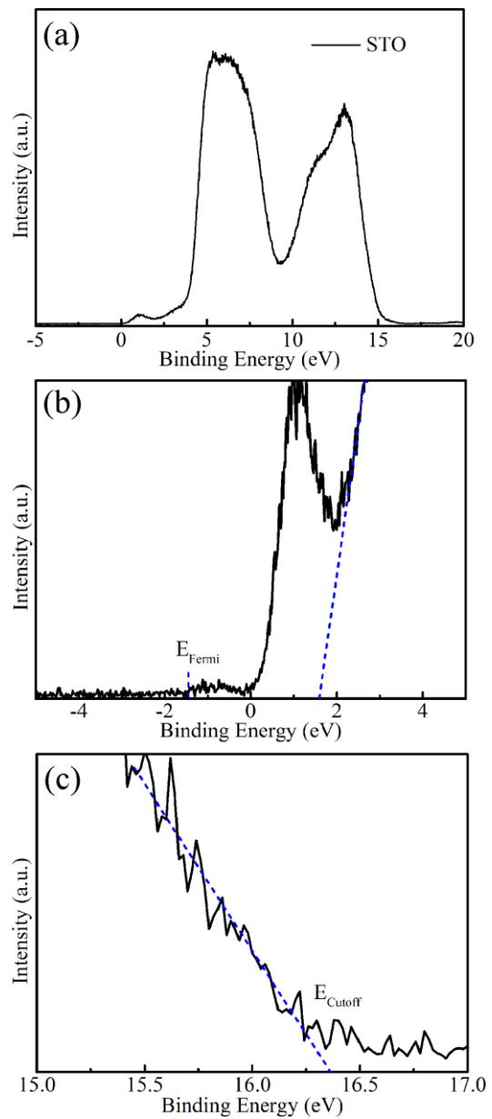
**Figure S13.** (a) UPS spectrum of STO, and (b-c) locally magnified spectrum of (a).
