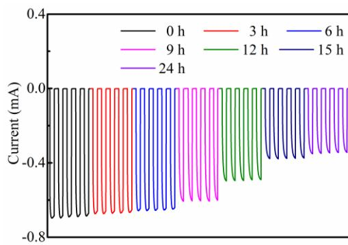
**Figure S11.** Stability measurement of positively poled STO-1 devices under white light illumination after placing in air for different hours.
