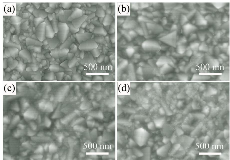
**Figure S1.** SEM images of (a) FTO, and STO layers with different spin-coated cycles: (b) 1 cycle, (c) 2 cycles, and (d) 3 cycles.
