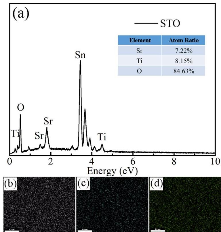
**Figure S6.** (a) EDX pattern of pristine STO film, and corresponding elemental mapping: (b) Sr, (c) Ti, and (d) O.
