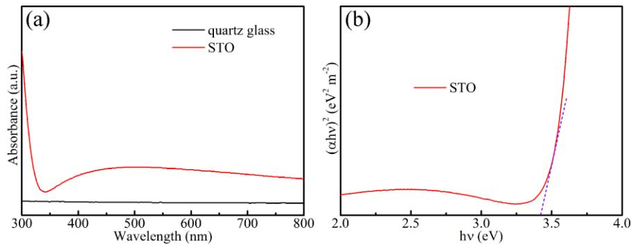
**Figure S12.** (a) The absorption spectra of pristine STO film and quartz glass. (b) The relationship between the absorption coefficient  $\alpha$  and the energy band gap of STO.
