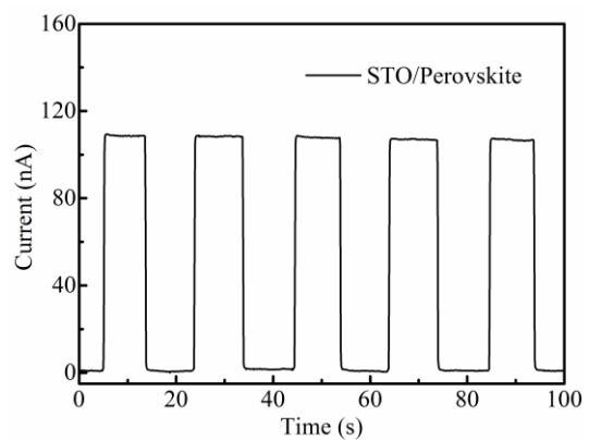
**Figure S8.**  $I$ - $t$  curve of the STO/Spiro-OMeTAD photodetector under white light illumination at 0 V.
