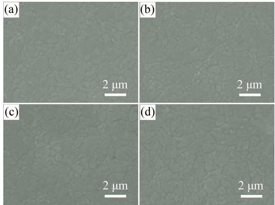
**Figure S4.** Low-magnified SEM images of (a) perovskite, and STO/perovskite hybrid structure with different spin-coated cycles of STO: (b) 1 cycle, (c) 2 cycles, and (d) 3 cycles.
