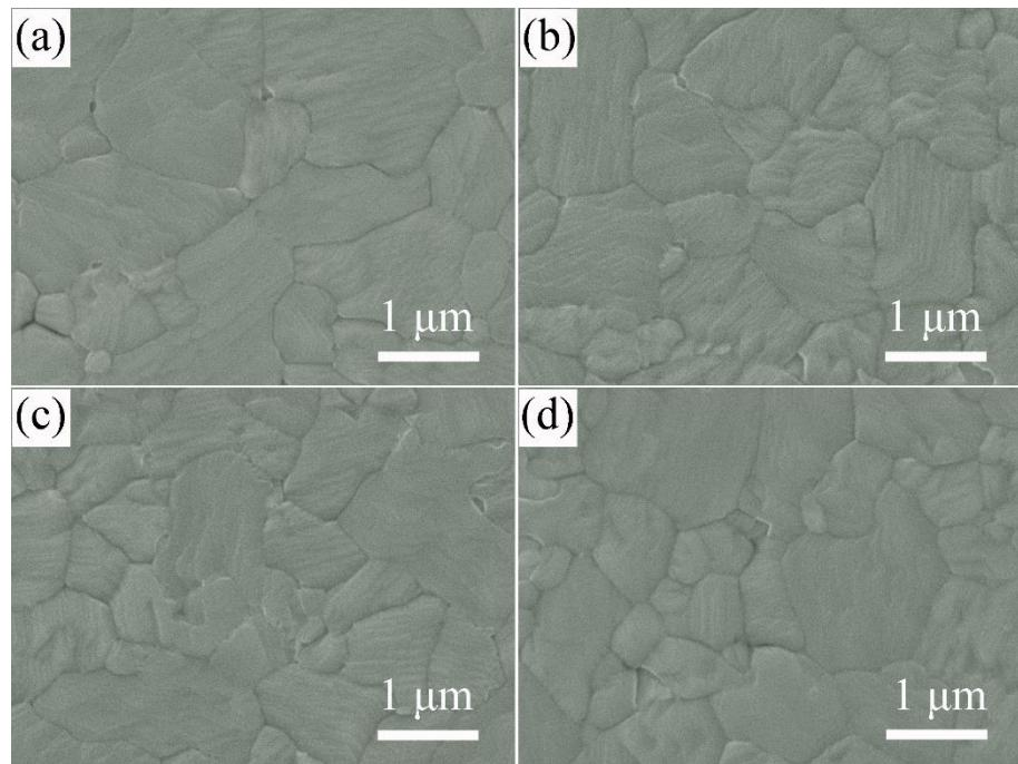
**Figure S3.** SEM images of (a) perovskite, and STO/perovskite hybrid structure with different spin-coated cycles of STO: (b) 1 cycle, (c) 2 cycles, and (d) 3 cycles.
