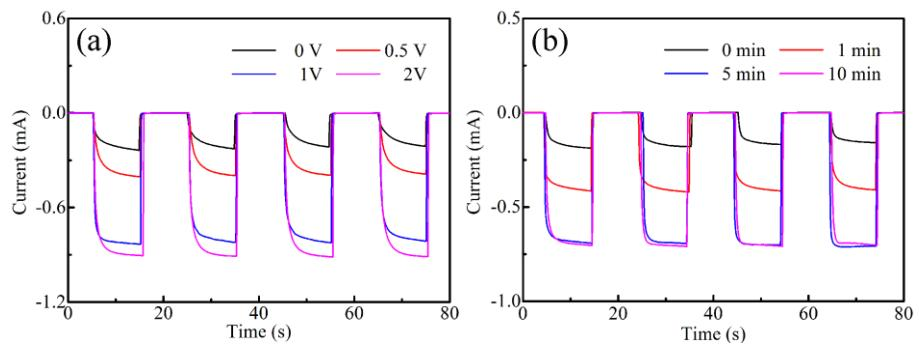
**Figure S10.** *I*-*t* curves of the as-prepared STO-1 under white light illumination at 0 V with different polarization treatment process: (a) different polarization voltage with certain time of 5 min, (b) different polarization time with certain voltage of 1 V.
