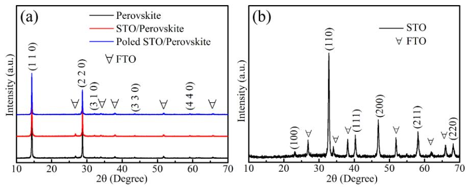
**Figure S7.** XRD patterns of (a) perovskite, STO/Perovskite, and positively poled STO/Perovskite, and (b) pristine STO film.
