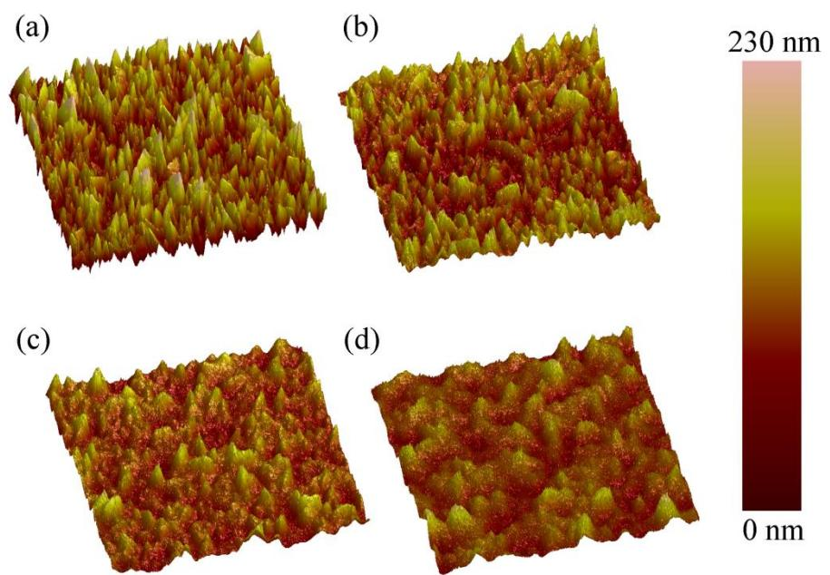
**Figure S2.** 3D AFM topography images of (a) FTO, and STO layers with different spin-coated cycles: (b) 1 cycle, (c) 2 cycles, and (d) 3 cycles.
