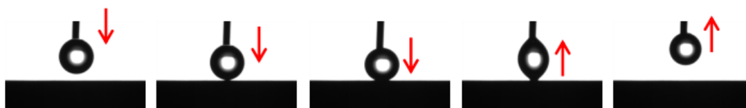
Figure S25. Water contact angle test sequence for FC-CNT membrane surface.
