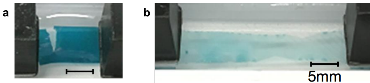
Figure S39. T-0 (a) and T-75 (b) films strained to their respective failure points.
