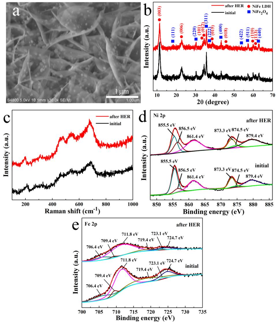
**Figure S13.** The SEM image (a), the XRD pattern (b), the Raman spectrum (c), the XPS spectra of Ni 2p (d) and Fe 2p (e) of NiFe<sub>2</sub>O<sub>4</sub>/NiFe LDH after 20 h HER chronopotentiometry test at overpotential of 150 mV.
