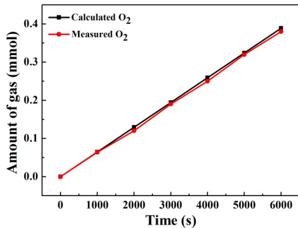
**Figure S10.** The electrocatalytic efficiency of NiFe<sub>2</sub>O<sub>4</sub>/NiFe-LDH for OER at 100 mA cm<sup>-2</sup>.
