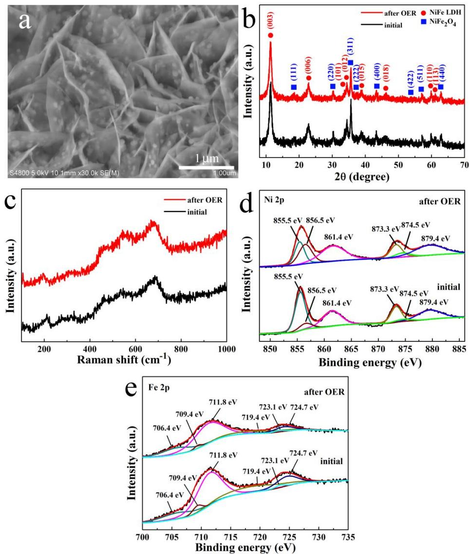
**Figure S9.** The SEM image (a), the XRD pattern (b), the Raman spectrum (c), the XPS spectra of Ni 2p (d) and Fe 2p (e) of NiFe<sub>2</sub>O<sub>4</sub>/NiFe LDH after 20 h OER chronopotentiometry test at overpotential of 202 mV.
