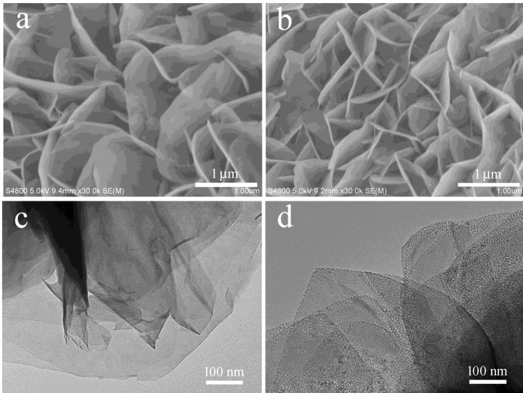
**Figure S3.** (a, b) The SEM images of the  $\text{NiFe}_2\text{O}_4$  precursor nanosheet array and the  $\text{NiFe}_2\text{O}_4$  nanosheet array, respectively. (c, d) The TEM images of  $\text{NiFe}_2\text{O}_4$  precursor nanosheets and  $\text{NiFe}_2\text{O}_4$  nanosheets, respectively.
