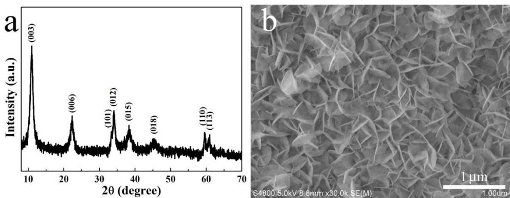
**Figure S5.** The XRD pattern (a) and SEM image (b) of the product with  $\text{FeCl}_3 \cdot 6\text{H}_2\text{O}$  instead of  $\text{FeCl}_2 \cdot 6\text{H}_2\text{O}$ .
