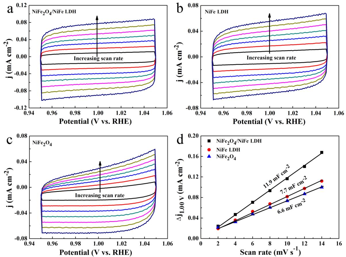
**Figure S14.** The cyclic voltammograms of  $\text{NiFe}_2\text{O}_4/\text{NiFe LDH}$  (a),  $\text{NiFe LDH}$  (b), and  $\text{NiFe}_2\text{O}_4$  (c) at different scan rates of 2, 4, 6, 8, 10, 12, and 14  $\text{mV s}^{-1}$ . (d) The capacitive currents at 1.00 V versus RHE with different scan rates.
