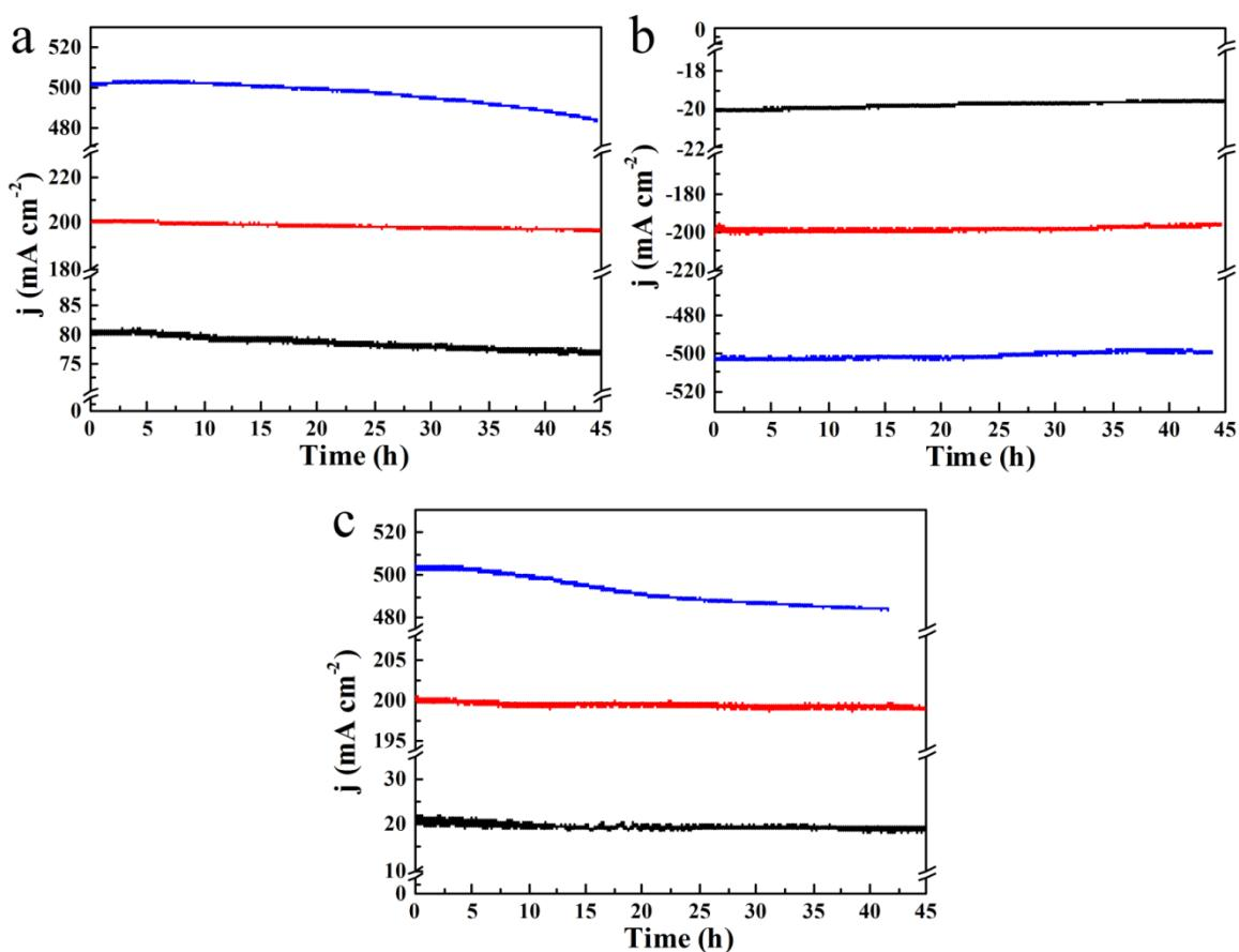
**Figure S17.** Chronoamperometric curves of  $\text{NiFe}_2\text{O}_4/\text{NiFe}$  LDH electrodes for exceeding 40 h for (a) OER at overpotentials of 202, 230 and 242 mV, respectively, (b) HER at overpotentials of 150, 259 and 298 mV, respectively, and (c) overall water splitting at a cell voltage of 1.60, 1.82 and 1.94 V, respectively.
