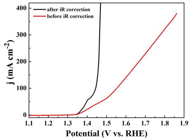
**Figure S8.** The OER LSV curves of  $\text{NiFe}_2\text{O}_4/\text{NiFe-LDH}$  electrode with and without iR-correction.
