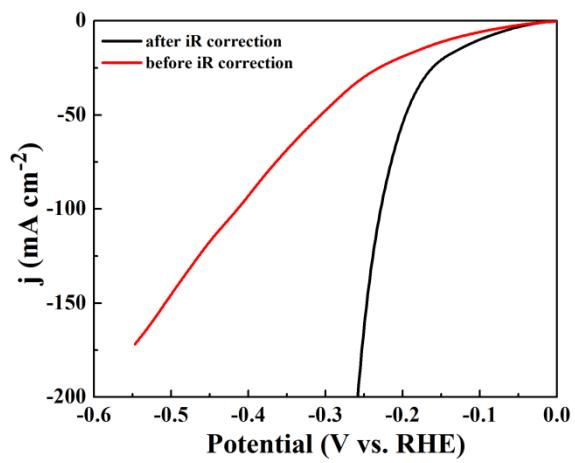
**Figure S12.** The HER LSV curves of  $\text{NiFe}_2\text{O}_4/\text{NiFe-LDH}$  electrode with and without iR-correction.
