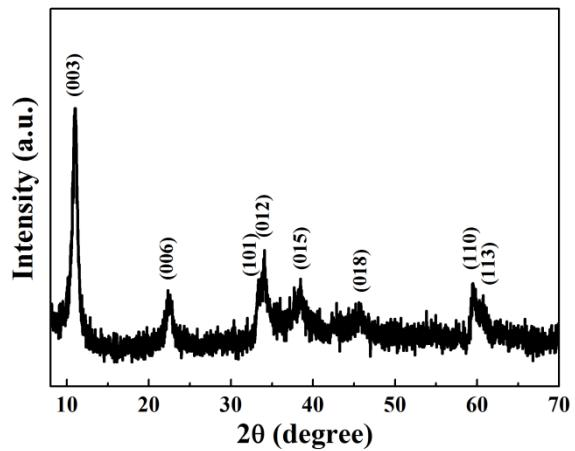
**Figure S1.**The XRD pattern of the precursor with Ni/Fe ratio of 1:2 in 5 mL of deionized water and 30 mL of methanol, showing it was the NiFe LDH phase.
