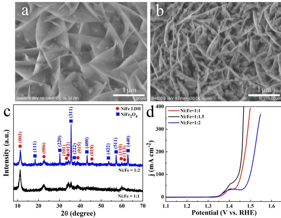
**Figure S7.** (a, b) The SEM images of the NiFe<sub>2</sub>O<sub>4</sub>/NiFe LDH products with Ni/Fe ratio of 1:1 and 1:2, respectively. (c) The XRD patterns of the NiFe<sub>2</sub>O<sub>4</sub>/NiFe LDH products with Ni/Fe ratio of 1:1 and 1:2. (d) The OER polarization curves of the NiFe<sub>2</sub>O<sub>4</sub>/NiFe LDH products with different ratio of Ni and Fe.
