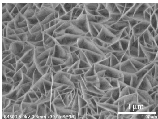
**Figure S2.** The SEM image of the NiFe LDH nanosheet array.
