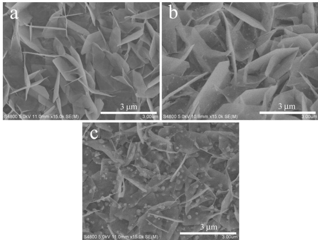
**Figure S6.** Time resolved experiments of  $\text{NiFe}_2\text{O}_4/\text{NiFe}$  LDH. (a) 30 min, (b) 60 min, and (c) 90 min.
