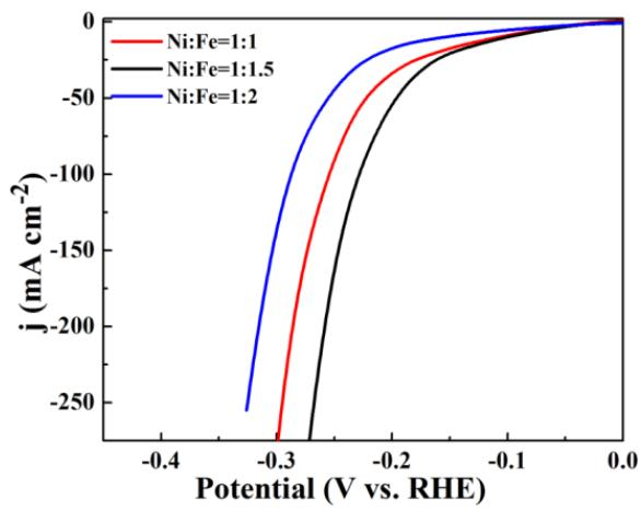
**Figure S11.** The HER polarization curves of the  $\text{NiFe}_2\text{O}_4/\text{NiFe}$  LDH products with different ratio of Ni and Fe.
