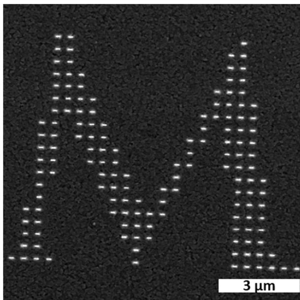
Figure S10. Scanning electron microscopy image of the letter “M” in the text “Melbourne”.
