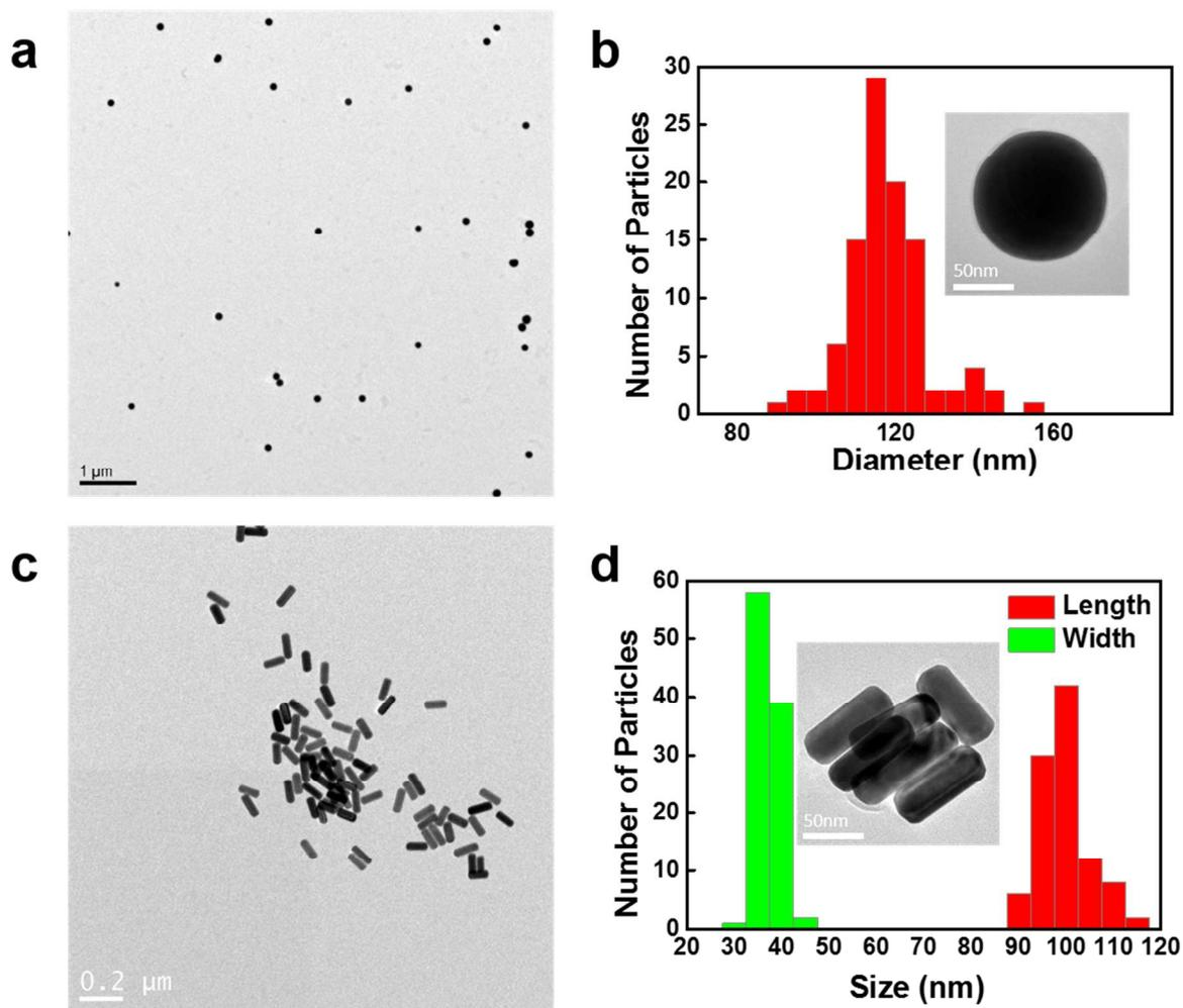
Figure S1. The transmission electron microscope images for (a) gold NSs with (b) 110 nm diameter distribution and (c) gold NRs with (d) 100 nm in length and 40 nm in width distribution.
