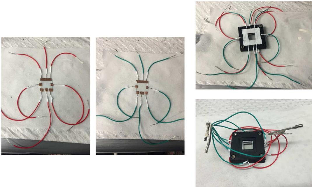
Figure S4. Digital images of assemble method and 3D printed large scale EPD cell with 20 mm (L)  $\times$  20 mm (W)  $\times$  2 mm (H) tank.
