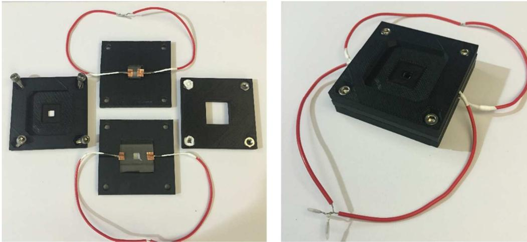
Figure S3. Digital images of assembly method and 3D printed, small-scale EPD cell with 10 mm (L)  $\times$  10 mm (W)  $\times$  2 mm (H) tank. Before and after assembly.
