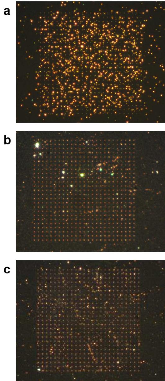
Figure S7: Gold nanorod EPD assembly under different electrolyte concentration and applied potential to demonstrate the influence of electric field overlapping near the electrode surface. EPD condition (Potential, NaCl concentration) **(a)**: 3V, 0 mM. **(b)**: 3V, 0.2 mM. **(c)**:4V, 0.2 mM.
