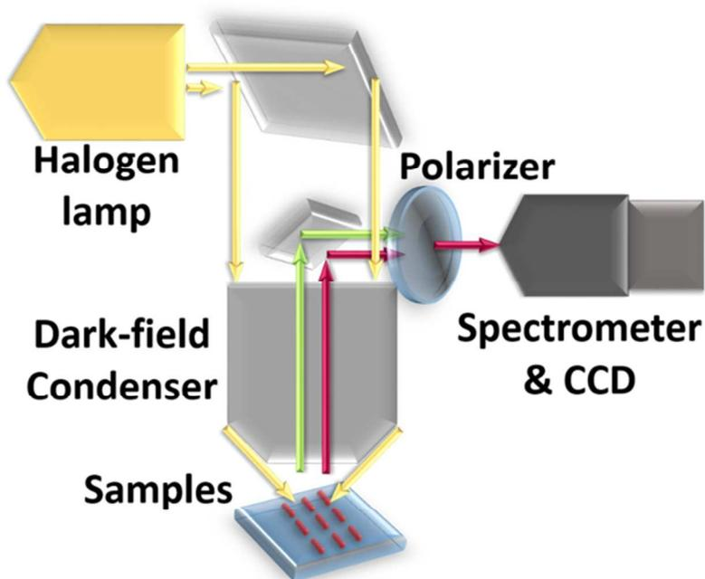
Figure S8: Schematic of reflectance dark-field microscope with polarizer.
