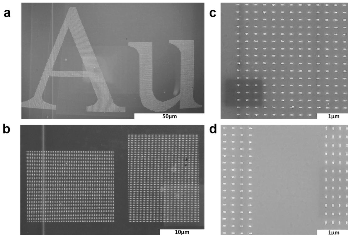
Figure S9: The scanning electron microscope image of (a) Letter “Au” assembled with gold NRs with perpendicular orientation and (b) corresponding rectangular array with same array structure. High magnification scanning electron microscope image of (c) the corner and (d) between rectangular arrays.
