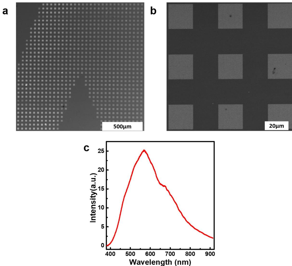
Figure S12 Scanning electron microscopy images of “Au” logo filled by gold NRs *via* EPD assembly. (a) Top part of the “Au” logo of the letter “A”. (b) 9 of the Pixels in “Au” logo filled by gold NRs. (c) Dark-field microscopy scattering spectrum of one pixel in “Au” logo.
