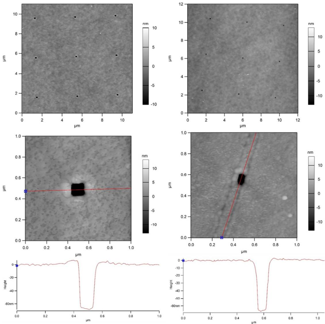
Figure S2. The atomic force microscopy images for box array (Left) and rod array (Right) and the height profile which shows 60 nm PMMA thickness.
