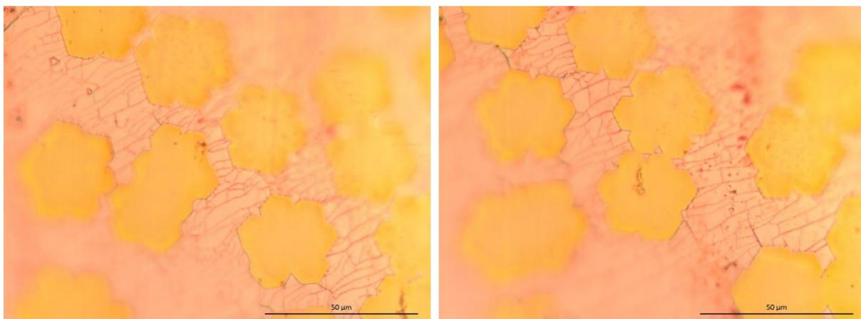
**Figure S1.** The OM images of hexagon flower-etched patterns on large-scale graphene located on liquid Cu/W foil.
