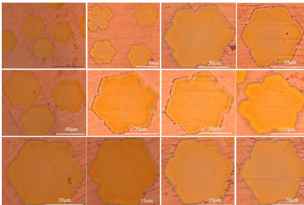
**Figure S2.** The OM images of hexagon flower-etched patterns on large-scale graphene located on liquid Cu/W foil at different magnifications.
