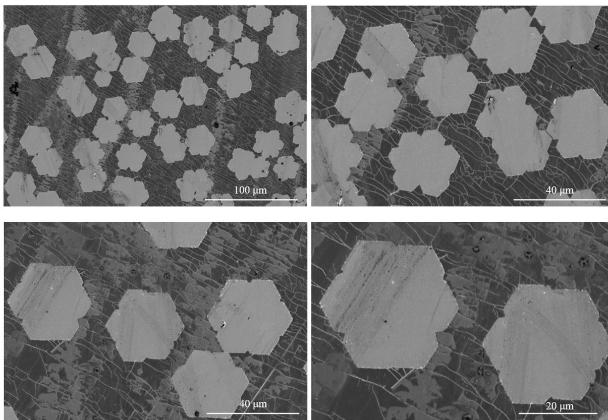
**Figure S4.** The SEM images of hexagon flower-etched patterns on large-scale graphene located on liquid Cu/W foil at different magnifications.
