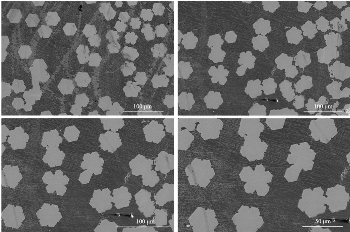
**Figure S3.** The SEM images of hexagon flower-etched patterns on large-scale graphene located on liquid Cu/W foil at different magnifications.
