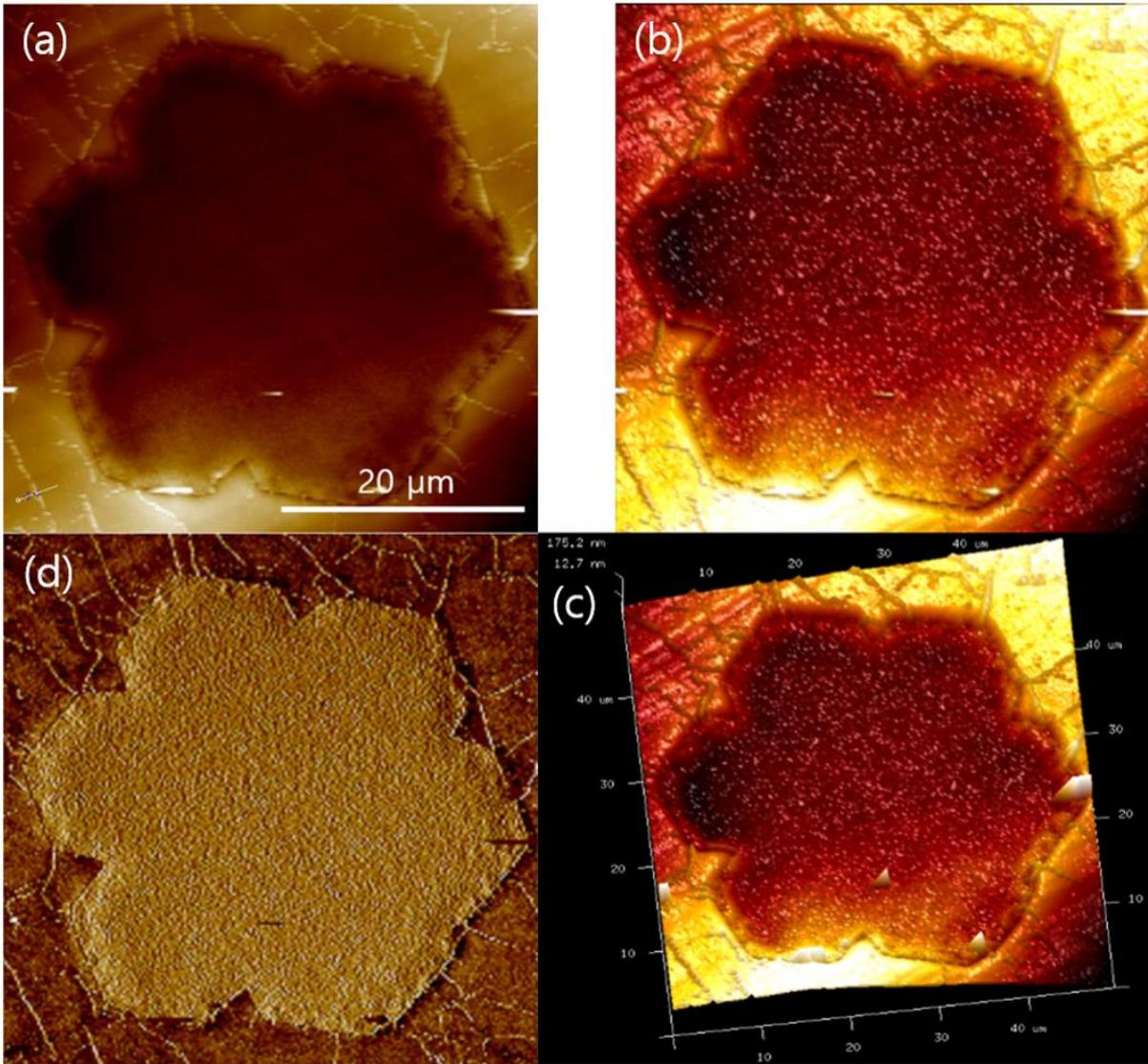
**Figure S5.** The AFM images of hexagon flower-etched patterns on large-scale graphene located on liquid Cu/W foil (a), (b) the 3D AFM mapping image of (a), the 3D AFM mapping image at different view of (a), and (d) the phase image of (a).
