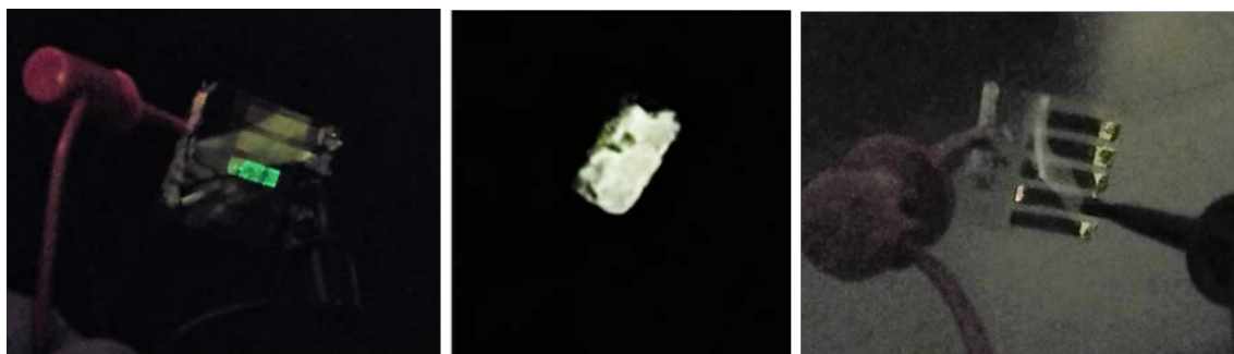
Figure S10: \text{CsPbBr}_3 and \text{CsPbX}_3 mixed halide film-based LEDs displaying characteristic green and white light emission. Left panel: LED based on \text{CsPbBr}_3 nanocrystals. Middle and Right panels: white light emission from \text{CsPbX}_3 LED.
