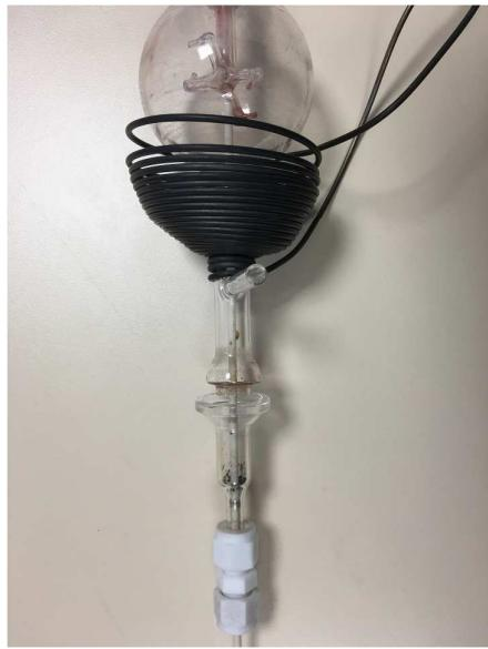
*Fig. SI2 - Thermocouple located inside the Nancy reactor.*
