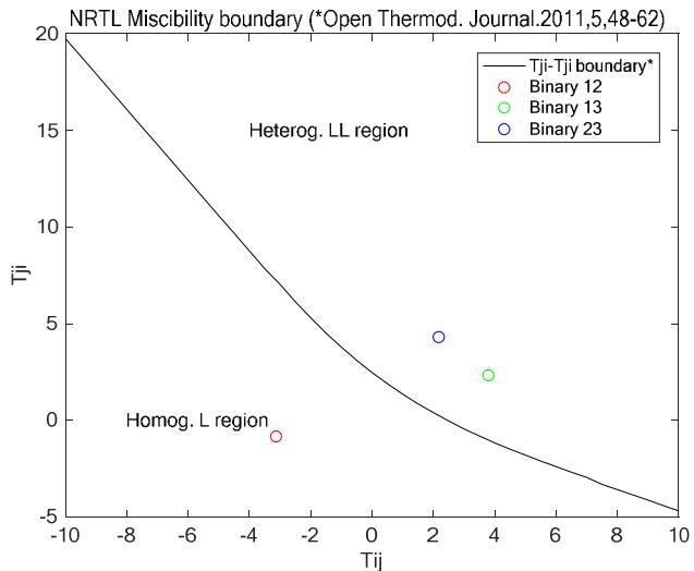
**Figure S8.** NRTL binary parameter boundary for total and partial miscibility for the ternary system {methyl isobutyl ketone (1) + isoquinoline (2) + water (3)} at 298.15 K.
