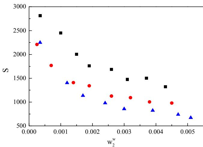
**Figure S4.** Separation factors plotted versus mass fraction of isoquinoline in the aqueous phase at different temperatures. (■)  $T = 298.15\text{ K}$ , (●)  $T = 318.15\text{ K}$ , (▲)  $T = 338.15\text{ K}$ .
