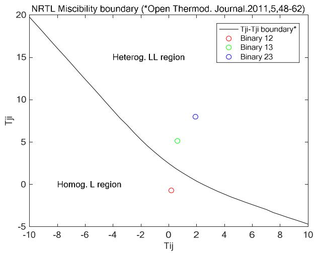
**Figure S7.** NRTL binary parameter boundary for total and partial miscibility for the ternary system {methyl isobutyl ketone (1) + quinoline (2) + water (3)} at 298.15 K.
