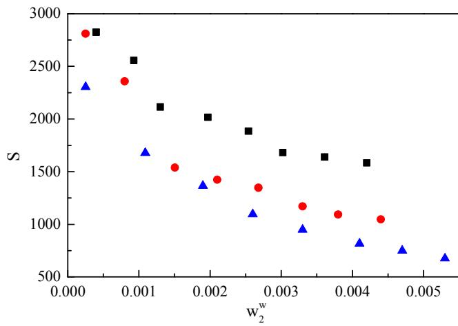
**Figure S3.** Separation factors plotted versus mass fraction of quinoline in the aqueous phase at different temperatures. (■)  $T = 298.15\text{ K}$ , (●)  $T = 318.15\text{ K}$ , (▲)  $T = 338.15\text{ K}$ .
