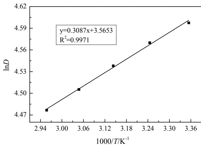
**Figure S6.**  $\ln D$  plotted versus  $1000/T/K^{-1}$  in isoquinoline extraction.
