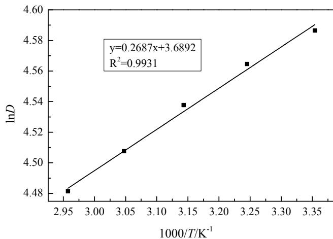
**Figure S5.**  $\ln D$  plotted versus  $1000/T/K^{-1}$  in quinoline extraction.
