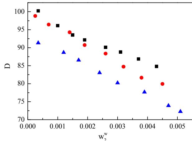
**Figure S2.** Distribution coefficients plotted versus mass fraction of isoquinoline in the aqueous phase at different temperatures. (■)  $T = 298.15\text{ K}$ , (●)  $T = 318.15\text{ K}$ , (▲)  $T = 338.15\text{ K}$ .
