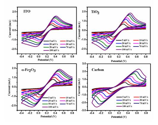
**Figure S3** Determination of the EASA using CVs conducted in 0.1 M KNO<sub>3</sub> containing 0.1 M K<sub>4</sub>Fe(CN)<sub>6</sub> at different scan rates of 5, 10, 20, 30, 50, 70, 100 mV/s
