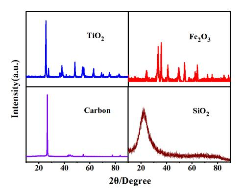
Figure S1 XRD patterns of NPs on the surface of ITO electrodes. The XRD were recorded on an Empyrean diffractometer at room temperature, operating at 40 kV and 40 mA, using a Cu K $\alpha$  radiation ( $\lambda = 0.15418$  nm).
