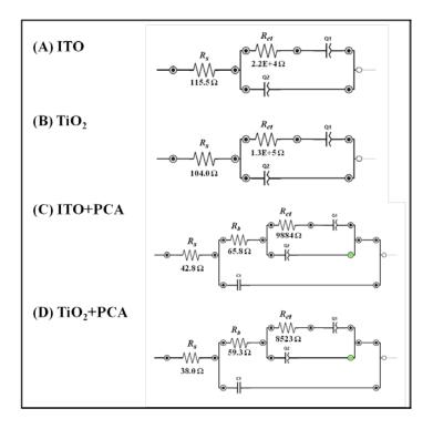
**Figure S2** The equivalent circuits used for fitting the EIS spectra for bare ITO (A) bare TiO<sub>2</sub> NPs-coated ITO (B), biofilm-attached ITO (C), and biofilm-attached TiO<sub>2</sub>-coated ITO (D), where the element  $R_s$  represents solution resistance (ohmic resistance),  $R_{ct}$  represents the activation (charge transfer) resistance, and  $R_b$  represents the biofilm resistance. The values obtained by fitting the EIS spectra were shown below each element.
