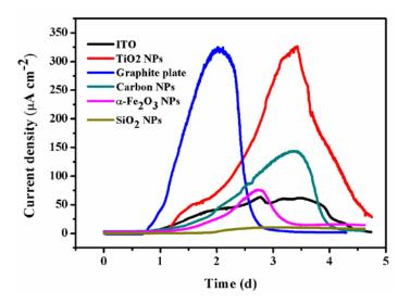
**Figure S4** Amperometric i-t curves for strain PCA grown on graphite plate and on ITO electrode coated with different NPs. The current densities produced were calculated normalized with the anode areas (Table S1).
