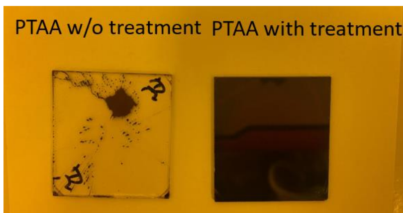
Supplementary Figure S10. Perovskite films deposited on PTAA with and without plasma treatment.
