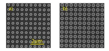
**Figure S8.** Top view SEM images of the fabricated Si nanodisk arrays with various diameters.
