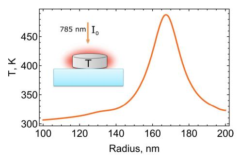
**Figure S5**: Laser-induced heating of Si nanodisks. Estimation of the stationary temperature of a Si nanodisk of 70 nm height on a glass substrate illuminated by a CW 785 nm laser of 10.85 mW power focused on the area of 1  $\mu$ m x 1  $\mu$ m, corresponding to the experimental conditions for anti-Stokes measurements.
