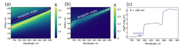
**Figure S2**: Linear properties of the anapole state. (a) Map of simulated reflection spectra from the Si nanodisks array. (b) The same map for absorption spectra. (c) The phase difference between the electric and toroidal dipole moments induced in a nanodisk inside the array extracted from the multipole decomposition.
