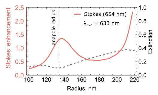
**Figure S7**. Theoretical analysis of Raman scattering for 633 nm excitation. Solid curve: intensity of the Stokes emission vs disk radius at the excitation wavelength of 633 nm normalized by Stokes emission from an un-patterned film of the same thickness. Dashed curve: extinction of the array vs nanodisk radius at the same excitation wavelength.
