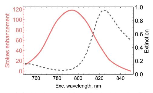
**Figure S4.** Simulated dependence of extinction and intensity of the Stokes emission on the excitation wavelength for a 180 nm radius nanodisk array normalized by Stokes emission from an unpatterned 70 nm height film.
