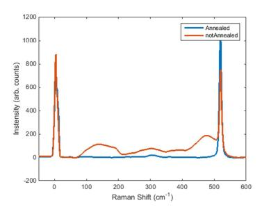
**Figure S6**. Raman spectrum for an amorphous Si film deposited at 625 °C (red line) and of a poly-Si film obtained after high temperature annealing (blue line). In the second case, only a peak at 521 cm<sup>-1</sup> from crystalline Si is clearly visible, while signals at shorter Raman shift produced by amorphous silicon is essentially absent. This result confirms the high quality of the film.
