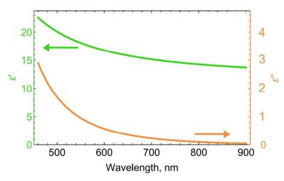
Figure S1: Poly-Si dielectric function obtained using spectroscopic ellipsometry.
