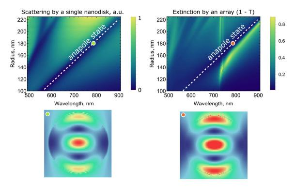
**Figure S3.** Comparison of the simulated anapole state dispersion in an isolated Si nanodisk and in the periodic array. Pictures at the bottom present electric field intensity in the horizontal plane at the center of the disk under plane wave illumination at the anapole wavelength.
