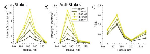
**Figure S9**. Laser intensity dependent Raman signal. Integrated 521 cm<sup>-1</sup> Stokes (a) and anti-Stokes (b) Raman scattering intensity from arrays of silicon nanodisks of various radii for 785 nm excitation. Results for different powers show increase in the signal. (c) Intensity ratio between anti-Stokes and Stokes signals versus radius and laser power. The similar curve shapes for different powers indicate only a weak dependence on temperature.
