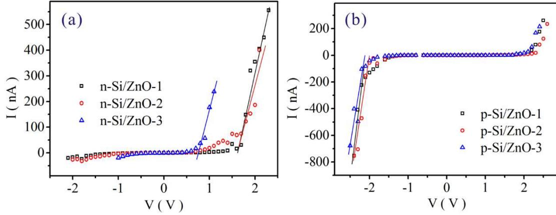
Figure S1. Experimental data of the electric conductance I-V curves for the individual (a) n-Si/ZnO and (b) p-Si/ZnO nano-emitters. (Reproduced from the insets of Figure 4 (a) and (b) in Ref [1].) The straight lines are the linear fitting curves in the high voltage regions.
