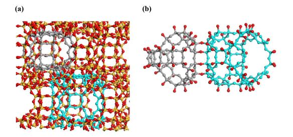
**Fig.S1.** (a) EMT-type zeolite framework with hypocage highlighted in silver and hypercage in cyan. (b) A detailed view on hypocage (in silver), connected to the hypercage (in cyan).
