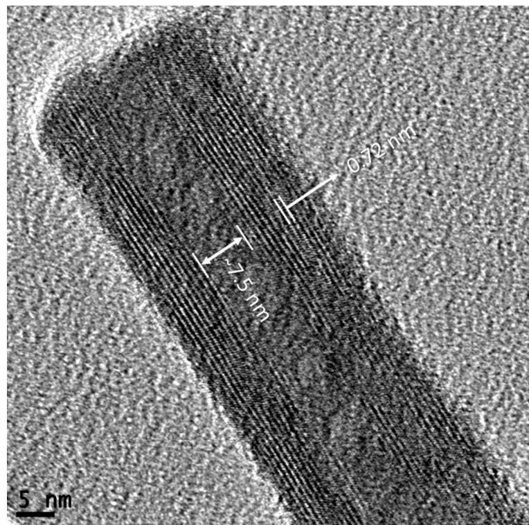
**Figure S3.** HR-TEM image of a BNKT2 nanotube with an inner diameter and interplanar distance of 7.5 nm and 0.72 nm, respectively.
