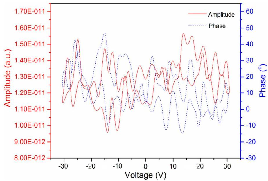
**Figure S5.** The amplitude and phase graphs of Si substrate as reference.
