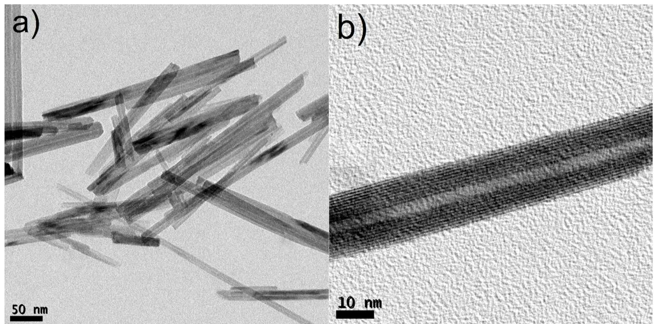
**Figure S2.** Bright field TEM image of a) a bunch of BNKT3 nanotubes and b) a single BNKT3 nanotube.
