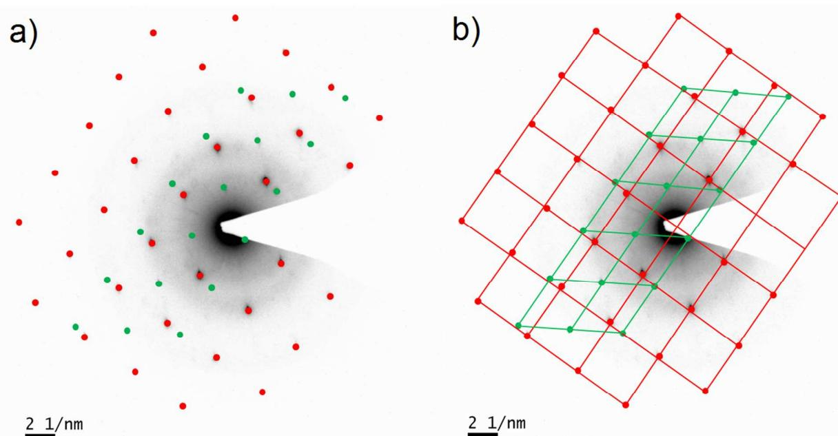
**Figure S4.** a) Inverted colour SAED map and, b) orthorhombic (green) and tetragonal (red) patterns of a BNKT2 nanotube.
