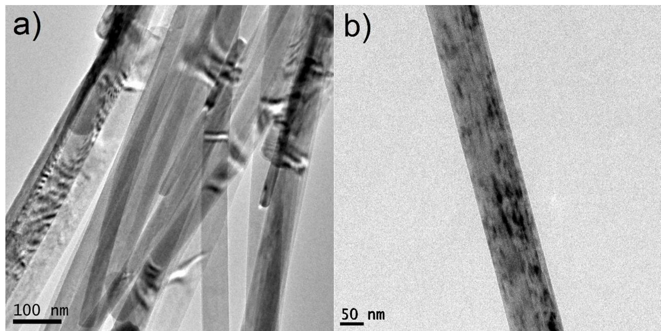
**Figure S1.** Bright field TEM images of a) a bunch of BNKT1 nanofibers and b) a single BNKT1 nanofiber.
