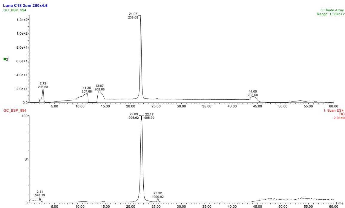
Figure S11. LC/MS Chromatogram of isolated Microcystin-LR.
