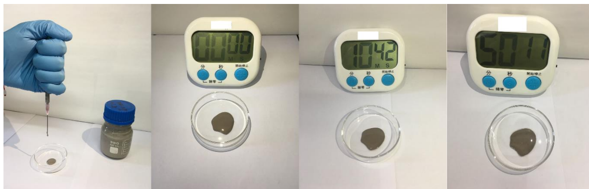
Figure S1. Sodium dispersions in oil (particle size 5-10 \mu\text{m} ) was transferred into a glassware via syringe and kept in an open atmosphere for 50 min.
