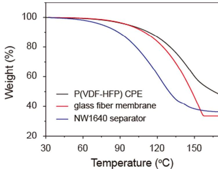
**Figure S3.** The comparison of TGA curves of the P(VDF-HFP) CPE with the glass fiber membrane and commercial separator NW1640 (Cangzhou Mingzhu Lithium Battery Separator co., ltd) after absorbing the organic electrolyte at the same amount as that in P(VDF-HFP) CPE.
