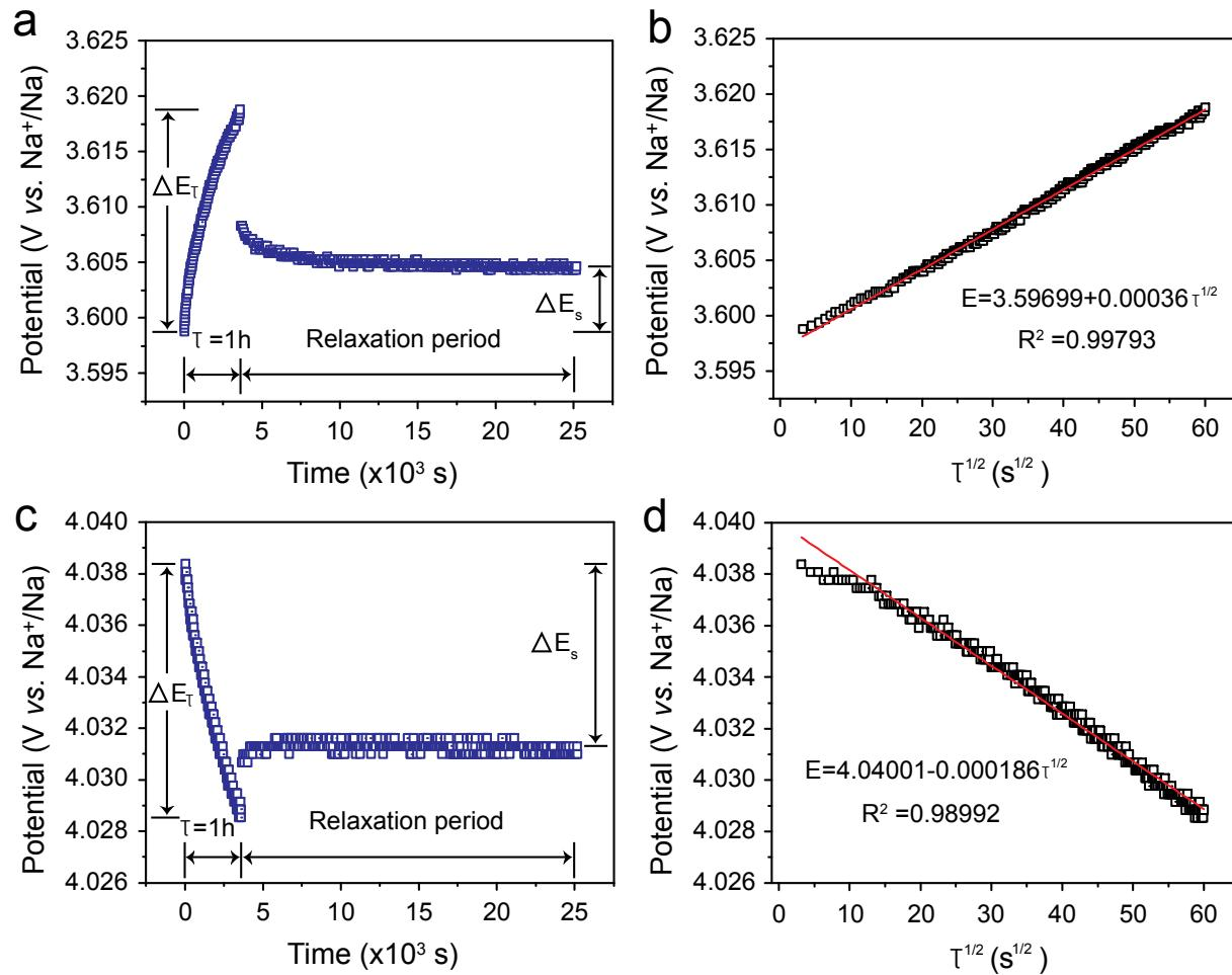
**Figure S8.** A single GITT profile for charge and discharge process.  $\tau$  vs.  $E$  profiles for a single GITT titration during (a) charge and (c) discharge processes. The corresponding linearly fitting behavior of  $E$  vs.  $\tau^{1/2}$  for the (b) charge and (d) discharge GITT titration.
