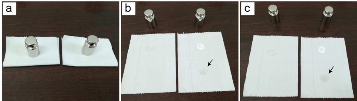
**Figure S1.** The ability to retain electrolyte of the P(VDF-HFP) CPE compared with the glass fiber membrane. (a) optical photograph under the 100 g pressure, (b) after 1 min, and (c) after 5 min.
