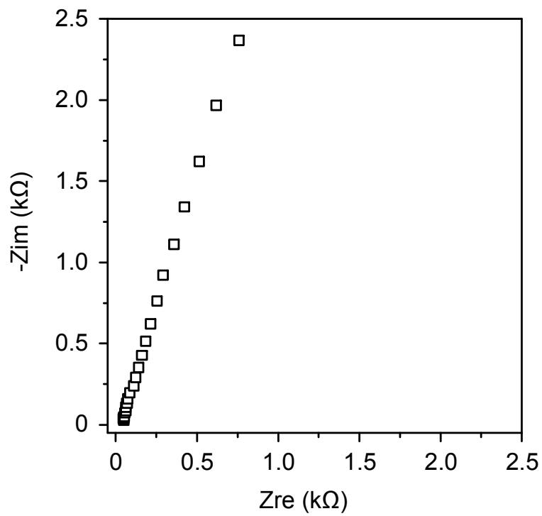
**Figure S2.** EIS measurement of the P(VDF-HFP) GPE at room temperature.
