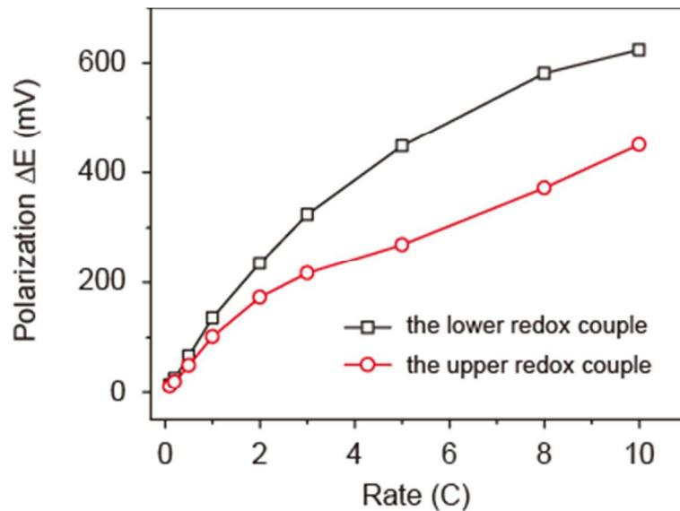
**Figure S6.** The variations of polarization values ( $\Delta E$ ) of the upper/lower redox couples for the NVPOF cathode along with C rates.
