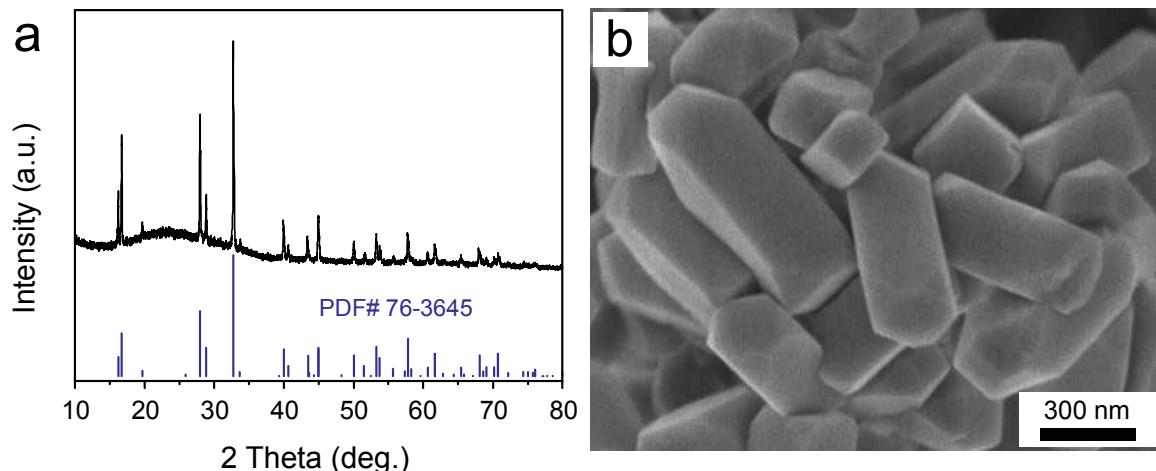
**Figure S4.** (a) XRD pattern, and (b) SEM image of the NVPOF cathode materials.
