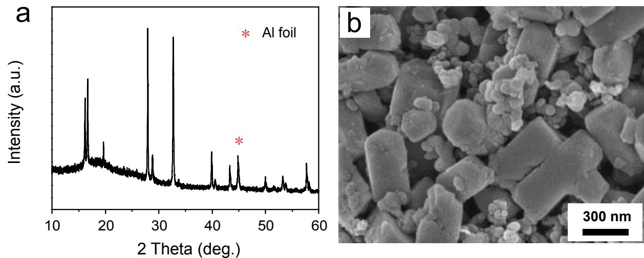
**Figure S7.** (a) XRD pattern and (b) SEM image of the NVPOF cathode after 50 cycles at 1 C.
