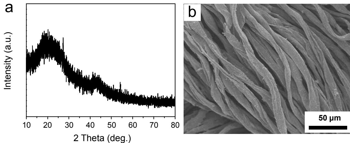
**Figure S5.** (a) XRD pattern, and (b) SEM image of the CC anode materials.
