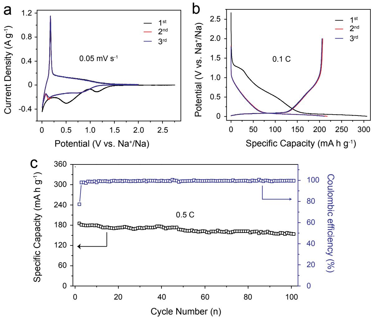
**Figure S9.** The Na-storage properties of CC anodes: (a) CV patterns of the initial 3 cycles, (b) GCD curves of the initial 3 cycles, and (c) cycling performance at 0.5 C.
