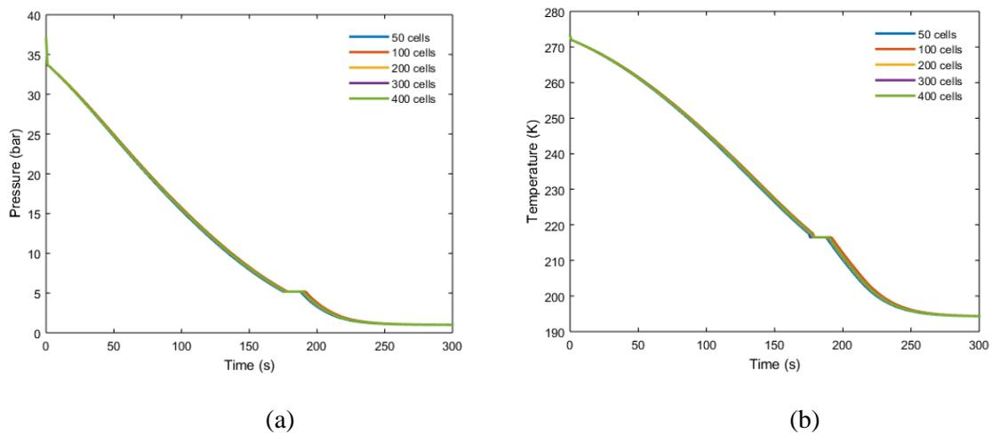
Figure A1. The histories of pressure (a) and temperature (b) variation at the second measurement point (Figure 2) in Test 1, predicted using 50, 100, 200, 300 and 400 computational cells.
