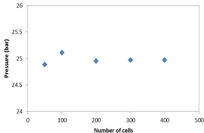
Figure A2. The impact of the number of cells on the pressure computed at the second measurement point (Figure 2) in Test 1 at 50 s.
