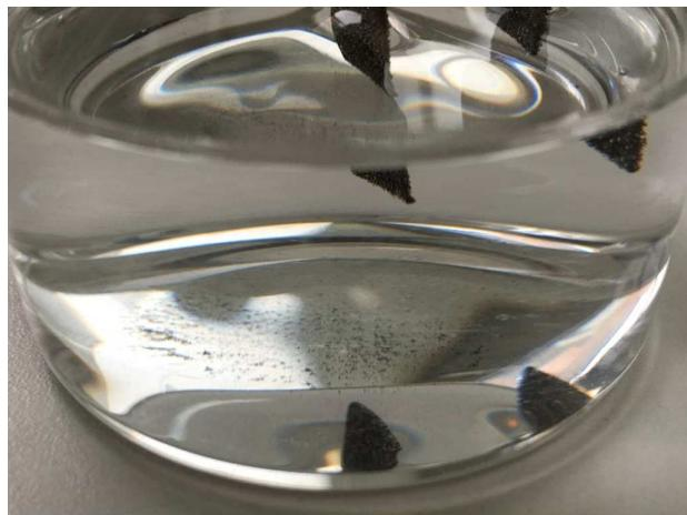
**Figure S24** Photograph of electrolytic cell after durability testing for  $\text{Pt/C}||\text{IrO}_x$  couple. The black powder at the bottom may be the catalyst peeled off from the NF substrate caused by the impact of generated gas bubbles.
