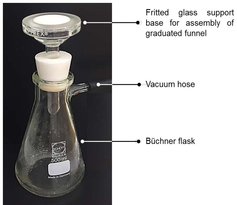
**Figure S1.** Photograph of the selective filtration system for the ultrasensitive detection of *E. coli* O157:H7.
