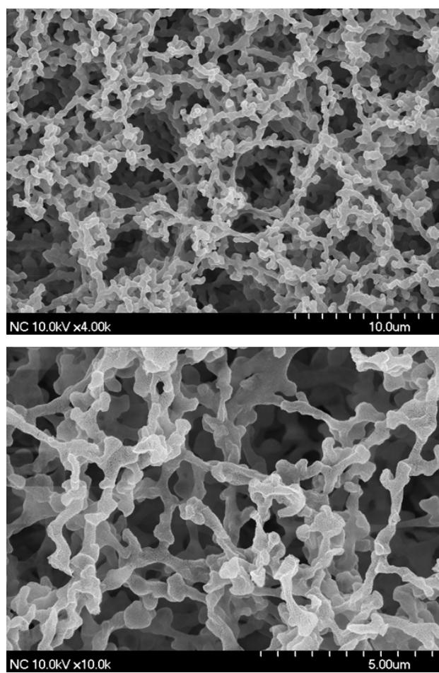
**Figure S2.** Scanning electron microscopy images of nitrocellulose membrane filters with a pore size of 1.2  $\mu\text{m}$ .
