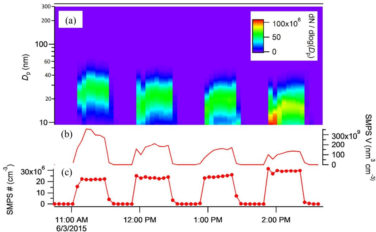
**Figure S11.** Results from four consecutive forced regenerations of the DPF on the 2007 HDDV. SMPS results are presented as (a) number size distributions, (b) total volume concentration, and (c) total number concentration.
