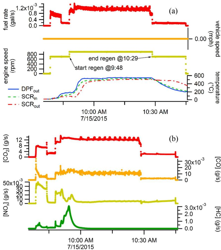
**Figure S6.** (a) Engine parameters and (b) emissions from a parked regeneration of the DPF from the 2010 HDDV performed on July 15, 2015.
