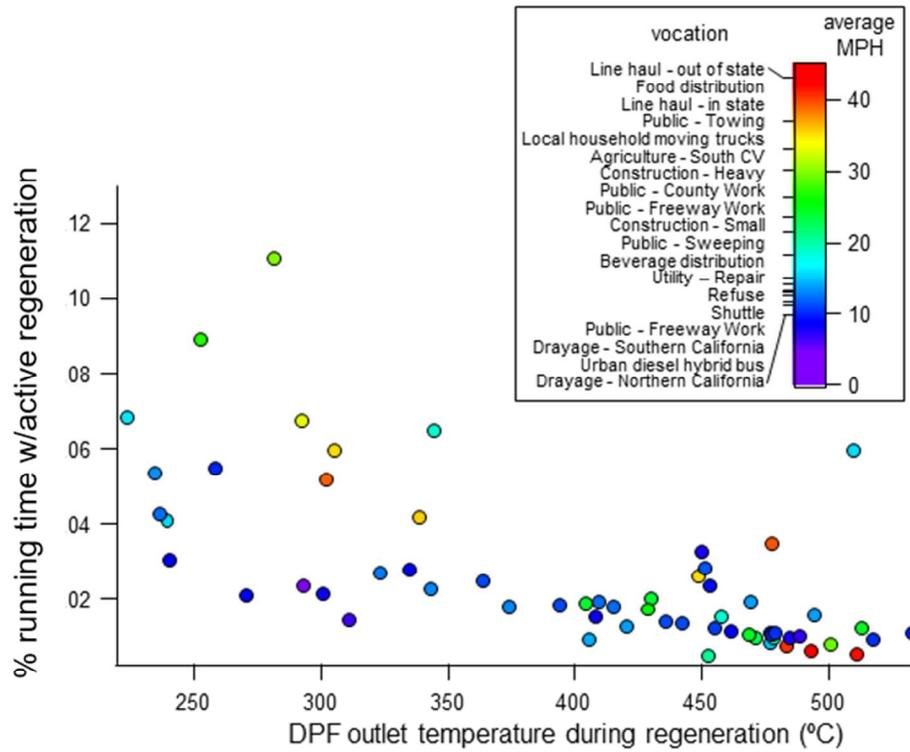
**Figure S13.** Percent of engine-on time in which active DPF regeneration was occurring vs. average DPF outlet temperature during regeneration.
