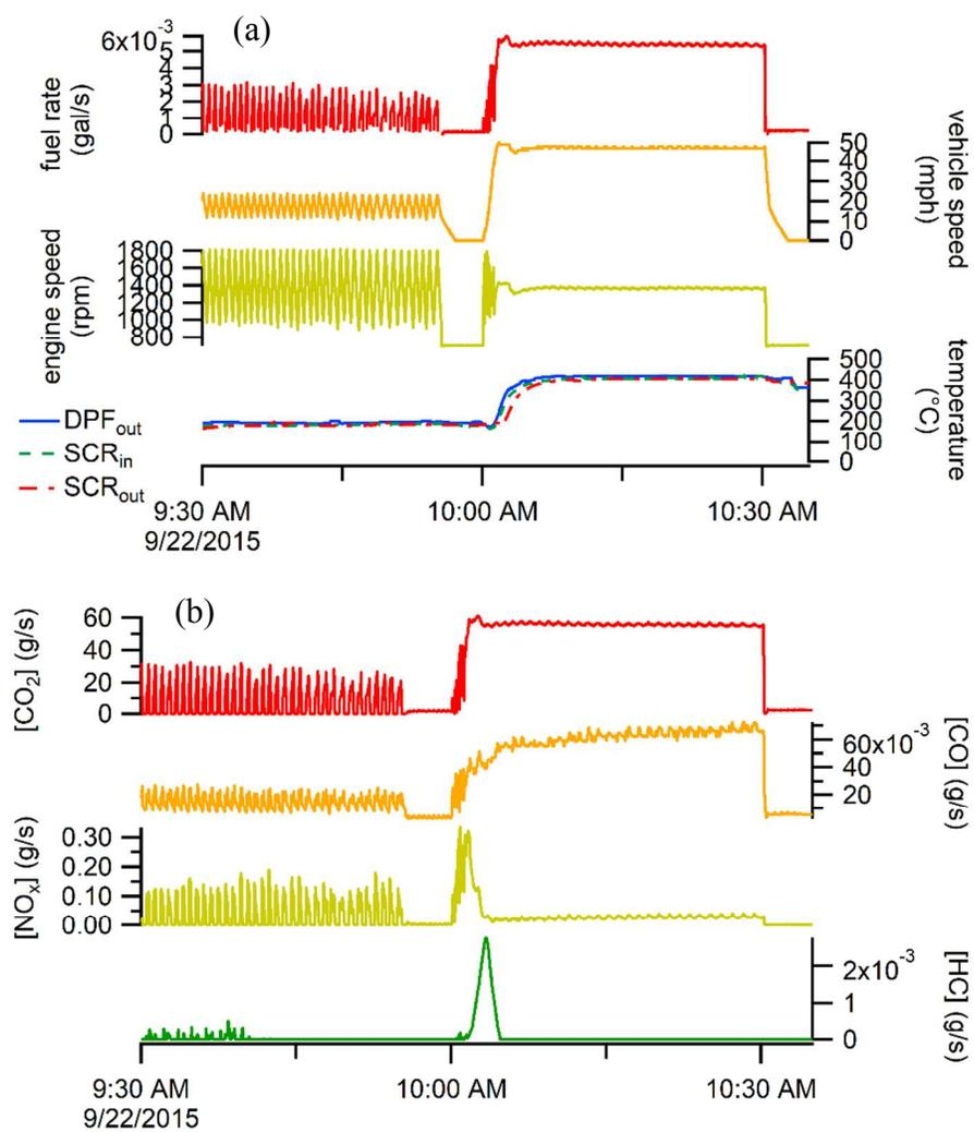
**Figure S9.** (a) Engine parameters and (b) emissions from a passive regeneration of the DPF from the 2010 HDDV performed on September 22, 2015.
