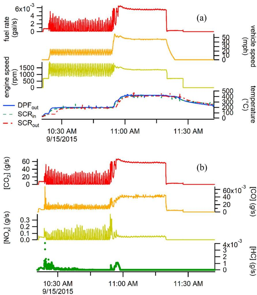
**Figure S7.** (a) Engine parameters and (b) emissions from a passive regeneration of the DPF from the 2010 HDDV performed on September 15, 2015.
