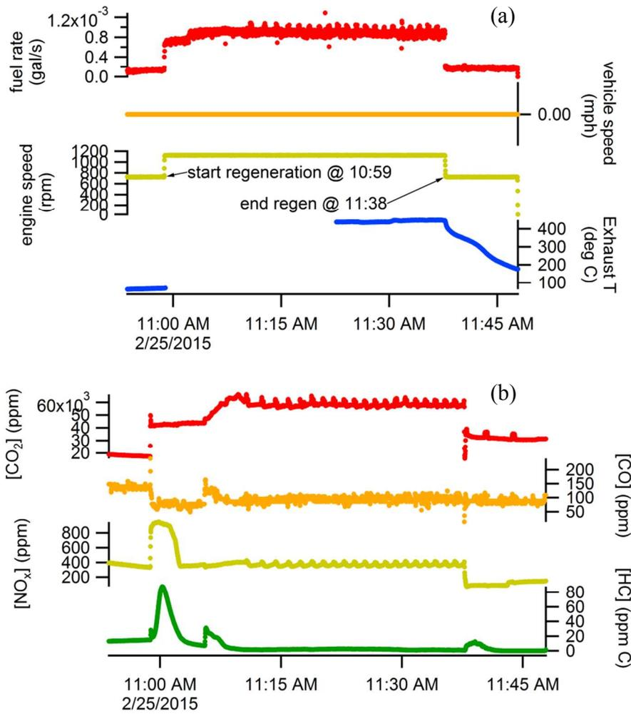
**Figure S2.** (a) Engine parameters and (b) emissions from a parked regeneration of the DPF from the 2007 HDDV performed on February 25, 2015.
