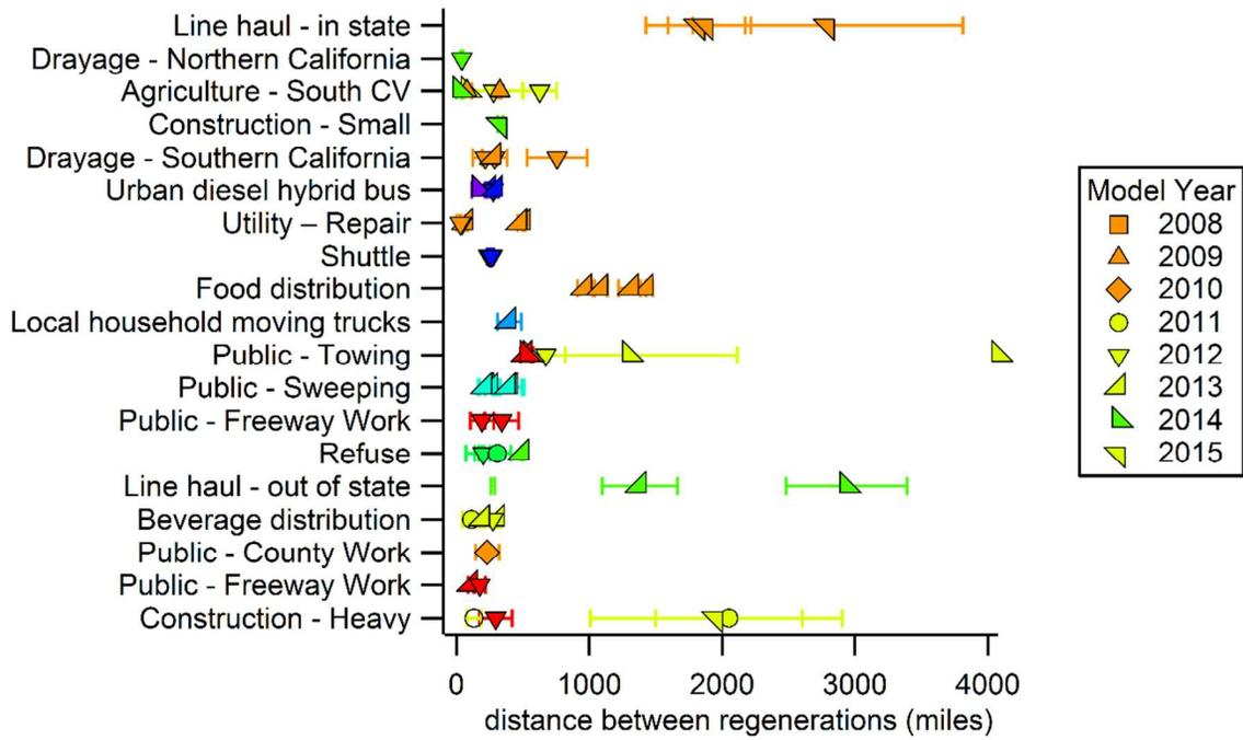
**Figure S15.** Average distance travelled between DPF regenerations, by HDDV vocation, model year (symbol), and OEM (color).
