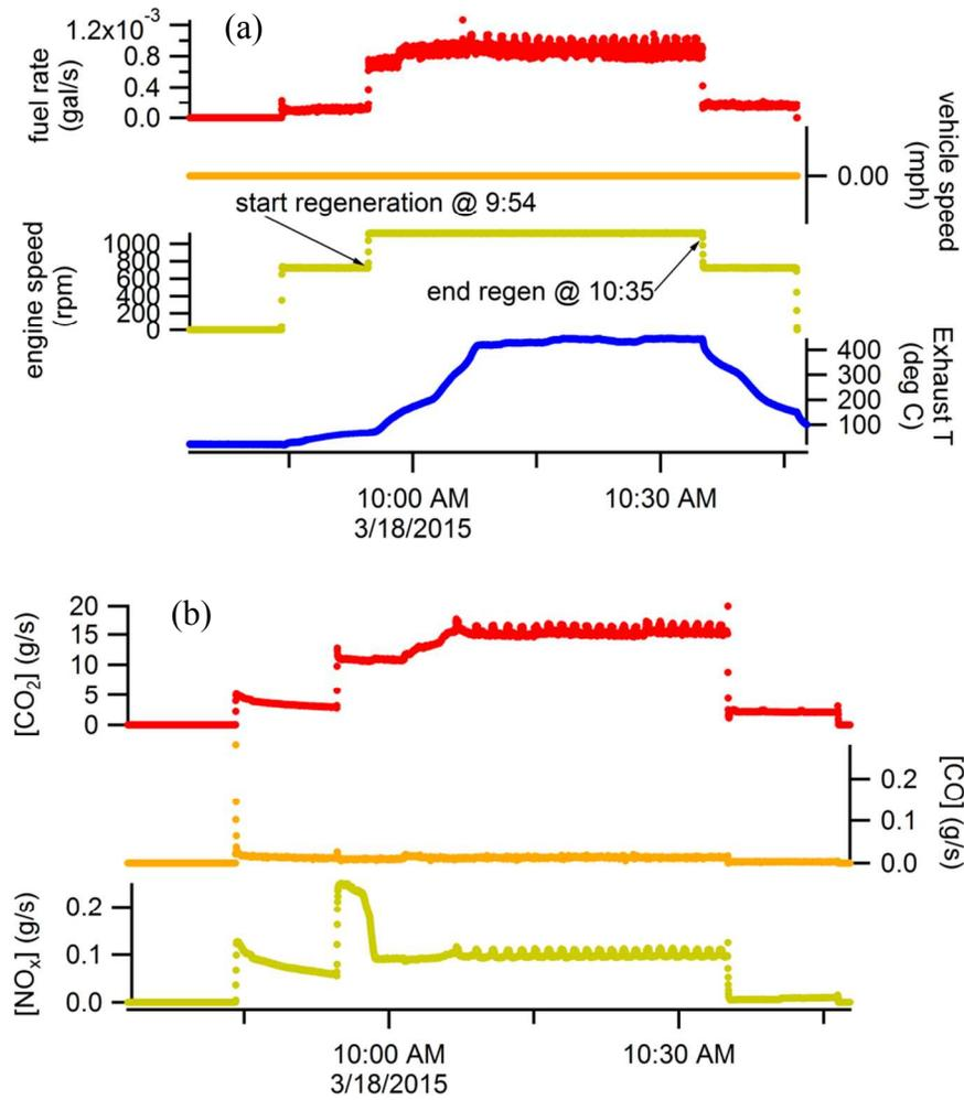
**Figure S3.** (a) Engine parameters and (b) emissions from a parked regeneration of the DPF from the 2007 HDDV performed on March 18, 2015.
