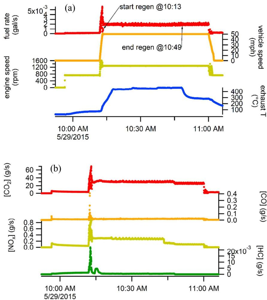
**Figure S5.** (a) Engine parameters and (b) emissions from a driving regeneration of the DPF from the 2007 HDDV performed on May 29, 2015.
