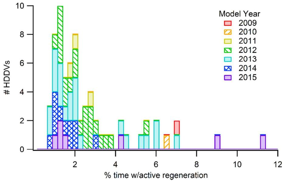
**Figure S12.** Histogram of the percentage of total running time that real-world vocational HDDVs underwent active DPF regeneration.
