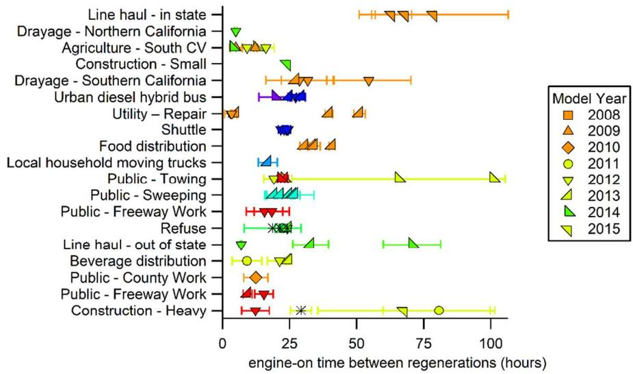
**Figure S14.** Average engine-on time between DPF regenerations, by HDDV vocation, model year (symbol), and OEM (color).
