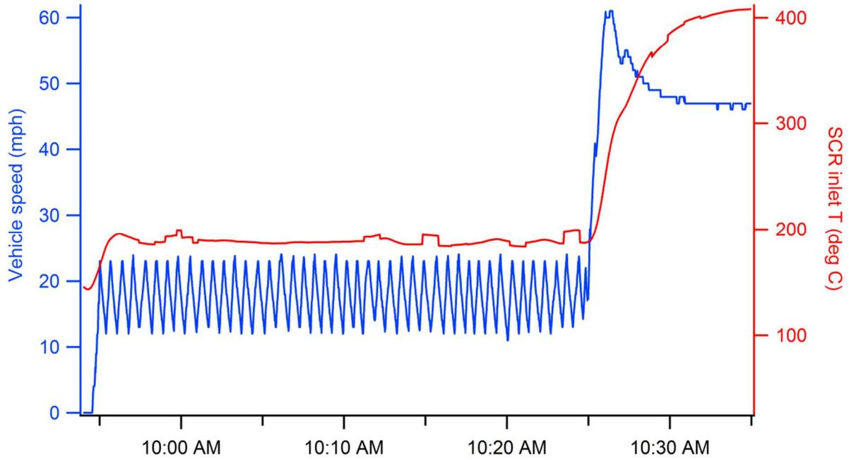
**Figure S1.** Typical pattern of acceleration/deceleration used to load HDDV DPFs with PM (through 10:25 AM), followed by an acceleration to highway speeds and associated increase in SCR inlet temperature.
