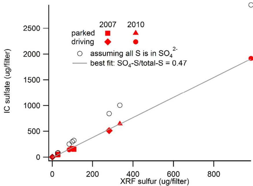
**Figure S10.** Sulfur detected by IC (as sulfate) vs detected by XRF.
