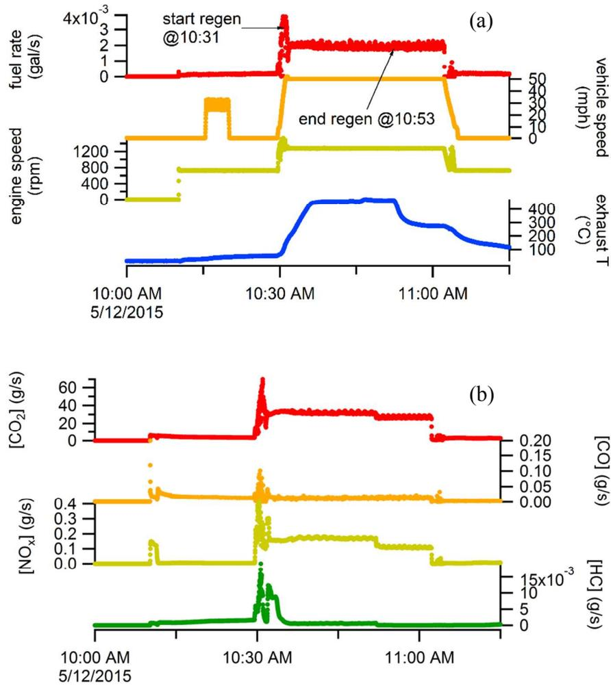
**Figure S4.** (a) Engine parameters and (b) emissions from a driving regeneration of the DPF from the 2007 HDDV performed on May 12, 2015.
