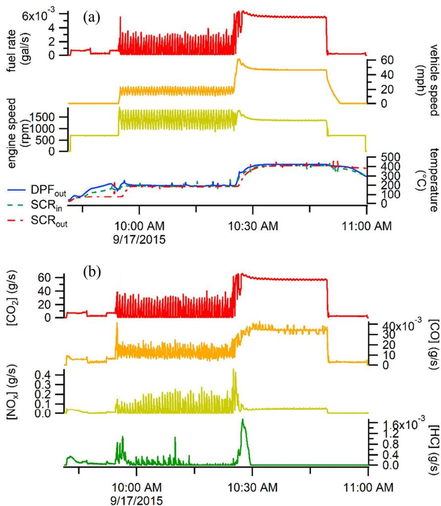
**Figure S8.** (a) Engine parameters and (b) emissions from a passive regeneration of the DPF from the 2010 HDDV performed on September 17, 2015.
