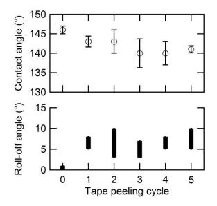
**Figure S2.** Variation of the water contact angle (top) and roll-off angle (bottom) as a function of the number of adhesive tape peeling cycles performed on a superhydrophobic fabric coated with PDMS(1.5 wt%)/silica particles(1 wt%)/PDMS(1.5 wt%).
