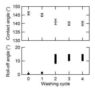
**Figure S3.** Variation of the water contact angle (top) and roll-off angle (bottom) versus the number of machine washing cycles, measured for PDMS(1.5 wt%)/silica particle(1 wt%)/PDMS(1.5 wt%) coating, for which the external PDMS layer was further cross-linked with the addition of Phobol XAN.
