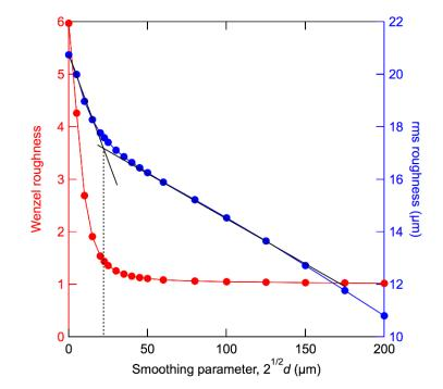
Figure S1. Variation of the rms roughness (blue, right axis) and of the Wenzel roughness (red, left axis) versus the degree of smoothing of the profilometry image of the fabric. The optimal smoothing parameter is found at the intersection between the two linear regimes of variation of the rms roughness, as indicated in the Figure. d is the standard deviation of the Gaussian low pass filter used for smoothing.
