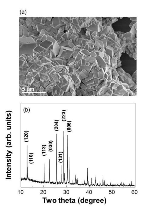
Figure S5. (a) SEM image and (b) XRD pattern of CsPbBr<sub>3</sub> QDs.
