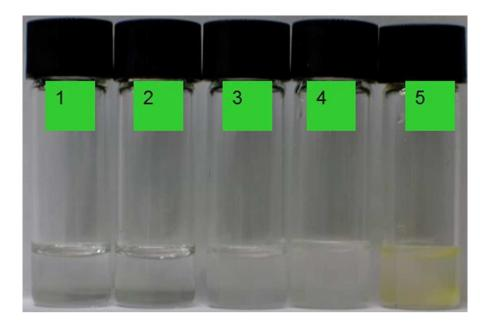
**Figure S2**. Photographs showing the formation of CsPbBr<sub>3</sub> MCs in HBr and its transformation to Cs<sub>4</sub>PbBr<sub>6</sub> MCs on adding DMSO.
