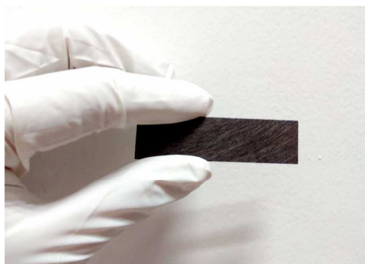
Figure S2: The photo shows a HER electrode (1.5 cm x 6 cm) with CoP loaded on carbon fiber paper, suggesting large-scale fabrication is possible.
