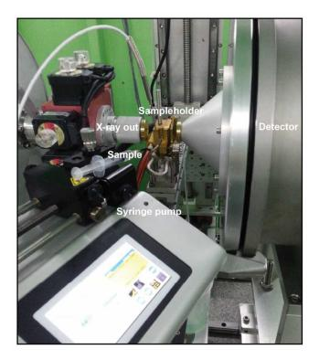
**Figure S1. Flow cell system for SAXS measurement at Pohang Light Source.** The sample is continuously injected using the syringe pump. The X-ray scattering pattern was measured using a quartz capillary in the flow cell available in the beamline.
