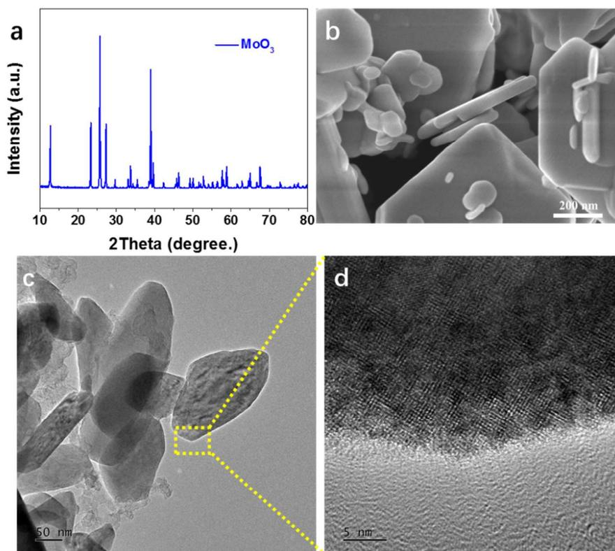
**Figure S2.** Characterization of blue MoO<sub>3</sub>. XRD pattern (a), SEM image (b), TEM and corresponding HRTEM images of the blue MoO<sub>3</sub> nanosheets.
