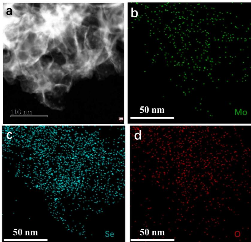
**Figure S5.** The dark-field TEM images (a) and corresponding element mapping images (b-d) of the prepared red MoSe<sub>2</sub> nanosheets (corresponding to area 3 in Figure 2f), suggesting the homogeneous distribution of Mo, O and Se.
