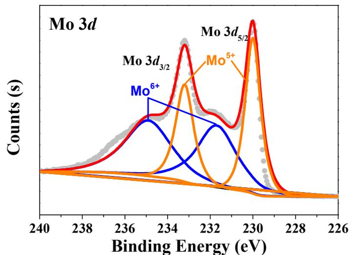
**Figure S9.** High-resolution XPS spectra of Mo 3d of the blue MoO<sub>3</sub> nanosheets.
