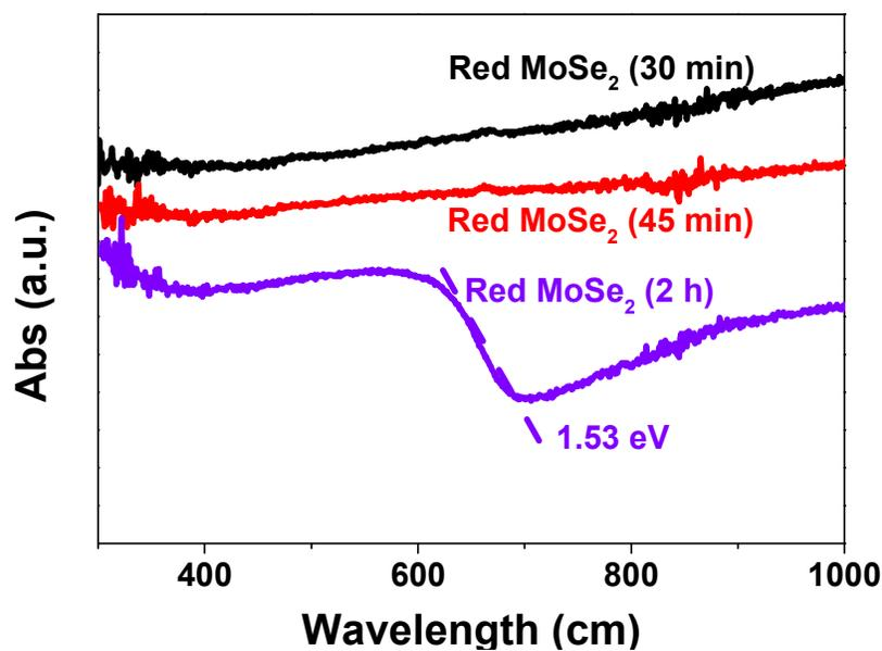
**Figure S1.** UV–visible absorption spectra showing the different absorption between the prepared series red MoSe<sub>2</sub> samples.
