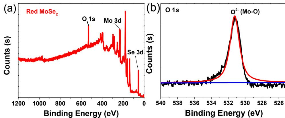
**Figure S8.** The overall (a) and high resolution O1s XPS spectra (b) of the prepared red MoSe<sub>2</sub> nanosheets.
