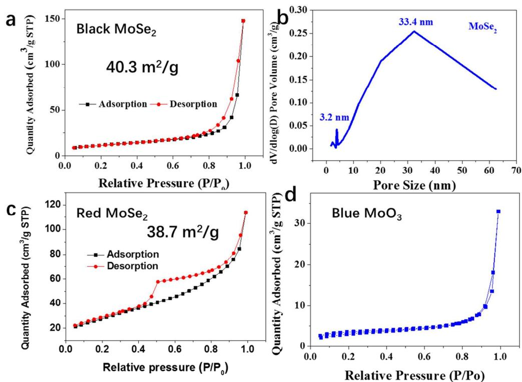
**Figure S10** Nitrogen adsorption-desorption isotherms of the prepared black MoSe<sub>2</sub> (a), red MoSe<sub>2</sub> (c) and blue MoO<sub>3</sub> (d). Corresponding pore size distributions of the prepared black MoSe<sub>2</sub> (b).
