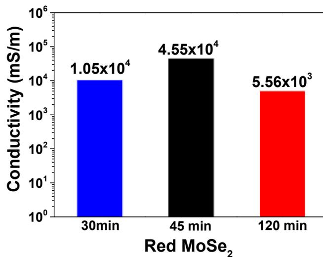
Figure S7. The electronic conductivity of the prepared series red  $\text{MoSe}_2$  samples.
