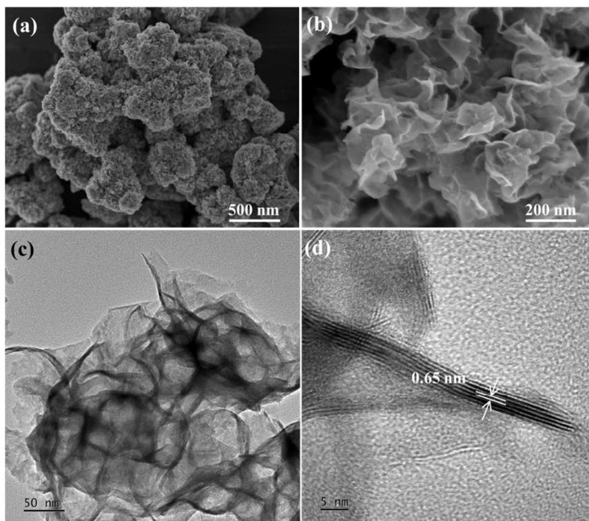
**Figure S3.** SEM (a) and corresponding enlarged SEM (b) images of the prepared MoSe<sub>2</sub> nanosheets. TEM (c) and HRTEM (d) images of the MoSe<sub>2</sub> NSs, displaying a uniform d spacing of 0.65 nm for the (002) plane in the MoSe<sub>2</sub> NSs.
