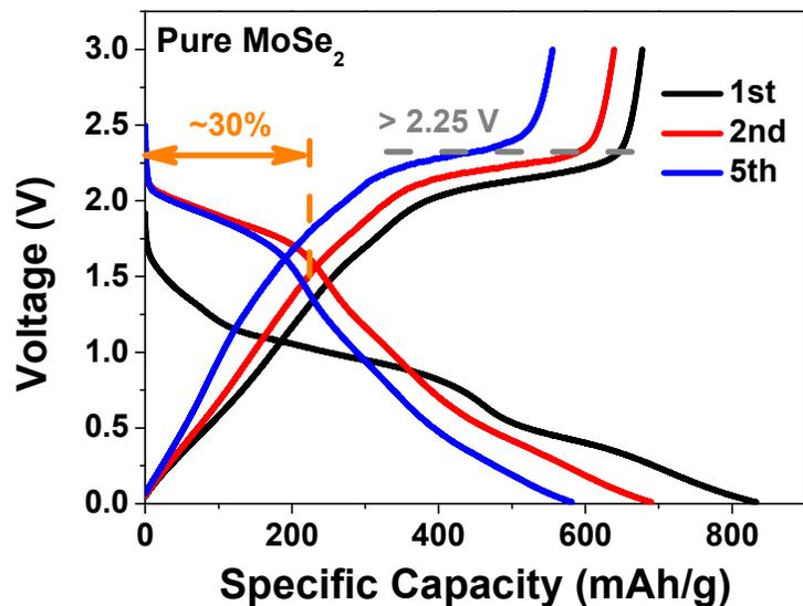
Figure S11. Discharge-charge voltage profiles of prepared black MoSe<sub>2</sub> anode in the initial 5 cycles.
