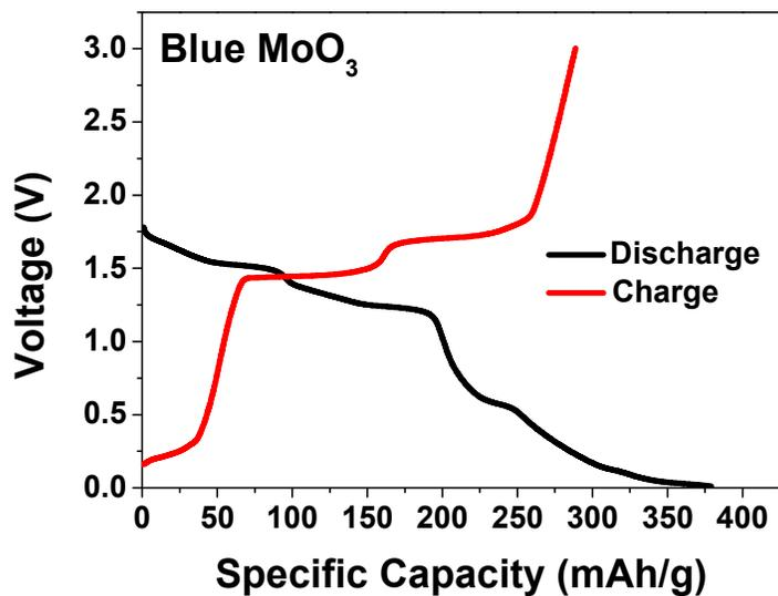
Figure S12. Discharge-charge voltage profiles of prepared blue MoO<sub>3</sub> anode in the initial cycle.
