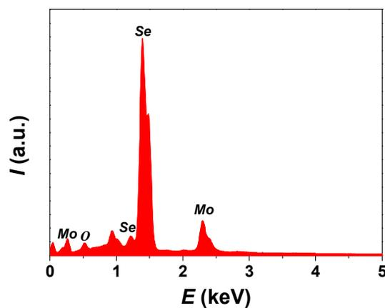
**Figure S4.** EDS spectra of the red MoSe<sub>2</sub> nanosheets, indicating the exist of elements Mo, Se, and O.
