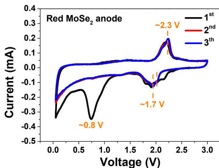
**Figure S13.** CV profiles of red MoSe<sub>2</sub> anode at a scanning rate of 0.1 mV/s showing the 1st, 2nd and 3rd cycles between 0.05 and 3.0 V.
