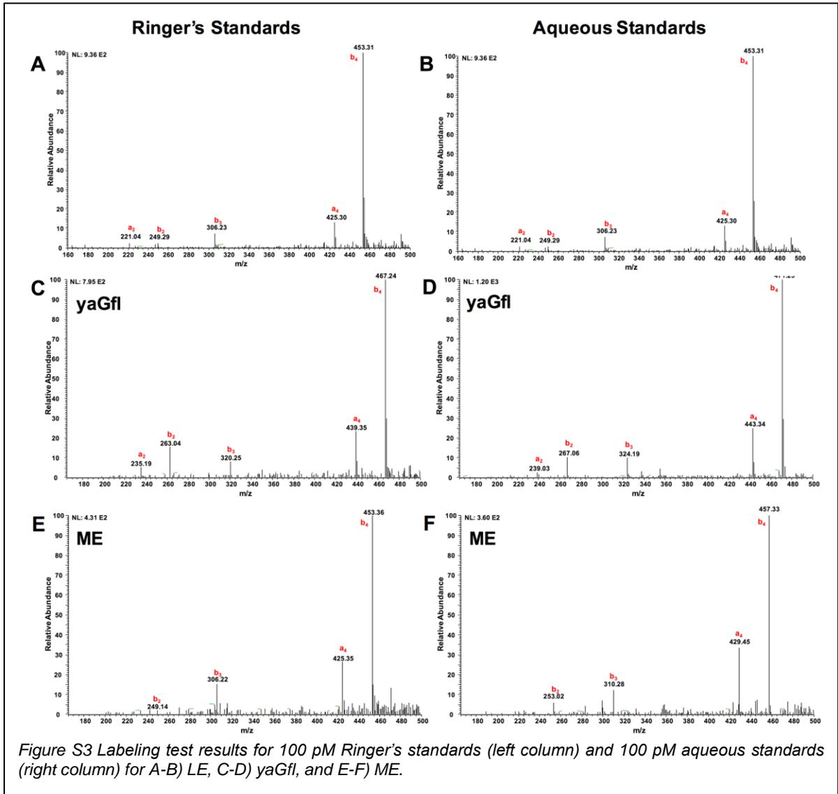
Figure S3 Labeling test results for 100 pM Ringer's standards (left column) and 100 pM aqueous standards (right column) for A-B) LE, C-D) yaGfl, and E-F) ME.
