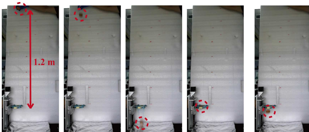
Figure S12. Series of optical images showing the egg jump from a height of 1.2m. The egg bounces and stretches the tough-hydrogel web, finally rests on the web.
