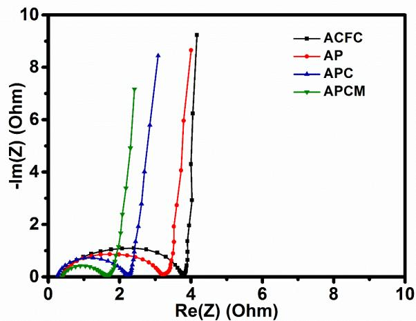
**Figure S10.** Nyquist plots of different textiles based symmetric aqueous supercapacitors. Nearly vertical lines can be observed at low frequency from all the electrodes, indicating good capacitive performance. In the high-frequency region, the Nyquist plot of APC shows the lowest equivalent series resistance, suggesting small electrode resistance and high charge-transfer rate between the electrolyte and electrodes.
