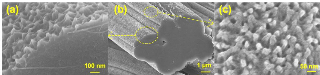
**Figure S3.** (a)-(c) Morphologies of PANI on activated carbon fiber surface in AP textile.
