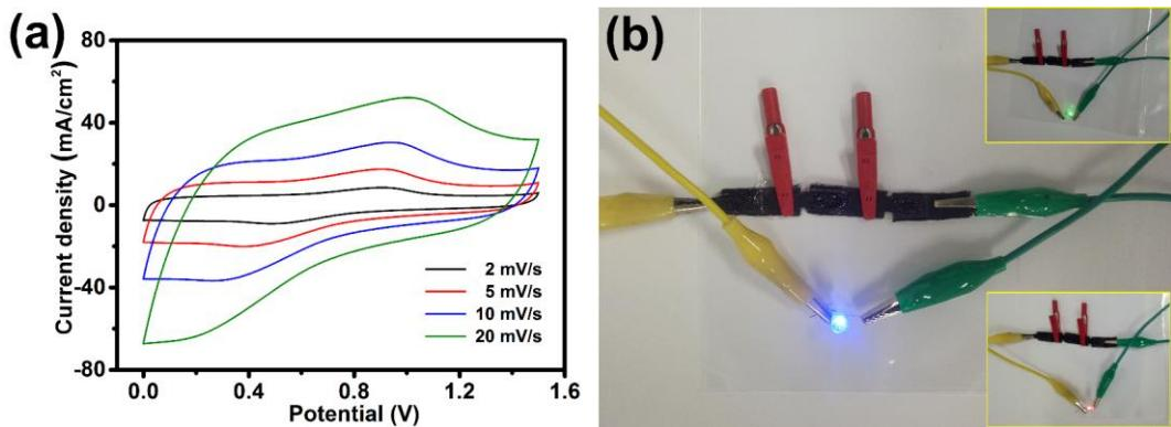
**Figure S15.** (a) CV curves of the asymmetric aqueous supercapacitor and (b) digital photographs of the flexible solid-state asymmetric textile supercapacitors (3 in series) lighting LEDs.
