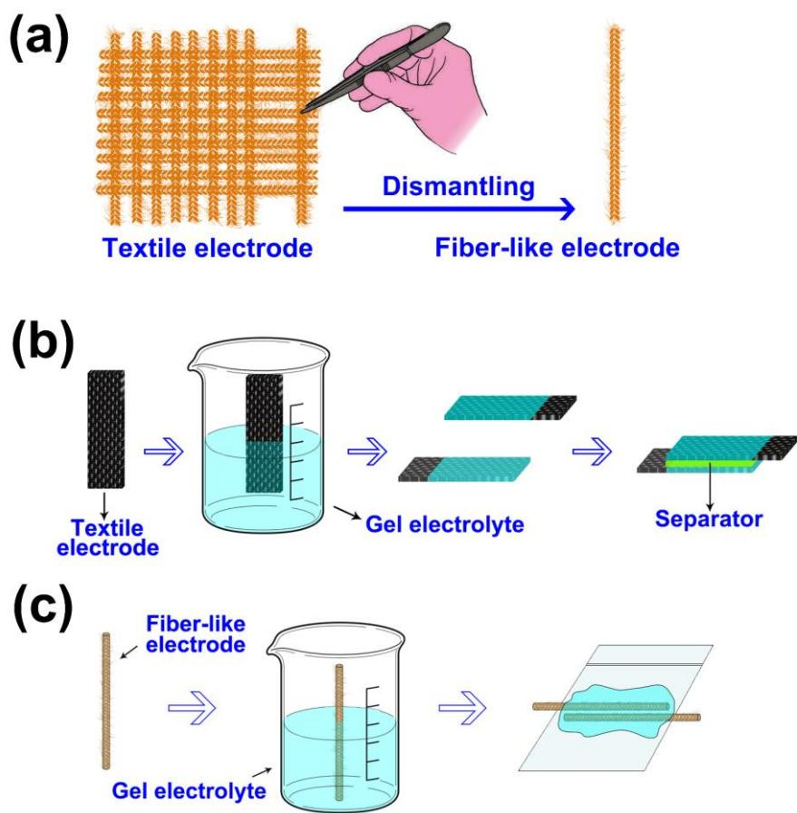
**Figure S1.** Fabrication schematics of (a) fiber-like electrode, (b) solid-state flexible textile supercapacitor and (c) solid-state flexible fiber-like supercapacitor.
