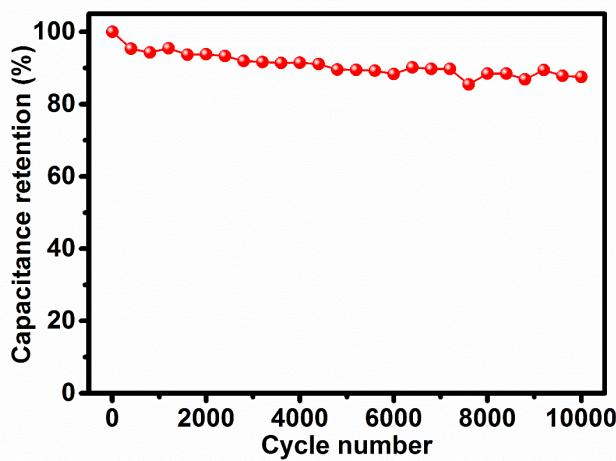
**Figure S16.** Cycling performance of the APCM fiber-like aqueous symmetric supercapacitor at the current density of  $40 \text{ mA cm}^{-2}$ .
