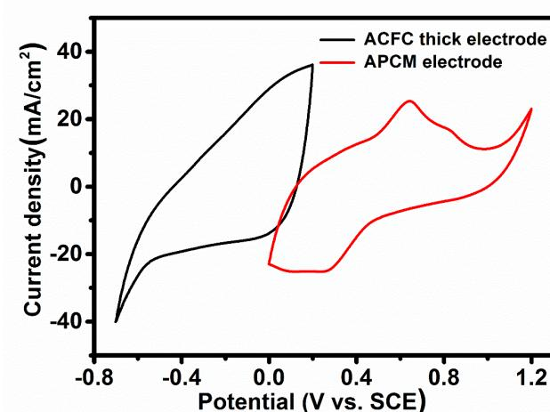
**Figure S13.** CV curves at  $2 \text{ mV s}^{-1}$  of the ACFC thick electrode and APCM electrode in  $1 \text{ M H}_2\text{SO}_4$  solution measured by three-electrode system.
