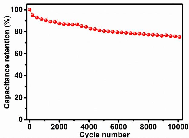
**Figure S11.** Cycling performance of APCM textile in aqueous symmetric supercapacitor at the current density of  $40 \text{ mA cm}^{-2}$ .
