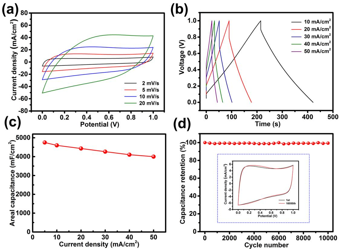
**Figure S14.** (a) CV curves, (b) GCD curves, (c) capacitance and (d) cycling behavior (applied current of  $40 \text{ mA cm}^{-2}$ ) of ACFC thick electrode in  $1 \text{ M H}_2\text{SO}_4$  solution.
