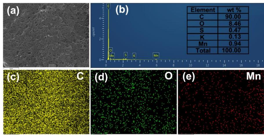
**Figure S5.** (a) SEM image and (b)-(e) EDS mapping of carbon fiber surface in APCM textile.
