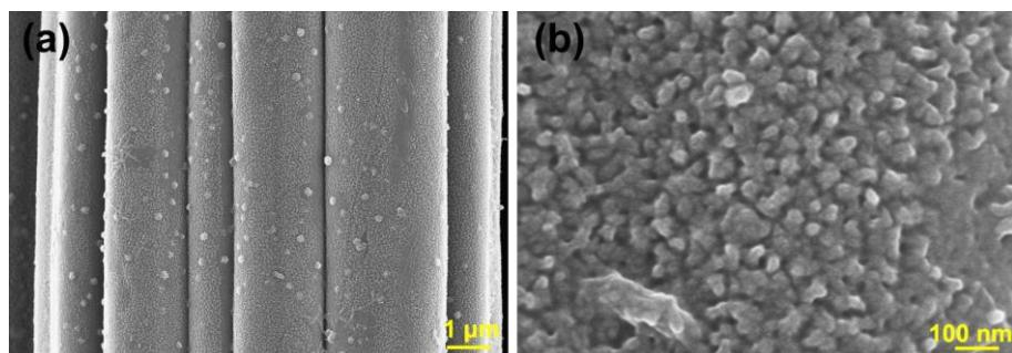
**Figure S9 (a) (b)** SEM images of AP electrode with 60 min deposition of PANI.
