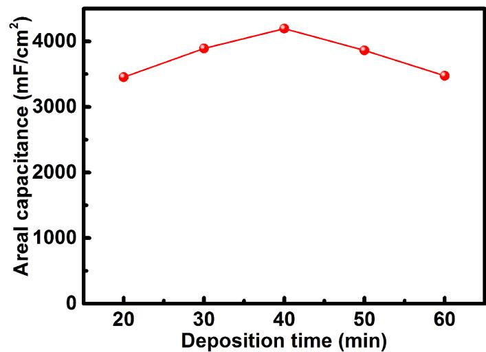
**Figure S8.** Areal capacitance of the ACFC/PANI composite textile electrodes prepared with different deposition time of PANI.
