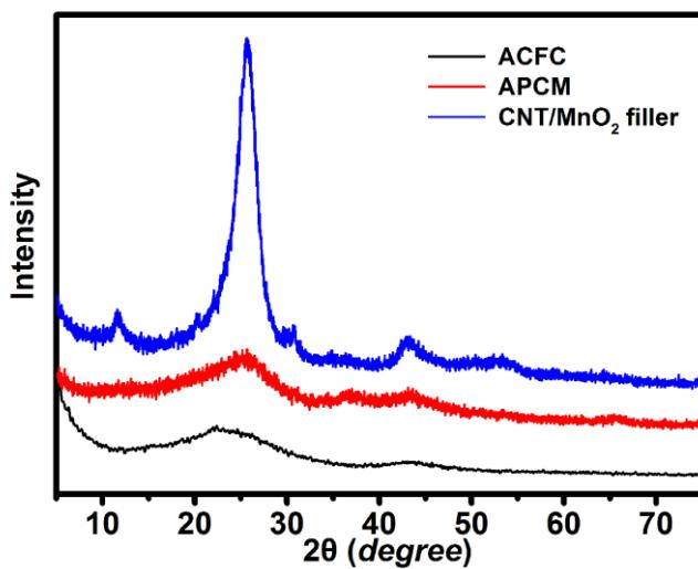
**Figure S6.** XRD patterns of ACFC, APCM and MnO<sub>2</sub>/CNT fillers. The XRD pattern indicates a type of birnessite MnO<sub>2</sub> (JCPDS#42-1317).
