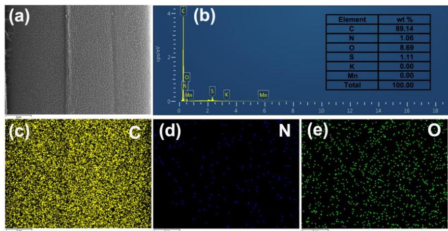
**Figure S4.** (a) SEM image and (b)-(e) EDS mapping of carbon fiber surface in AP textile.
