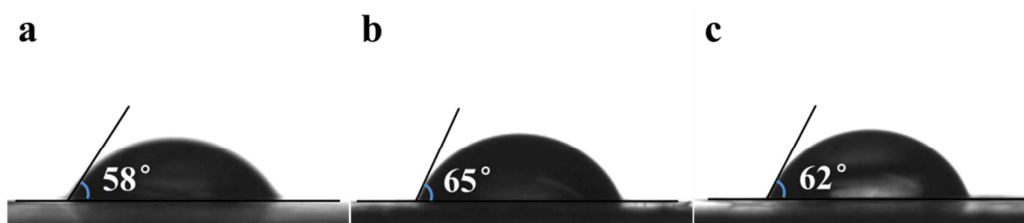
Figure S7 Digital image of a water drop on paper-like \text{Ti}_3\text{C}_2\text{T}_x (a), \text{Ti}_3\text{C}_2\text{T}_x/\text{SDS} (b) and \text{Ti}_3\text{C}_2\text{T}_x/\text{CTAB} (c). The contact angles were measured to be 58^\circ , 65^\circ and 62^\circ , respectively.
