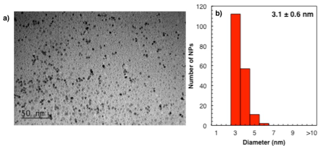
**Figure S10.** a) TEM image and b) size distribution of Pt NPs before encapsulation.
