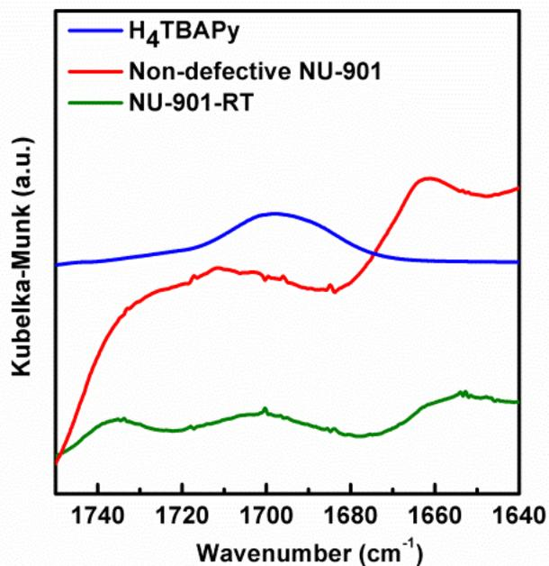
**Figure S4.** DRIFT spectra of NU-901-RT, Non-defective NU-901, and free H<sub>4</sub>TBAPy linker. The MOF spectra are multiplied by a factor of 20 for clarity.
