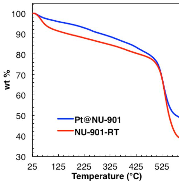
**Figure S7.** TGA traces of NU-901-RT and Pt@NU-901. The difference in wt % at 600 °C is 10 wt % similar to that determined through the ICP-OES measurements.
