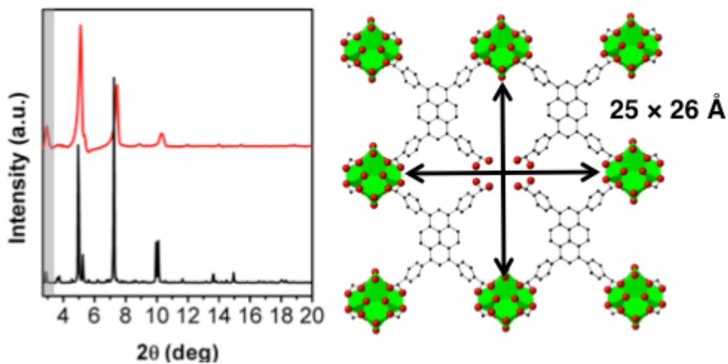
**Figure S21.** Simulated PXR D pattern of a missing  $Zr_6$  node structure, as represented by the figure on the right (viewed from the *a*-axis of the crystal). Note the similar dimension of the mesopore as to that determined through the DFT-calculated pore size distribution.
