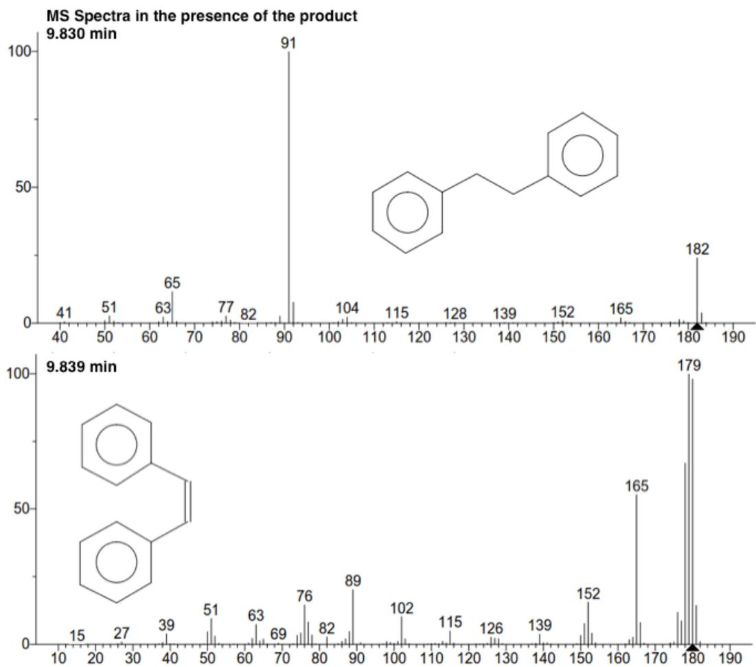
**Figure S14.** GC-MS spectra of all reaction mixtures after 1 h. The MS spectra of all controls showed no detectable amount of a molecule with  $m/z = 182$ , suggesting an absence of bibenzyl.
