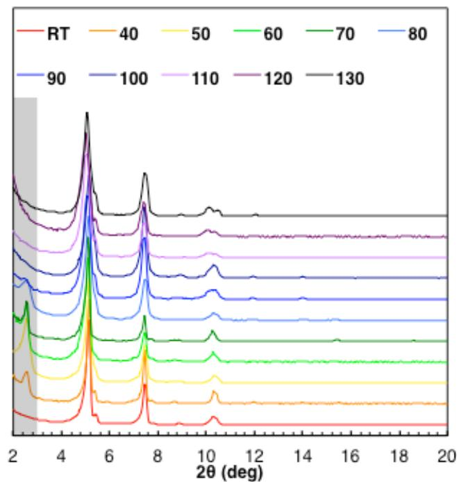
**Figure S5.** PXRD patterns of NU-901 synthesized at various temperatures. The  $2\theta = 2.5^\circ$  peak is highlighted in gray.
