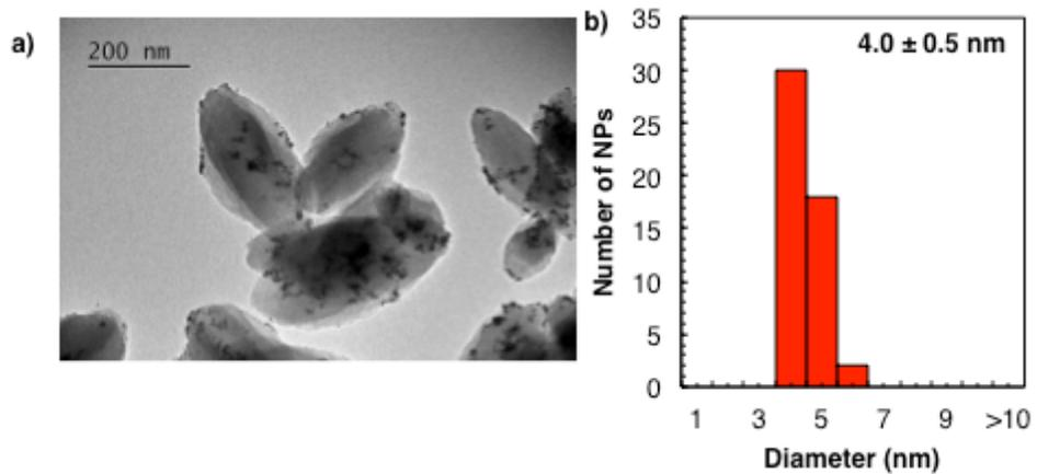
**Figure S9.** a) TEM image of Pt@NU-901 and b) histogram for the particle size distribution of encapsulated Pt NPs.
