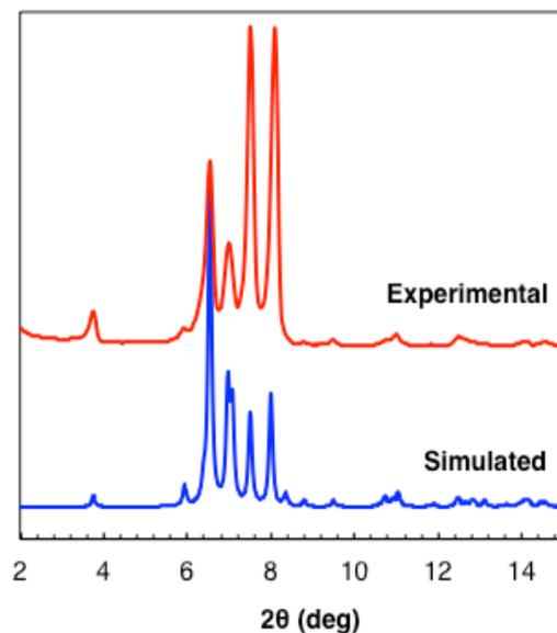
**Figure S1.** Experimental and simulated PXRD patterns of the  $Zr_6$  node.
