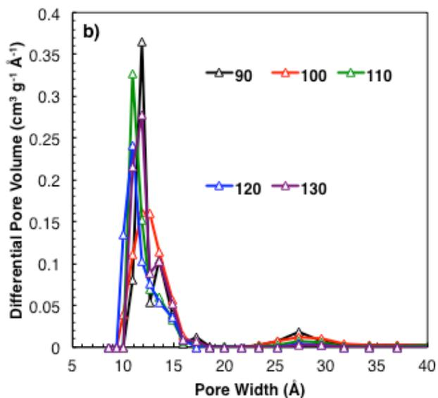
**Figure S6.** DFT-calculated pore size distribution of NU-901 synthesized at various temperatures.
