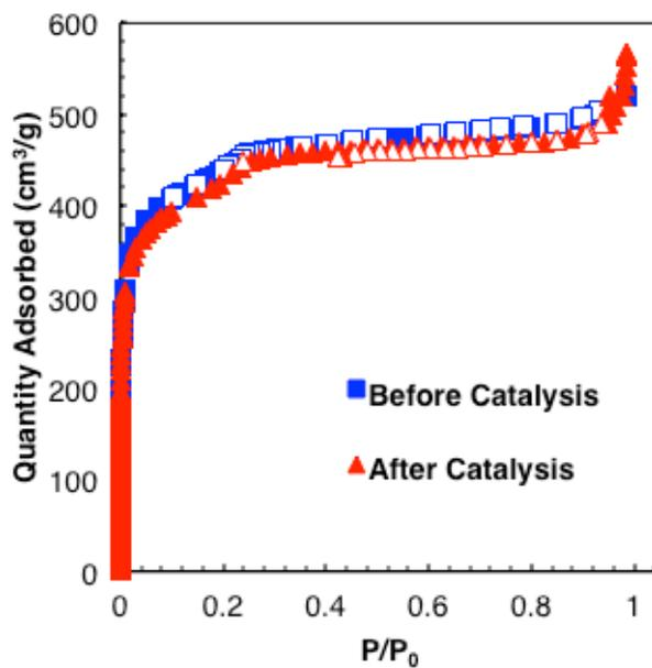
**Figure S16.** N<sub>2</sub> isotherm at 77 K of Pt@NU-901 before and after catalysis.
