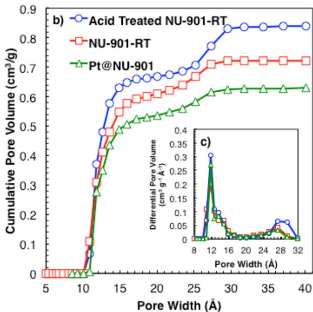
**Figure S3.** a) N<sub>2</sub> isotherms and DFT-calculated b) cumulative and c) differential pore size distributions of NU-901-RT before and after acid treatment and Pt@NU-901.
