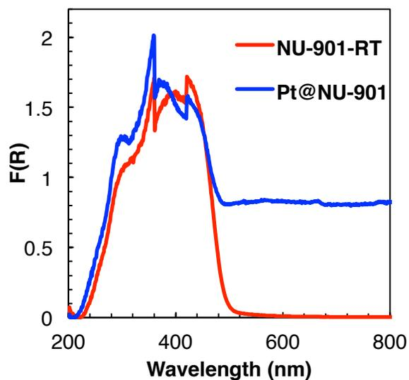
**Figure S11.** Diffuse reflectance UV-Vis Spectra of NU-901-RT and Pt@NU-901. Enhanced extinction in 500–800 nm region is attributed to the scattering due to close packing of Pt NPs and the MOF.
