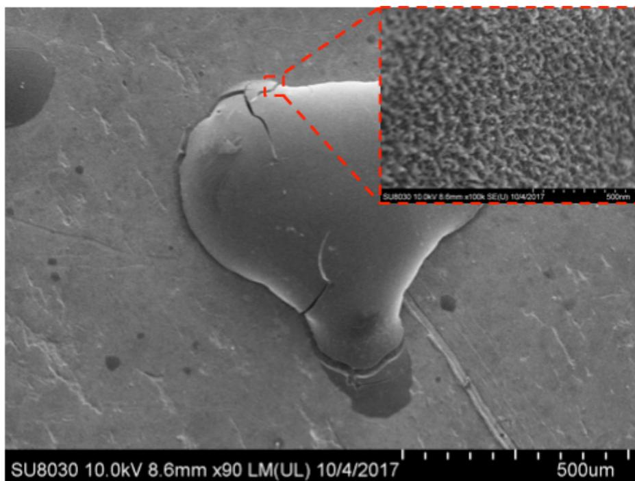
**Figure S18.** SEM images of bare Pt NPs after 1 h of catalysis.
