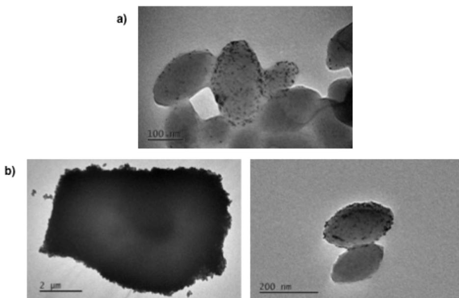
**Figure S20.** TEM images of **Pt/NU-901** (i.e. Pt NPs on the exterior surface of NU-901) **a)** before and **b)** after catalysis.
