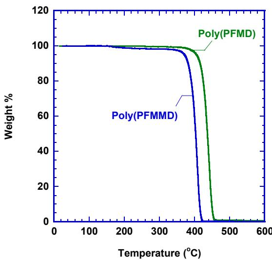
**Figure S1.** TGA curves of poly(PFMD) and poly(PFMMD) under N<sub>2</sub> atmosphere.
