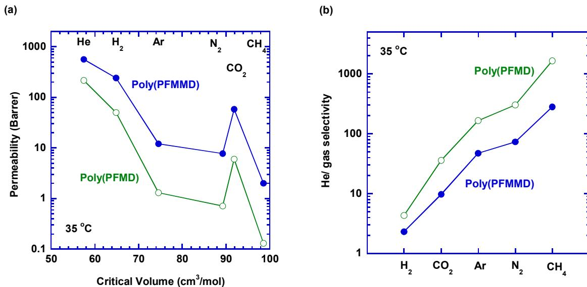
**Figure S2.** Comparison of (a) gas permeability and (b) He/gas selectivity at 35 °C in poly(PFMD) and poly(PFMMD).
