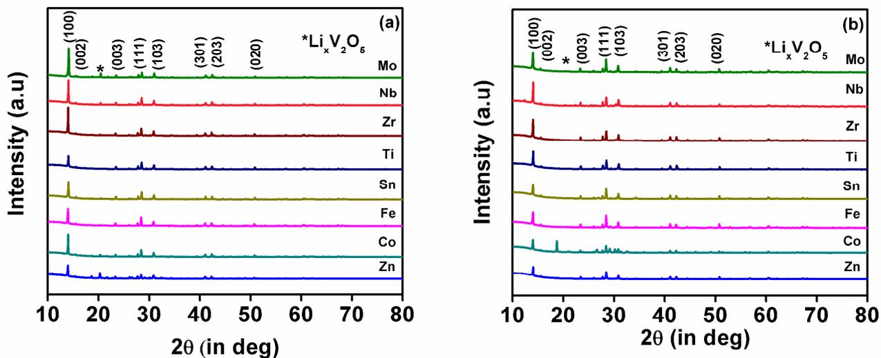
**Figure.S1** (a) XRD pattern of  $\text{LiV}_{2.99}\text{M}_{0.01}\text{O}_8$  and (b)  $\text{LiV}_{2.9}\text{M}_{0.1}\text{O}_8$  ( $\text{M} = \text{Zn}/\text{Co}/\text{Fe}/\text{Sn}/\text{Ti}/\text{Zr}/\text{Nb}/\text{Mo}$ ) compounds
