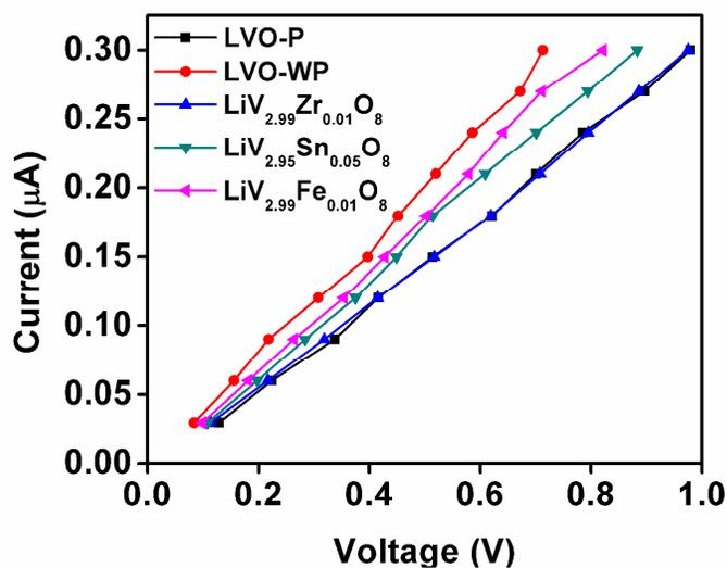
**Figure.S3** V/I spectra of LVO-P, LVO-WP,  $\text{LiV}_{2.99}\text{Zr}_{0.01}\text{O}_8$ ,  $\text{LiV}_{2.95}\text{Sn}_{0.05}\text{O}_8$  and  $\text{LiV}_{2.99}\text{Fe}_{0.01}\text{O}_8$  compounds
