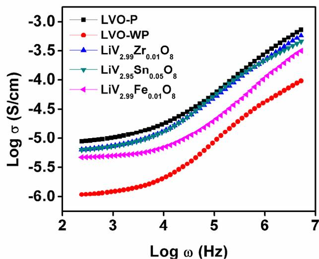
**Figure.S2** Conductivity spectra of LVO-P, LVO-WP,  $\text{LiV}_{2.99}\text{Zr}_{0.01}\text{O}_8$ ,  $\text{LiV}_{2.95}\text{Sn}_{0.05}\text{O}_8$  and  $\text{LiV}_{2.99}\text{Fe}_{0.01}\text{O}_8$  compounds
